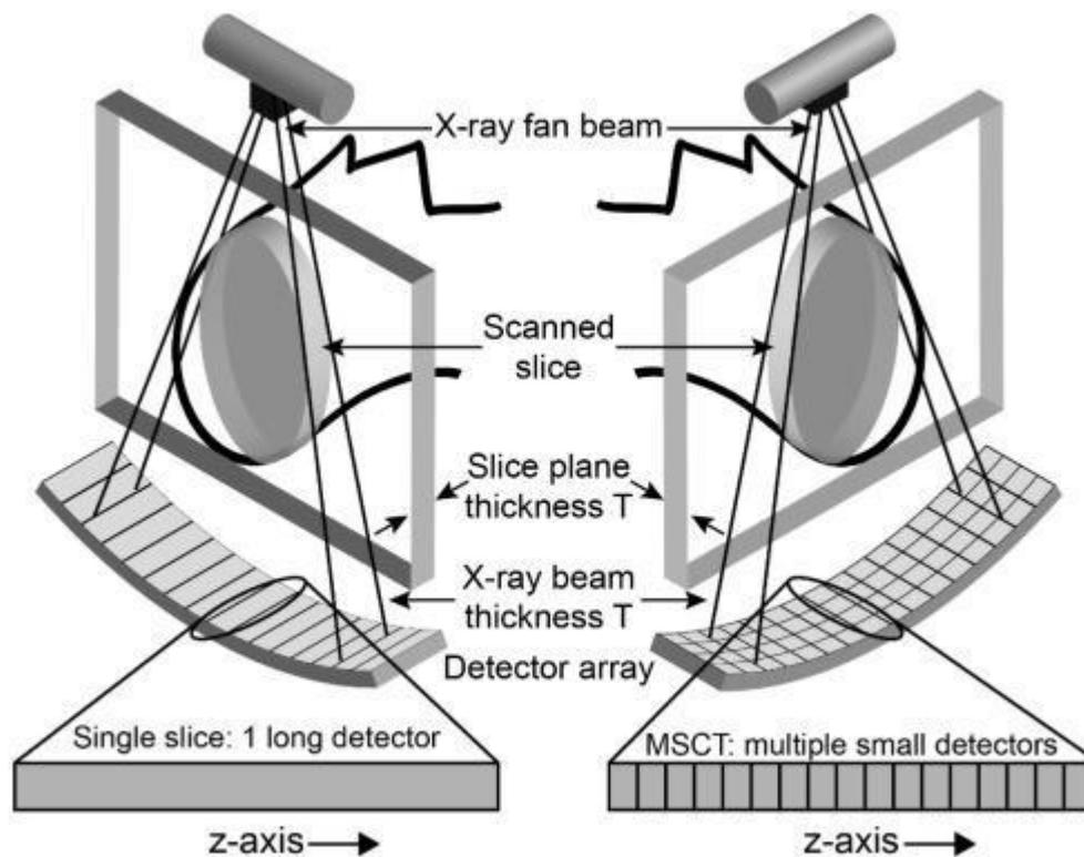
Figure (2.1): Shows multi detector CT scanner.<sup>(9)</sup>
