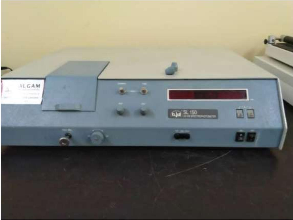
**Plate No.4:** Spectrophotometer (measure chemical compounds in a sample).
