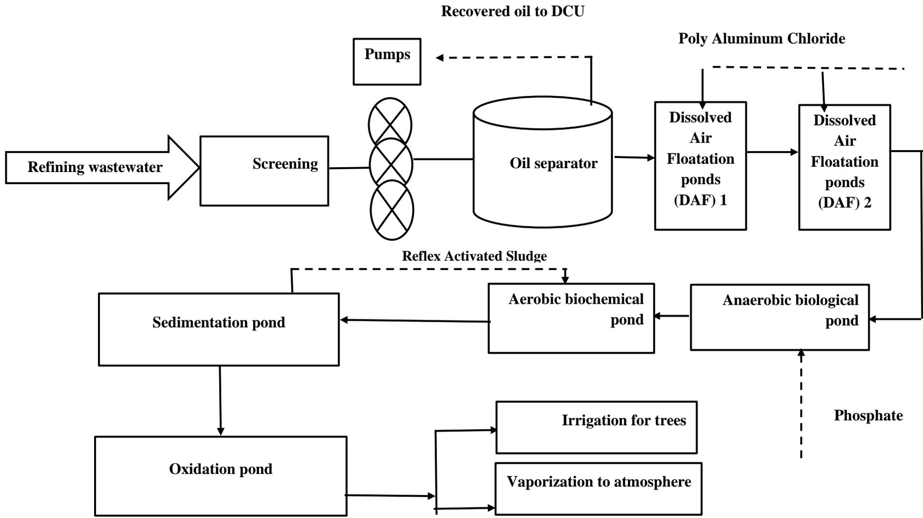
Fig (2.3): waste water treatment process flow chart (Operation Manual for Water Purifying Treatment Unit, 2004)
