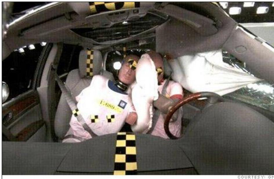
Figure 2-4. The center airbags (Nayak et al., 2013)
