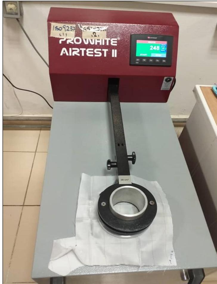
Figure 4-6: Air permeability tester.
