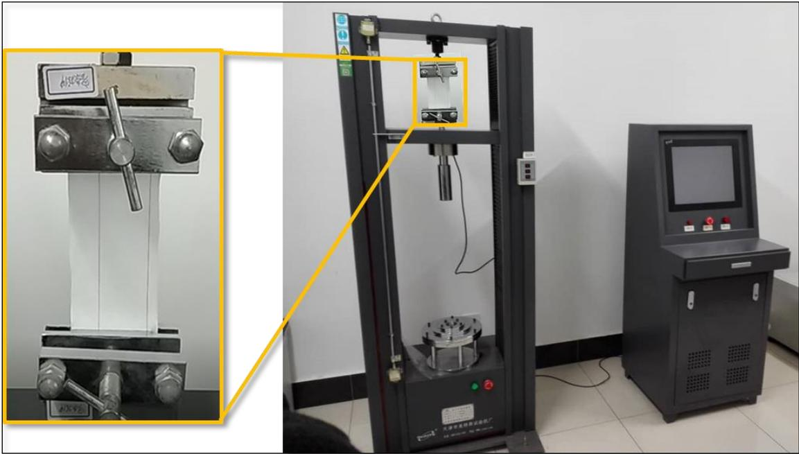
Figure 4-4: Tensile strength tester.
