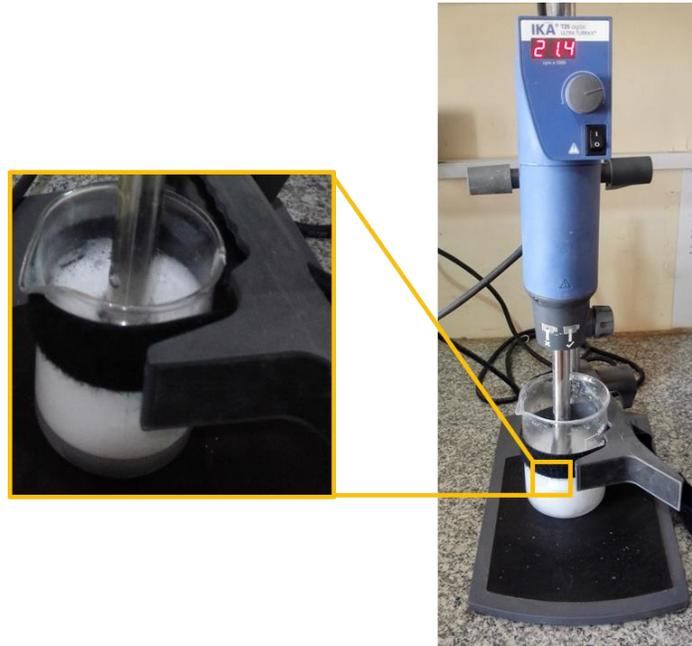
Figure 3-6: Sonication of silica nanoparticles in PVA solution.
