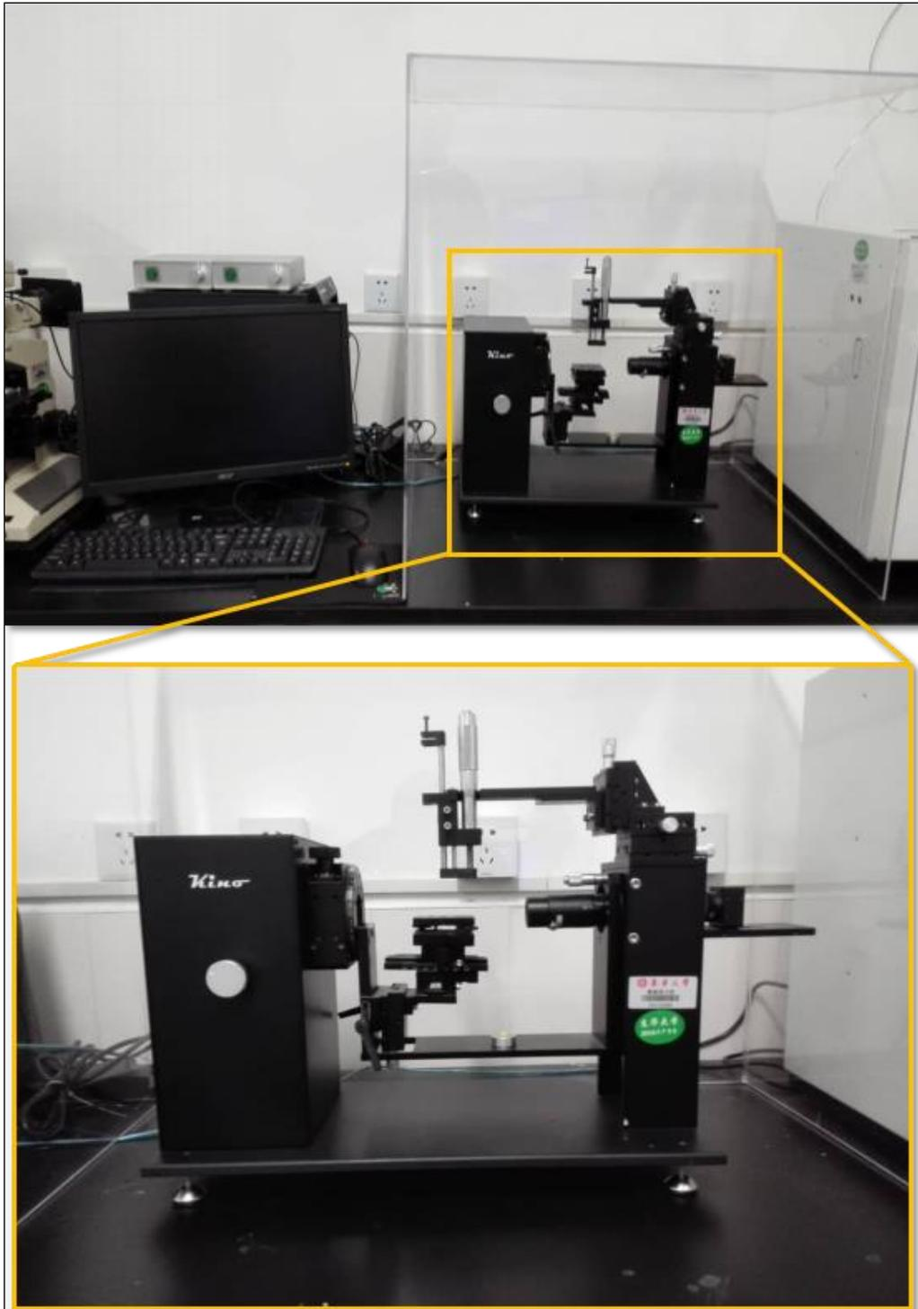
Figure 4-5: Water Contact angle (WCA) tester.
