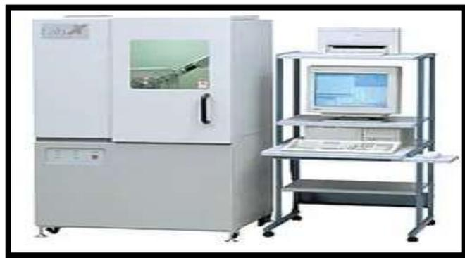
Figure (3.1) XRD instrument
