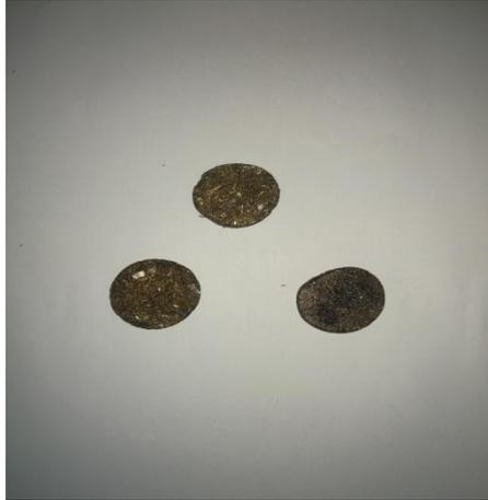
Figure (4-3-3): Copper + Gum-Arabic After compressing in the piston
