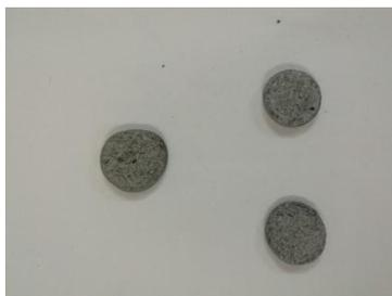
Figure (4-3-1): Aluminum + Gum-Arabic After compressing in the piston
