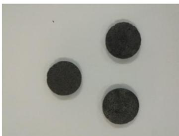
Figure (4-3-2): Iron + Gum-Arabic After compressing in the piston
