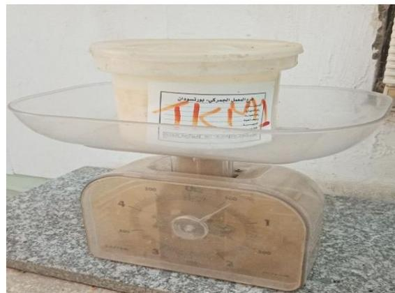
**Figure 3.6: A prepared soil sample filling in a Marinelli beaker sealed with plastic tape to prevent the escape of airborne radionuclide**
