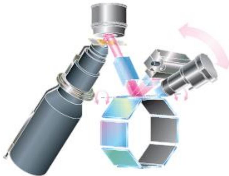
Figure (3.8) Construction of wavelength dispersive spectrometer with 2D optics and direct excitation
