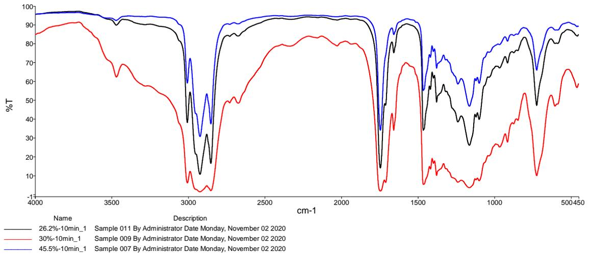
Figure (4-23) FTIR spectrum of samples compare with different humidity in 10 min.
