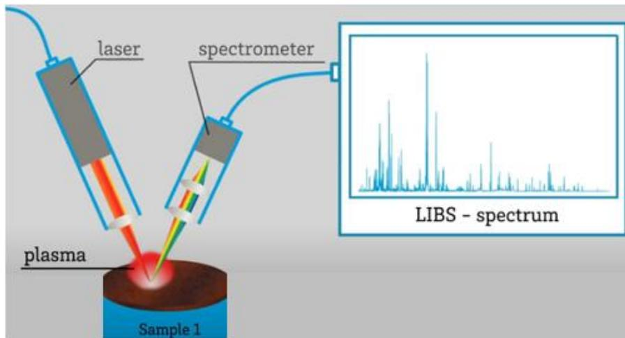
Figure (1-3): schematic diagram of simple libs system
