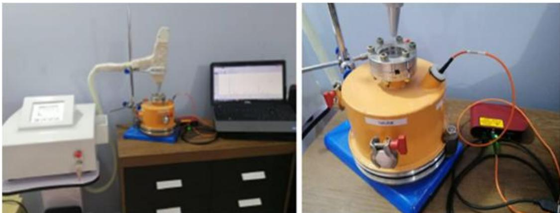
Figure (3-3) Optical System for Libs.
