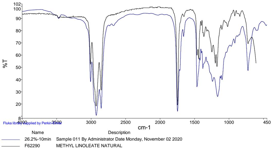
Figure (4-3) FTIR spectrum of sample (S1) at 26.2% -10 min compare with Fluka library.
