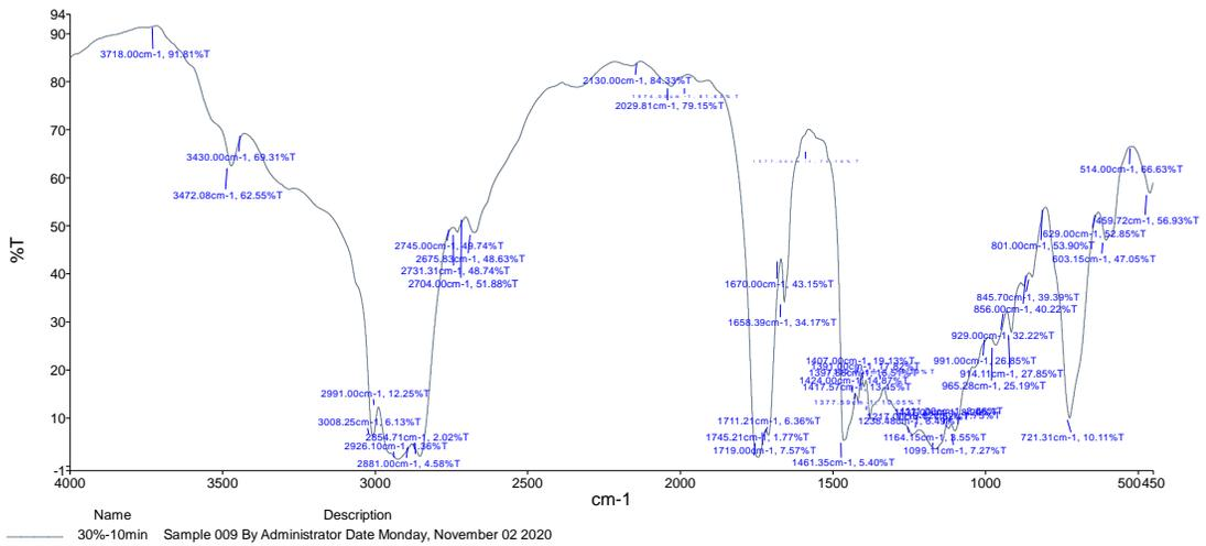
Figure (4-11) FTIR spectrum of sample (S2) at 30% -10 min compare with peaks by Fluka library.
