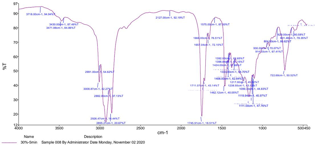
Figure (4-9) FTIR spectrum of sample (S2) at 30% -5 min compare with peaks by Fluka library.
