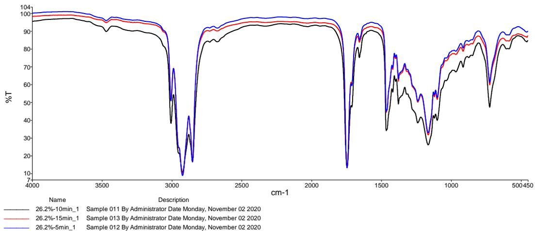
Figure (4-7) FTIR spectrum of sampled (S1) compare in different time.
