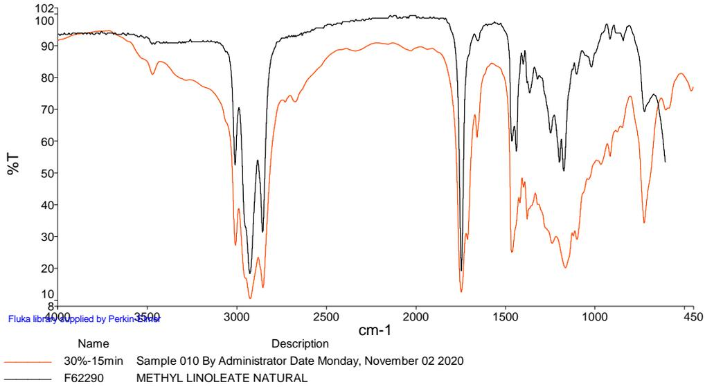
Figure (4-12) FTIR spectrum of sample (S2) at 30% -15 min compare with Fluka library.
