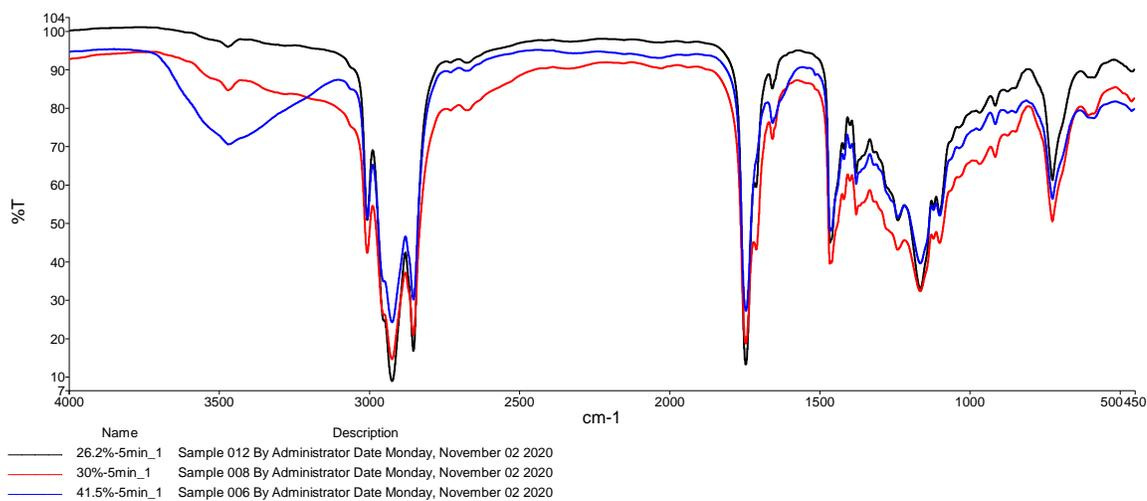
Figure (4-22) FTIR spectrum of samples compare with different humidity in 5 min.
