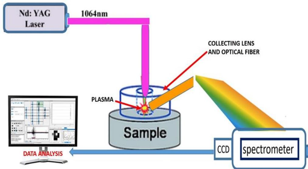
Figure 3.4 Experimental Setup of LIBS.
