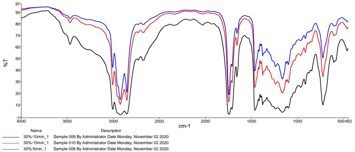
Figure (4-14) FTIR spectrum of sampled (S2) compare in different time.
