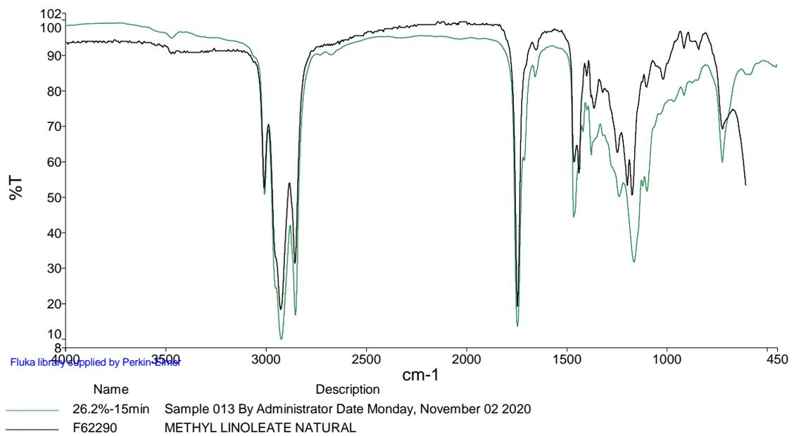
Figure (4-5) FTIR spectrum of sample (S1) at 26.2% -15 min compare with Fluka library.
