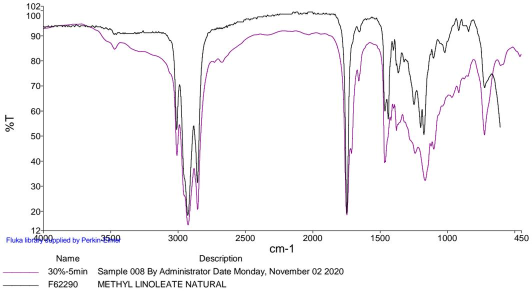
Figure (4-8) FTIR spectrum of sample (S2) at 30% -5min compare with Fluka library.
