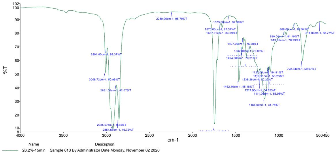
Figure (4-6) FTIR spectrum of sample (S1) at 26.2% -15 min with peaks by Fluka library.
