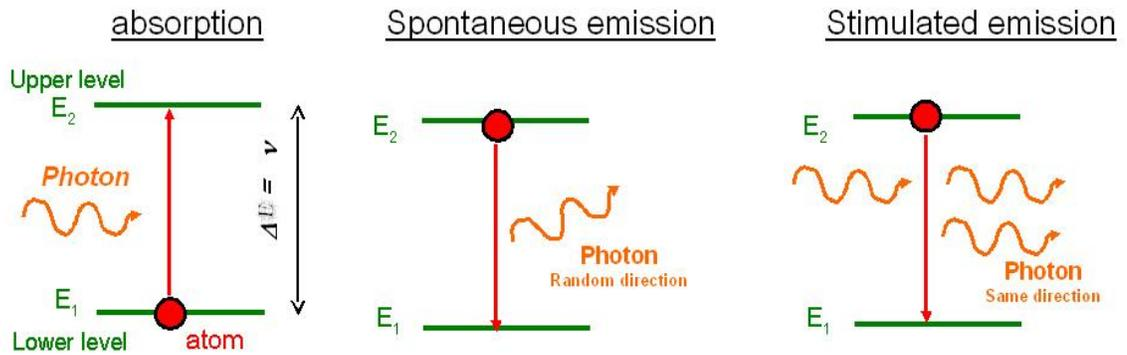
Figure (1.1) Mechanism of the interaction between an atom and a photon
