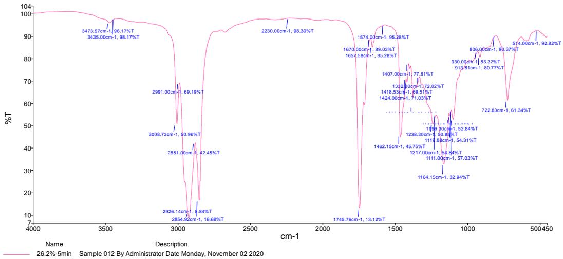
Figure (4-2) FTIR spectrum of sample (S1) at 26.2% -5min with peaks by Fluka library.
