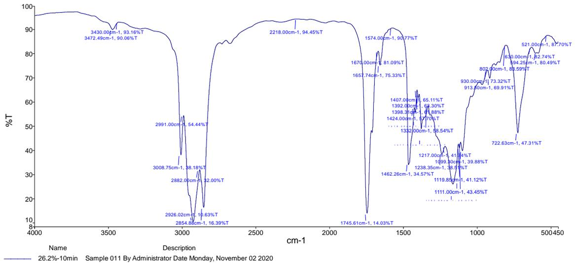
Figure (4-4) FTIR spectrum of sample (S1) at 26.2% -10 min with peaks by Fluka library.
