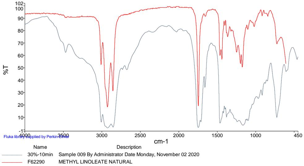
Figure (4-10) FTIR spectrum of sample (S2) at 30% -10 min compare with Fluka library.
