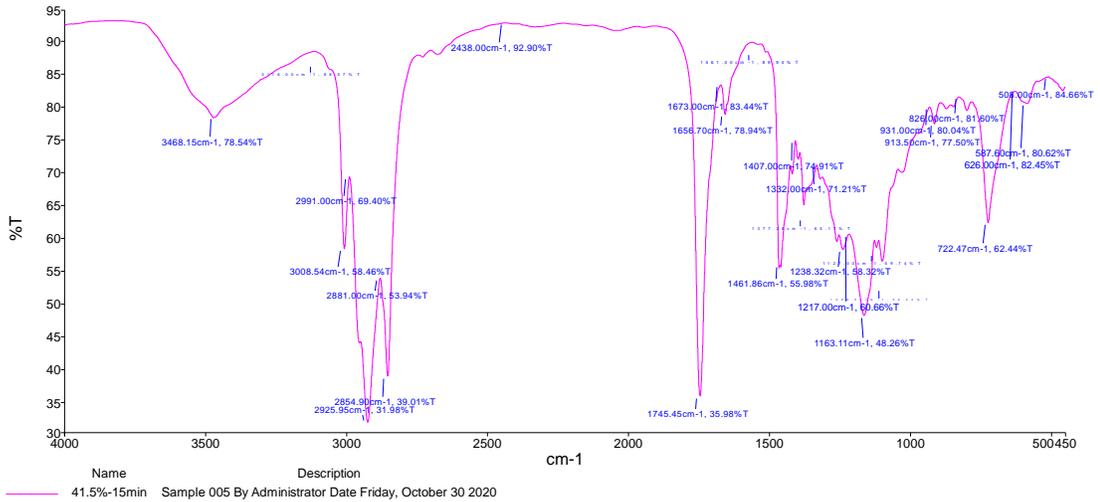
Figure (4-20) FTIR spectrum of sample (S3) at 41.5% -15 min with peaks by Fluka library.
