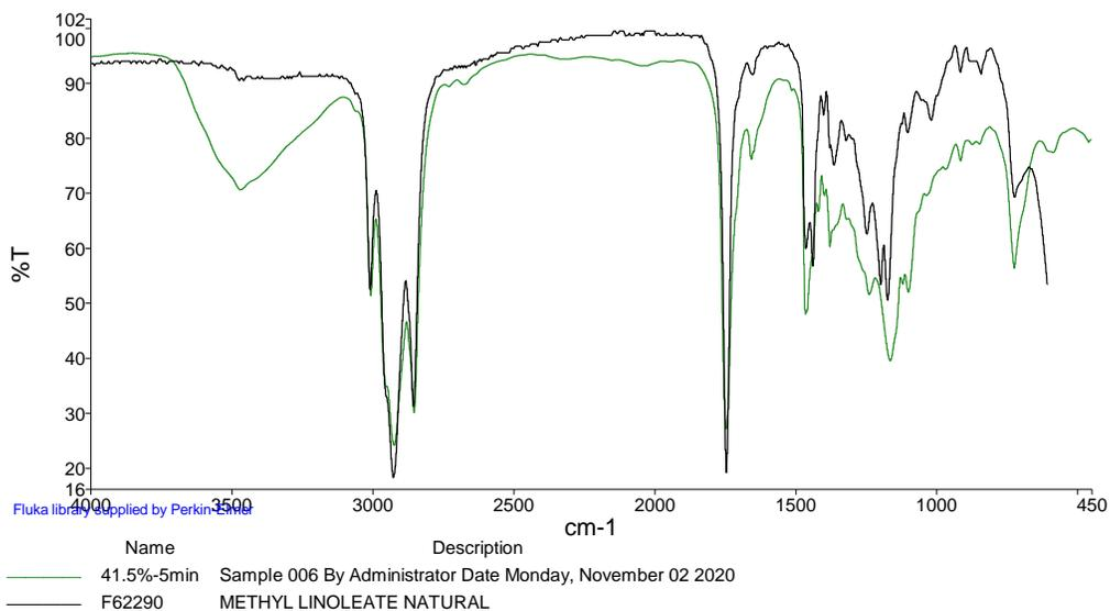
Figure (4-15) FTIR spectrum of sample (S3) at 41.5% -5min compare with Fluka library.
