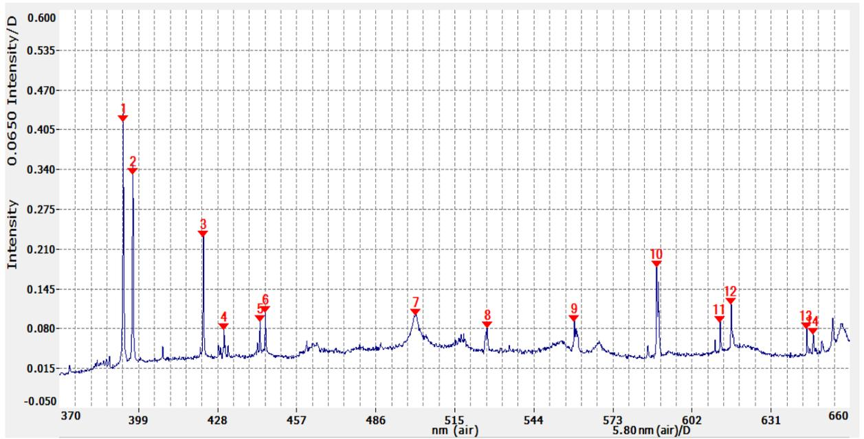
Figure (4-25) LIBS spectrum of sample (S1) at 26.2% -5min.
