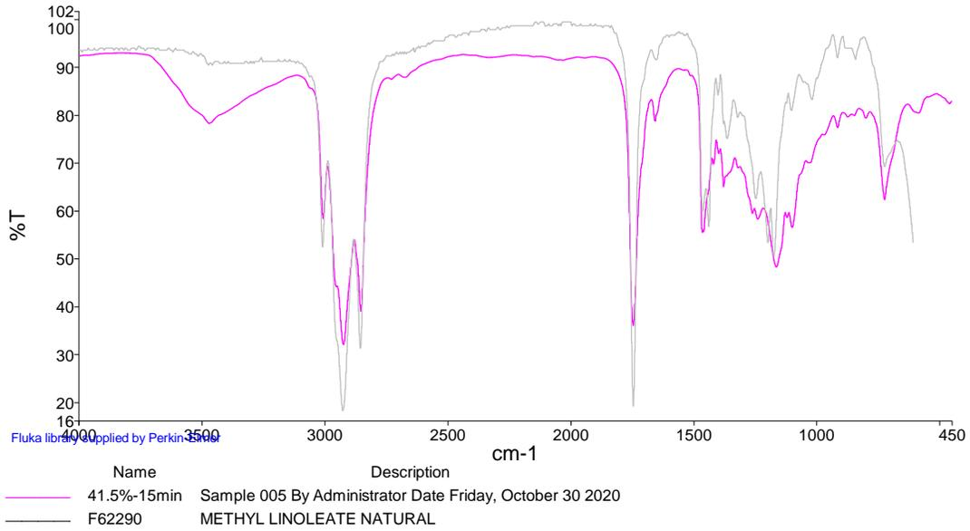
Figure (4-19) FTIR spectrum of sample (S3) at 41.5% -15 min compare with Fluka library.
