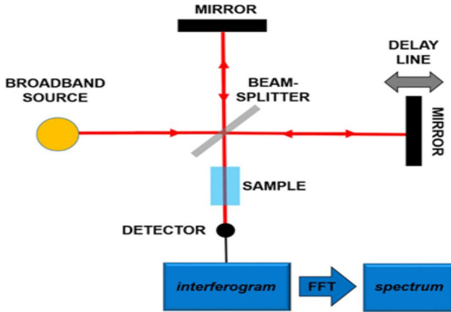
Figure (1-2): Fourier Transform Infrared spectroscopy (FTIR) principle
