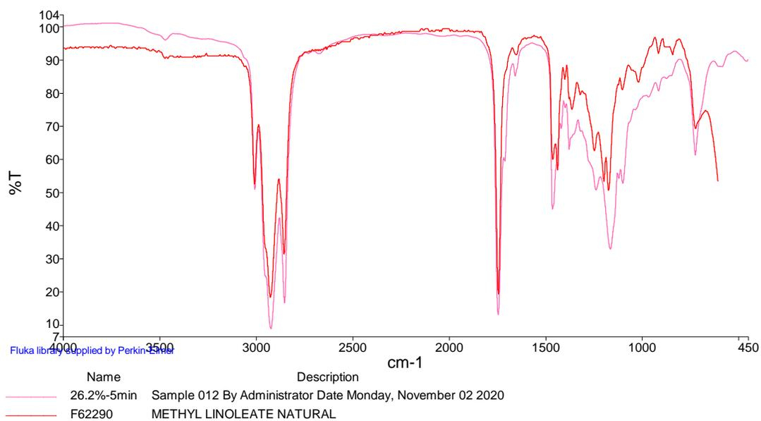
Figure (4-1) FTIR spectrum of sample (S1) at 26.2% -5min compare with Fluka library.
