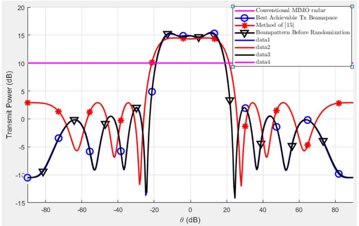
Figure 4.3: Transmit beampatterns of the traditional MIMO
