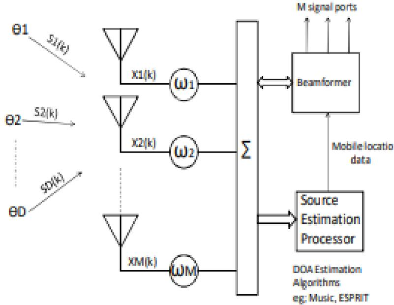
Figure 2.2: M element antenna array with D arriving signals
