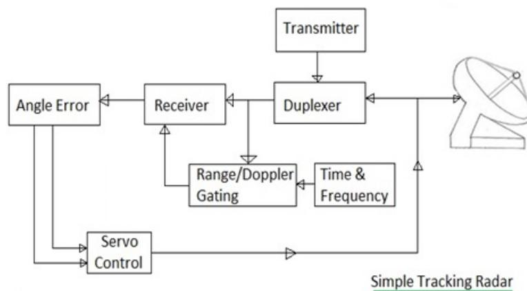
Figure 1.1: Radar Operation [2]
