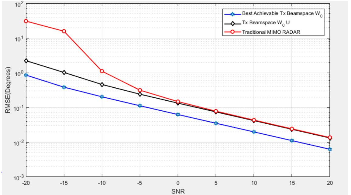
Figure 4.2: The root mean square error RMSE Versus SNR
