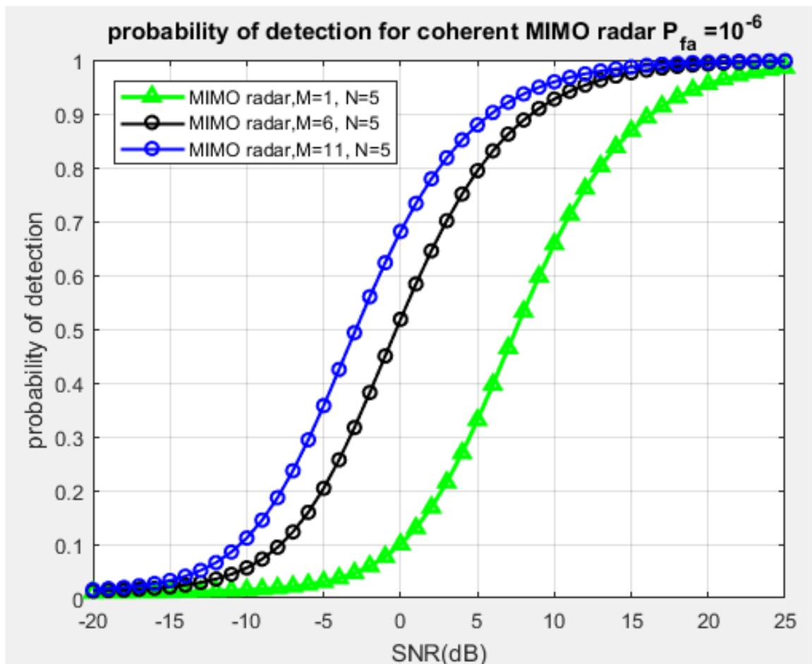
Figure 4.1: Coherent MIMO Radar: The performance of Changing N
