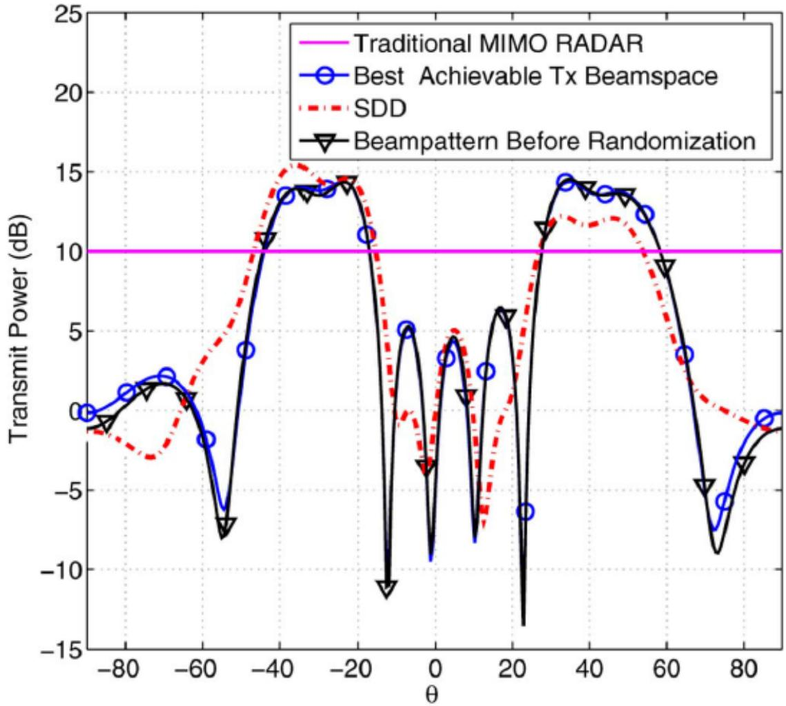
Figure 4.4: Transmit beampatterns of the traditional MIMO, Two Separated Sectors of Width 20 Degrees Each.
