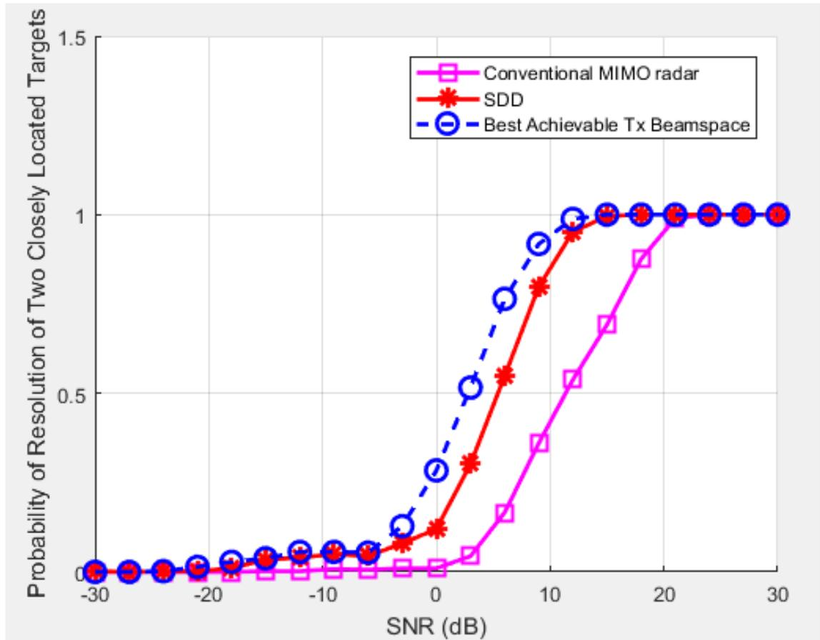
Figure 4.5: The probability of resolve two closely located targets versus SNR
