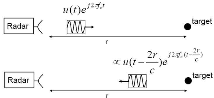
Figure 1.2: Detection and ranging
