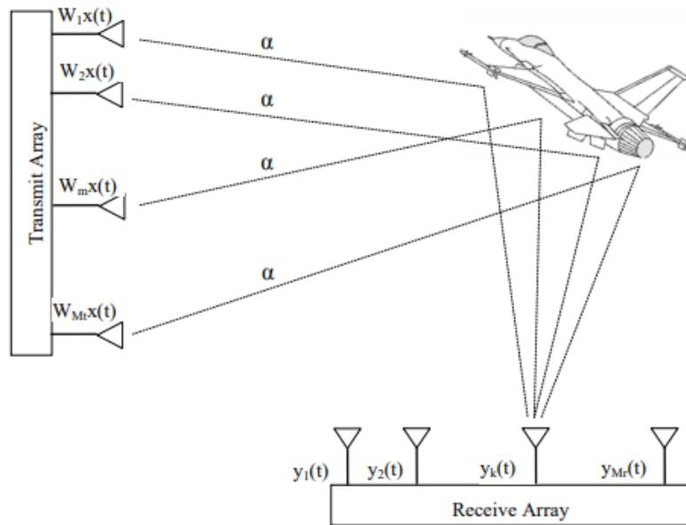
Figure 3.1: Phased Array Radar Configuration [20]
