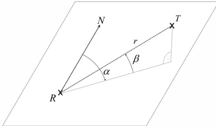
Figure 2.4: Parameters of the Target Position [14]
