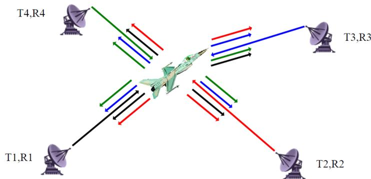
Figure 2.3: MIMO radar
