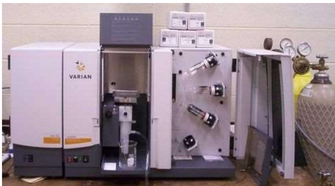
Figure 2.3 Varian atomic absorption spectrometer (AAS) instrument
