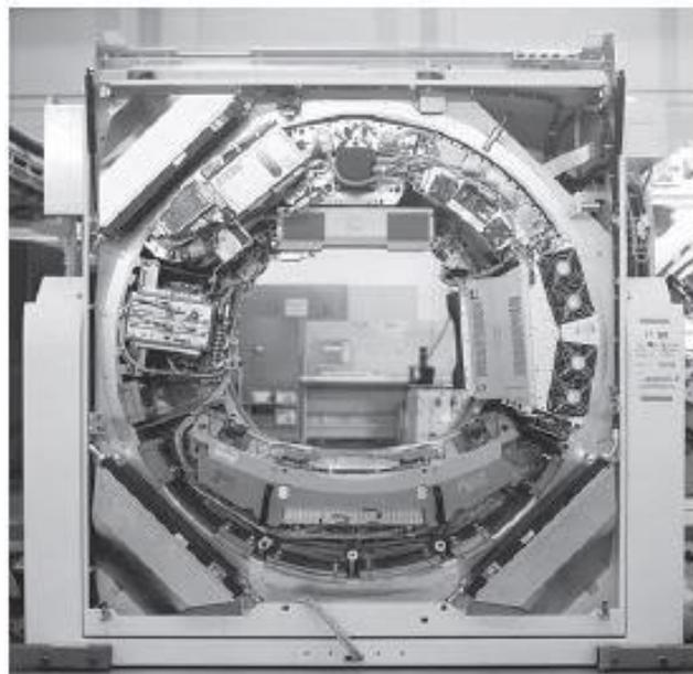
**Figure (2.2) The gantry houses many of the components necessary to produce and detect x-rays. The gantry cover is removed on this third-**
