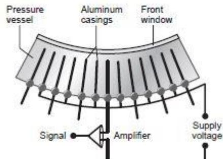
**Figure (2.4) Structure of a xenon gas detector array.**
