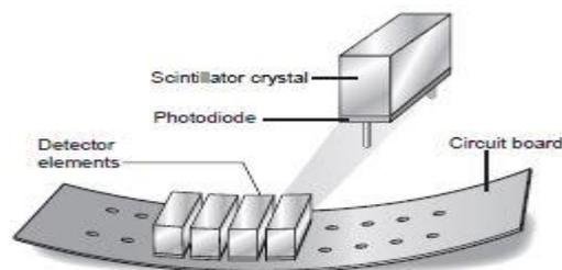
**Figure (2.5) Structure of a solid-state detector array.**
