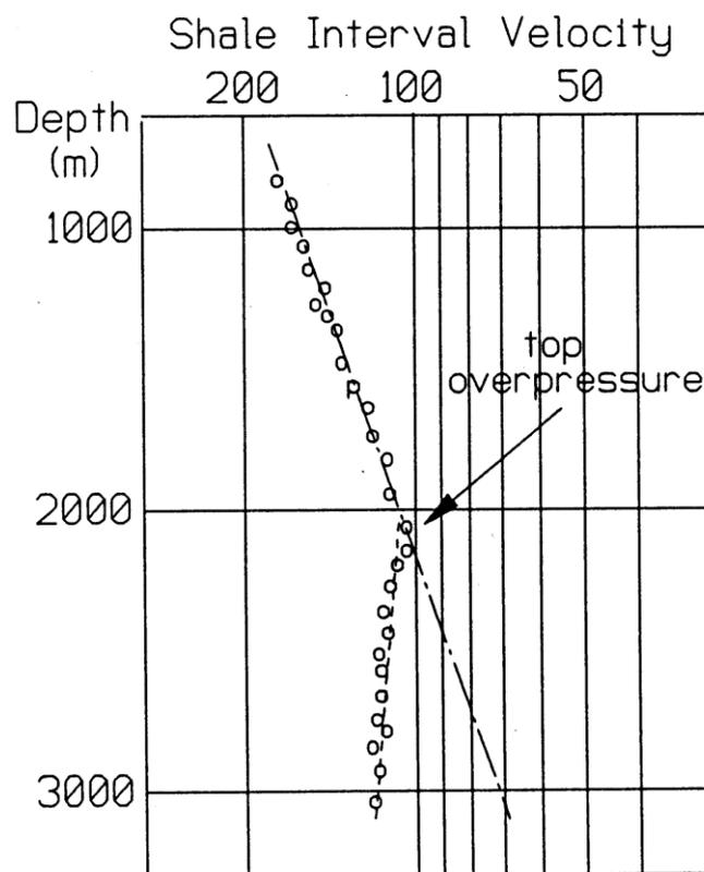
Figure 2.1 the interval velocity
