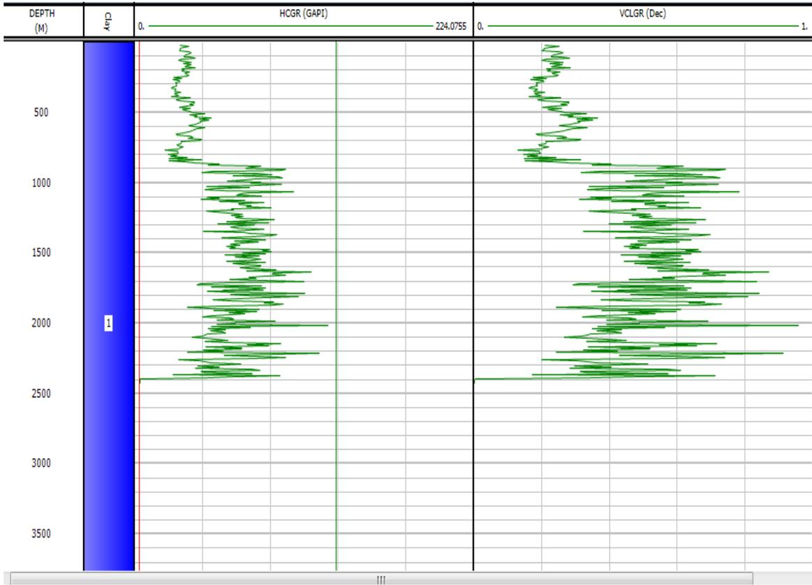
Figure 3.2 volume of shale from gamma ray log
