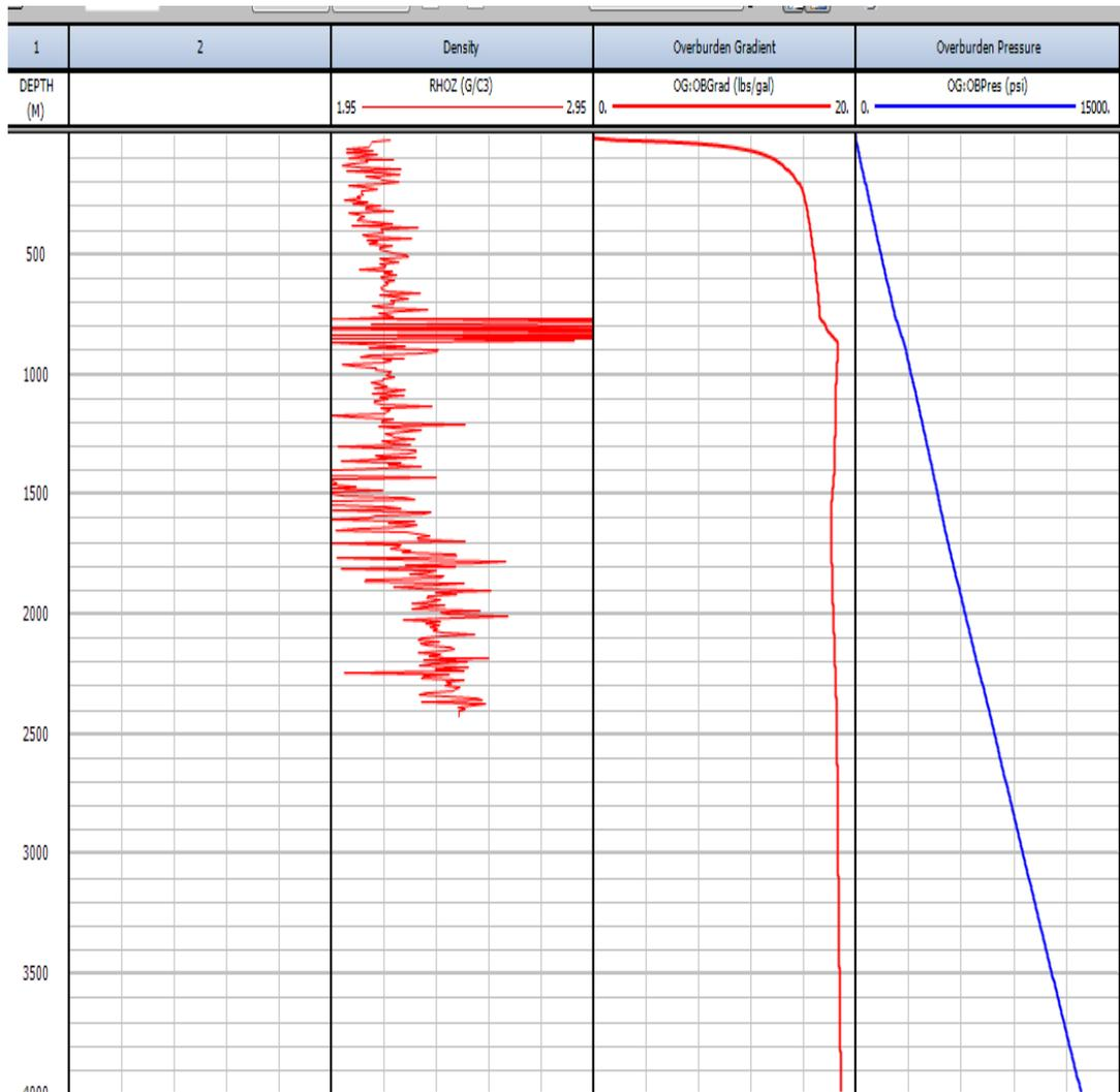
Figure 3.4 output data of over burden Gradient curve& Over burden pressure curve and bulk density
