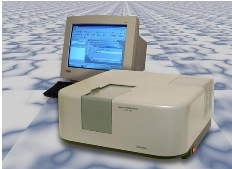
**Figure (2.4): Spectrophotometer (Labomed – UVS-2800)**
