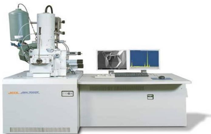
**Figure (2.1): Scanning Electron Microscopy (SEM) Energy Disperse X-ray EDX (JEOL 7000f)**
