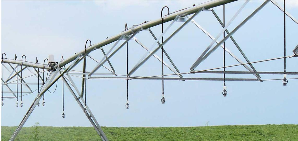
Figure (2.1): The pipeline, the supporting structure and the sprinkler. [5]
