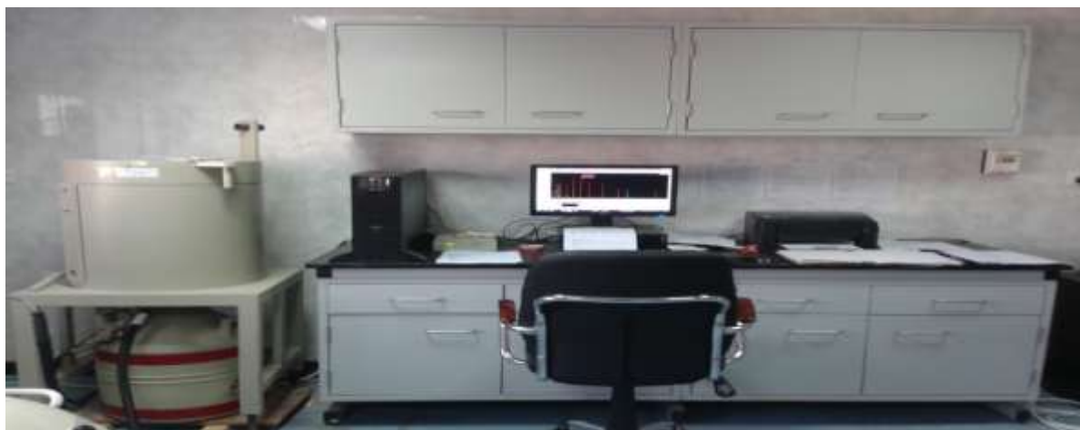
Fig(3-4): gamma ray spectroscopy system with high purity Germanium detector (HPGe).
