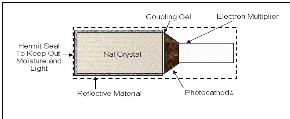
**Figure 2.2 the diagram below shows the parts of a standard commercial NaI detector.** ([http\physics.tamuk.edu](http://physics.tamuk.edu))
