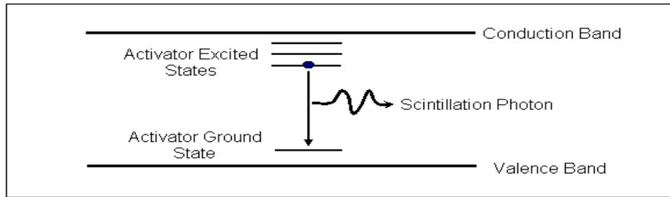
**Figure 2.1 shows (inorganic scintillator crystal is doped with a small amount of an activator impurity (in the case of NaI this is thallium)).**
