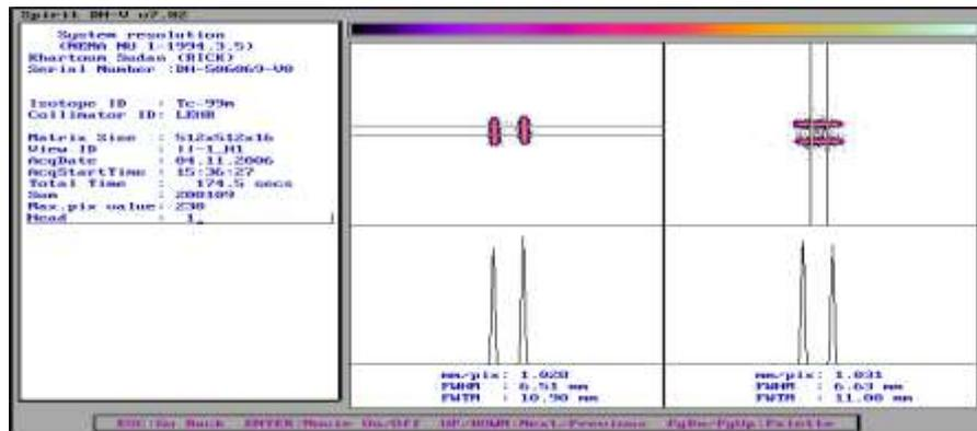
**Figure 2. 12: demonstrate system resolution**
