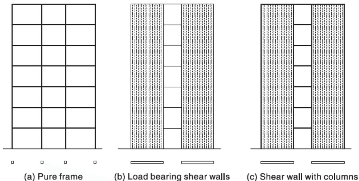
Fig. 2.8 Types of system framing (Earthquake Behavior of Buildings, 2012)
