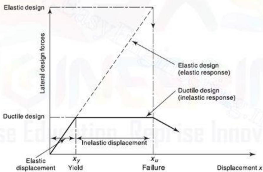
Fig.3.7 Lateral forces and ductility (ductility factor  $x_u/x_y$ , ductile capacity  $x_u/x_y$ ) (Chen and Lui, 2006)
