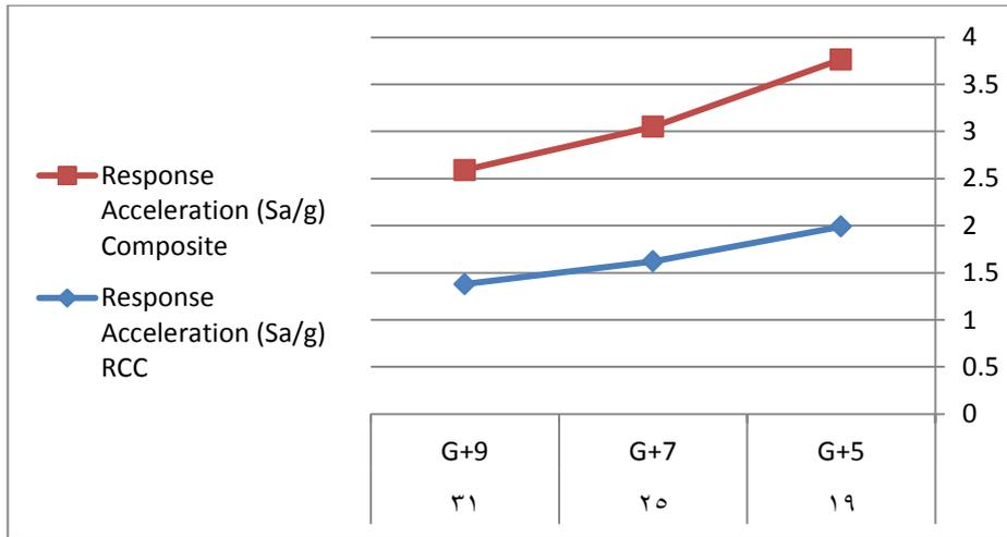
Figure 4.5: Graph of Average Response Acceleration against Number of stories for both models
