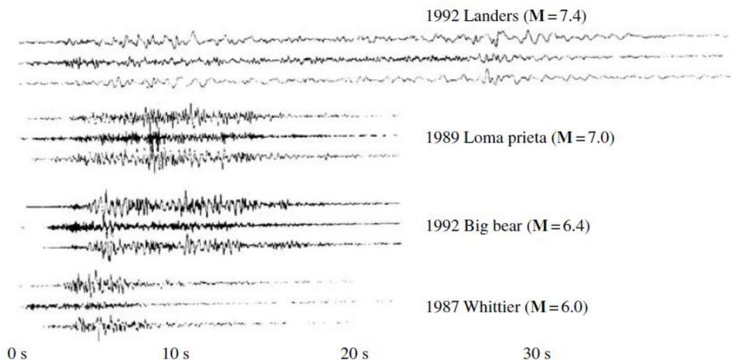
Figure (3.1) Typical earthquake accelerograms
