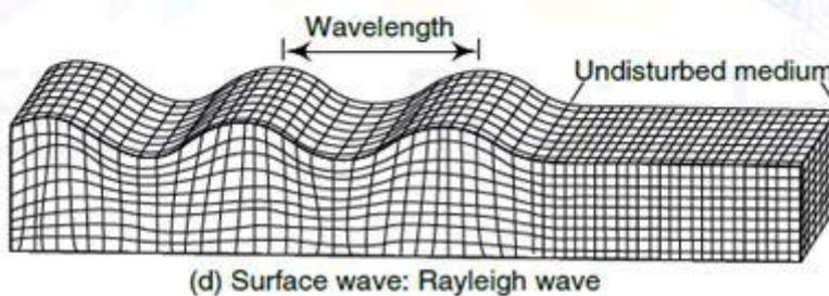
Fig. 2.6 Deformation produced by seismic waves (Chen and Lui, 2006)
