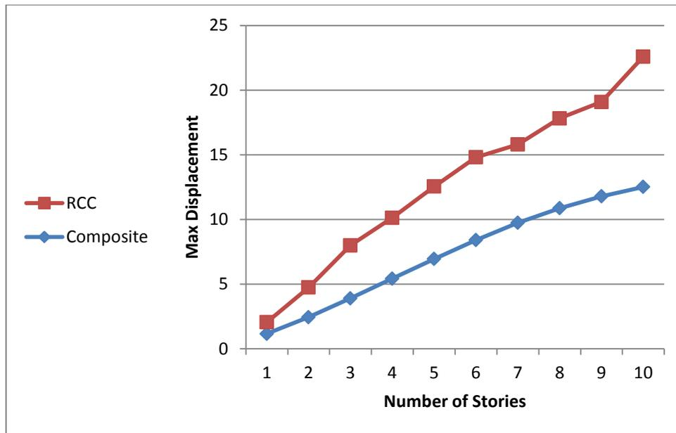
Figure (4.7) Graph of Maximum Displacement against Number of stories.
