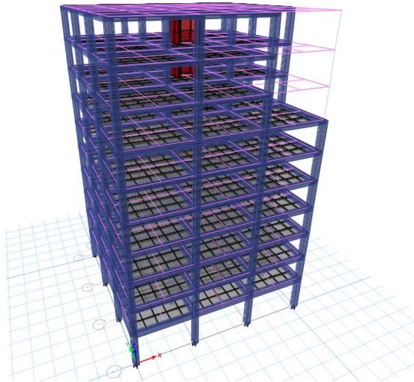
Figure (4.2) 3-D View for 10 Stories RCC Framed Structure
