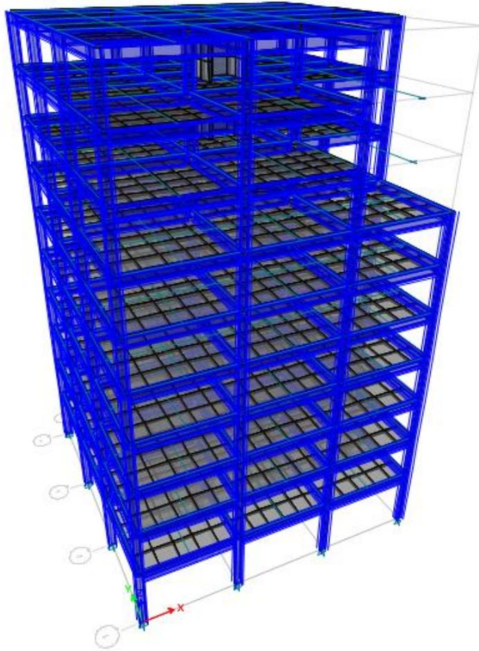
Figure (4.3) 3-D View for 10 Stories Composite Steel Frame Structure
