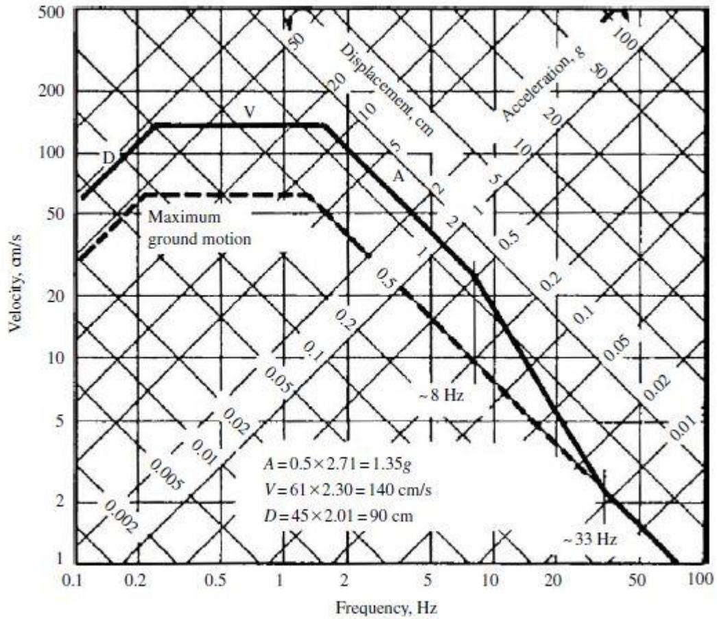
Fig. 3.5 Idealized elastic design spectrum, horizontal motion ( $ZPA^{1/4}0.5g$ , 5% damping, one sigma cumulative probability (Chen and Lui, 2006)
