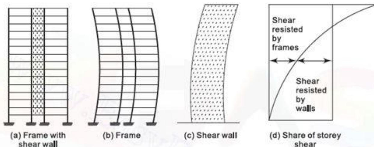
Fig. 2.9 Contribution of frames and shear walls to storey shear (Earthquake Behavior of Buildings, 2012)
