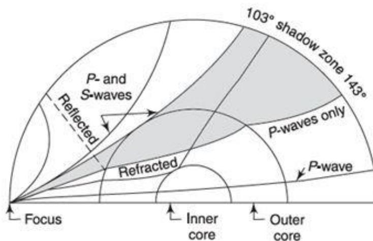
Fig. 2.5 Seismic wave paths (Chen and Lui, 2006)
