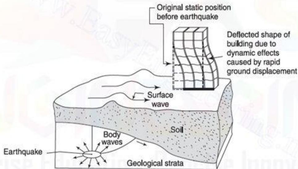
Fig. 2.4 Arrival of seismic wave (Chen and Lui, 2006)
