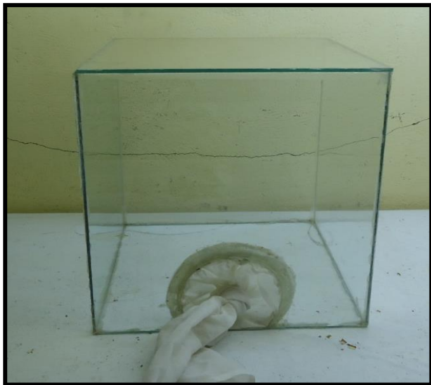
Plate No. (3) A Glass Cage for Rearing Adult Fruit Flies
