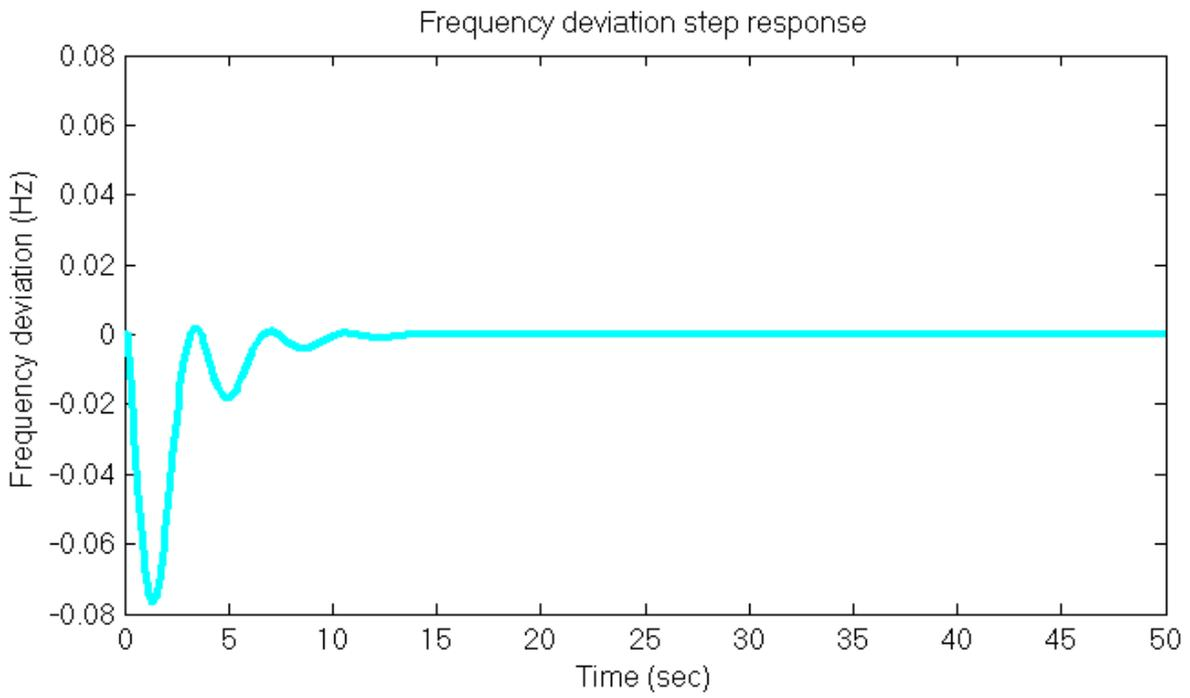
**Figure 5.29:** Frequency deviation step response of AGC including excitation system with FLC
