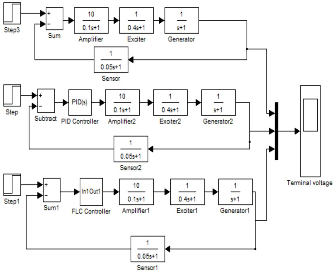
**Figure 5.8:** Simulation block diagram of (SG) with (AVR) without, PID and FLC controllers
