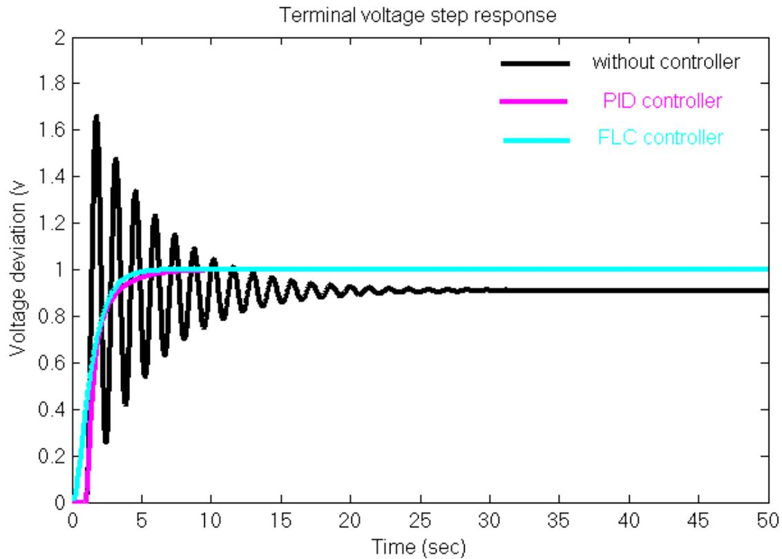
**Figure 5.9:** Terminal voltage step response of AVR loop using without, PID and FLC controllers
