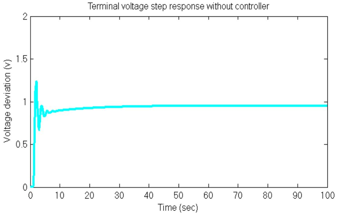
**Figure 5.23:** Terminal voltage step response of AGC including excitation system without controller
