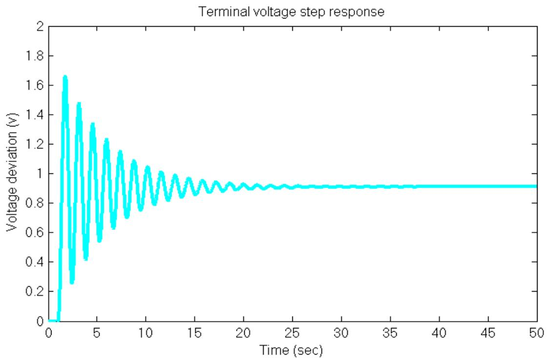
**Figure 5.2:** Terminal voltage step response of (SG) with (AVR) without control loop
