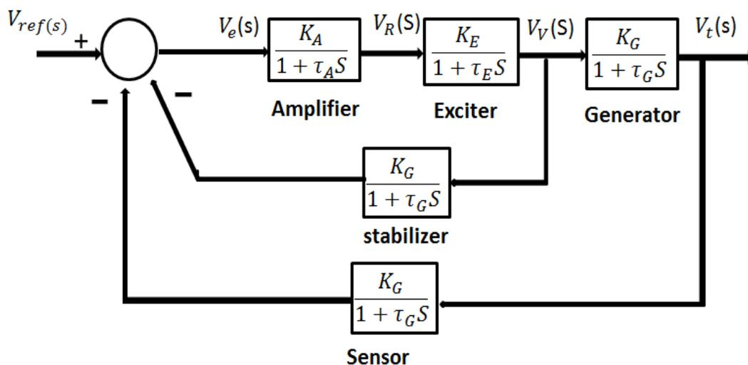
Figure 3.4: Block Diagram of the Compensated AVR System
