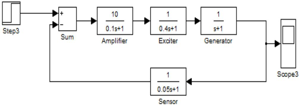
**Figure 5.1:** Simulation block diagram of (SG) with (AVR) without control loop
