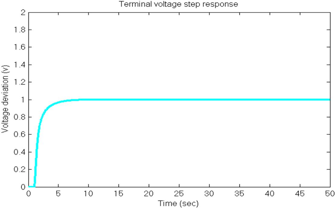
**Figure 5.4:** Terminal voltage step response of (SG) with (AVR) with PID controller
