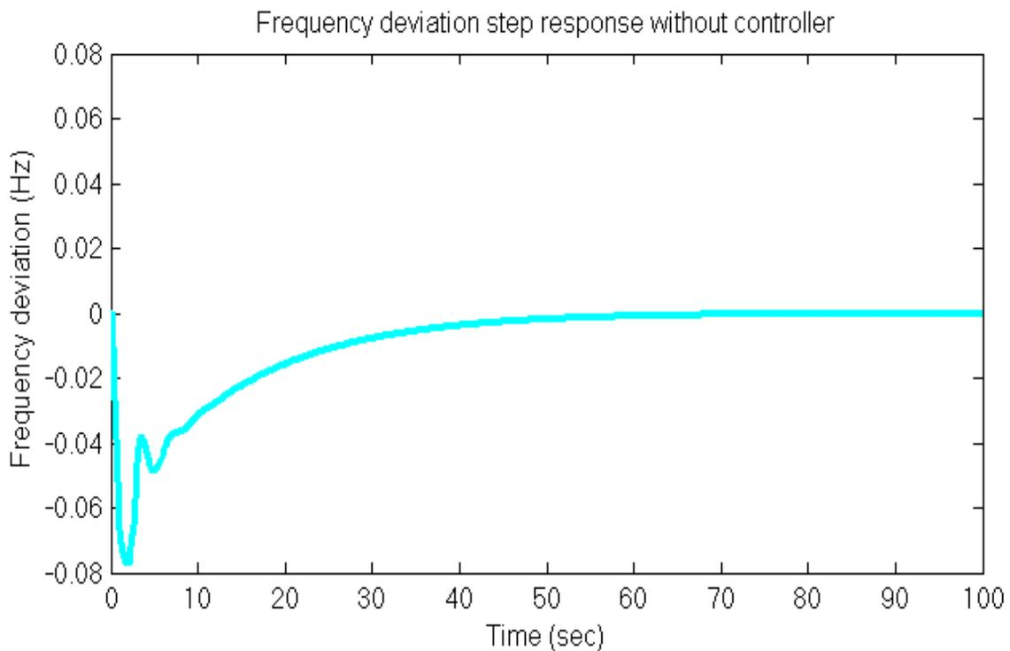
**Figure 5.22:** Frequency deviation step response of AGC including excitation system without control loop
