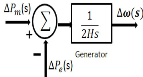
**Figure 4.1:** Generator block diagram
