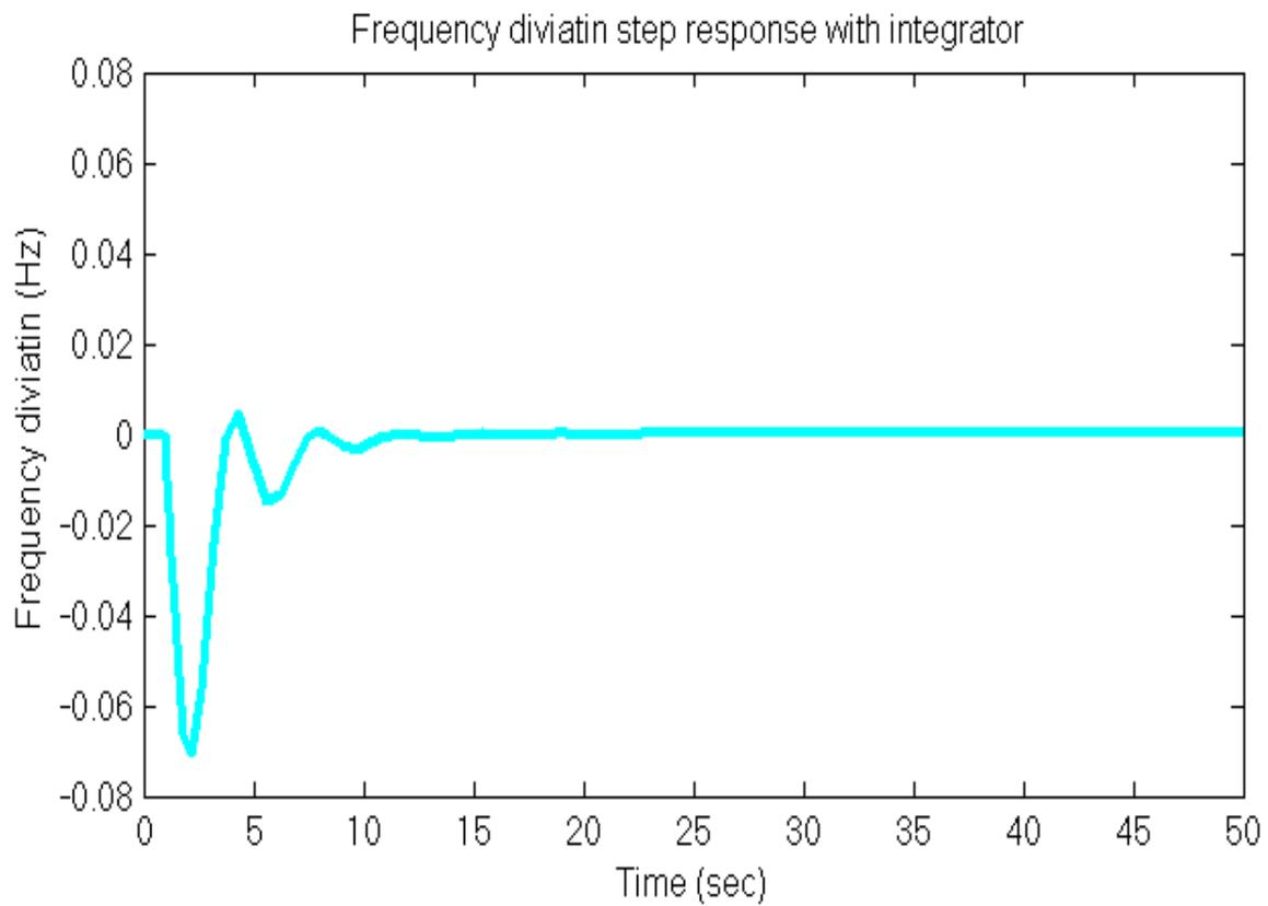
**Figure 5.20:** Frequency deviation step response of LFC with integrator
