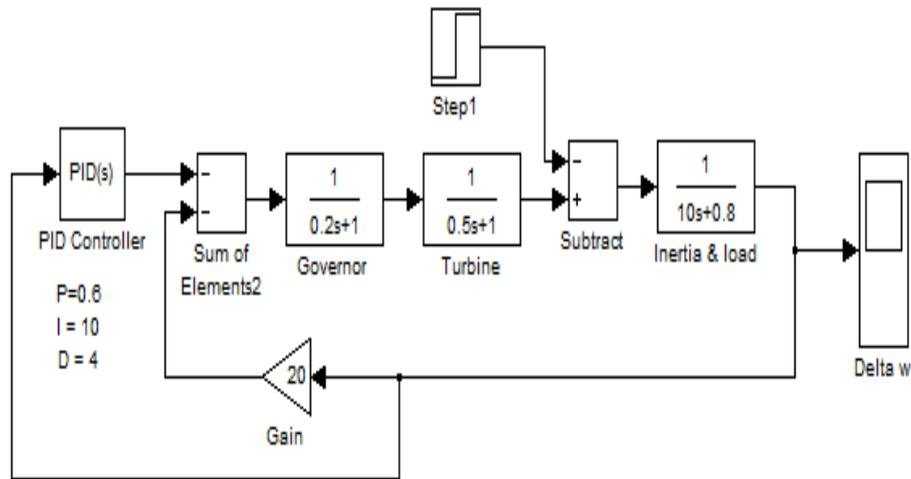
**Figure 5.12:** Simulation block diagram (LFC) with PID control loop
