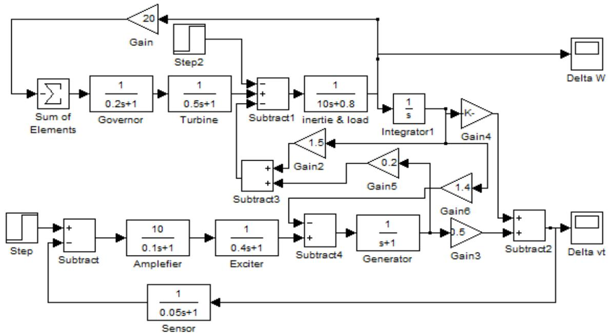
**Figure 5.21:** Simulation block diagram of AGC including excitation system without controller
