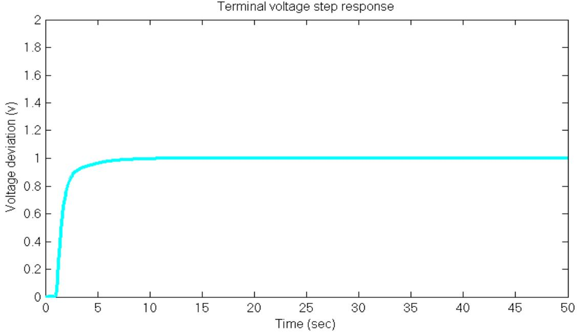
**Figure (5.26):** Terminal voltage step response of AGC including excitation system with PID controller
