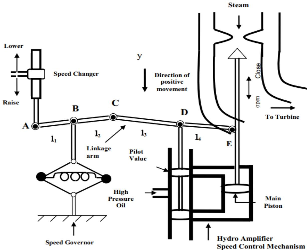
Figure 4.5: Block diagram of speed governing model
