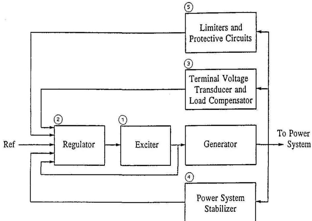
**Figure 3.1:** Shows the function block diagram synchronous Generator excitation control system
