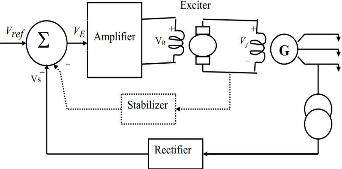
Figure 3.2: Block diagram of automatic voltage regulator
