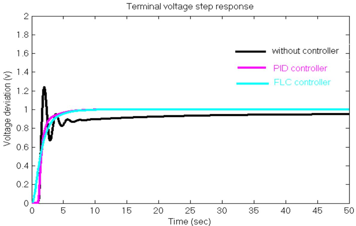
**Figure 5.31:** Terminal voltage response of AGC including excitation system for the AGC including excitation system loop using without, PID and FLC controllers
