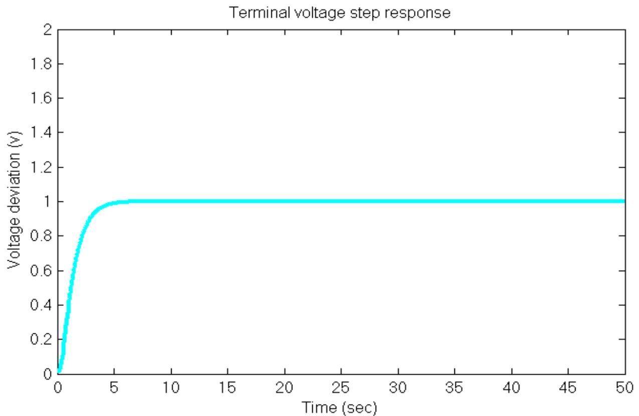
**Figure 5.7:** Terminal voltage step response of (SG) with (AVR) with FLC controller
