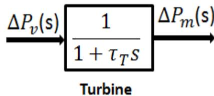
**Figure 4.4:** Block diagram for a simple non-reheat steam turbine
