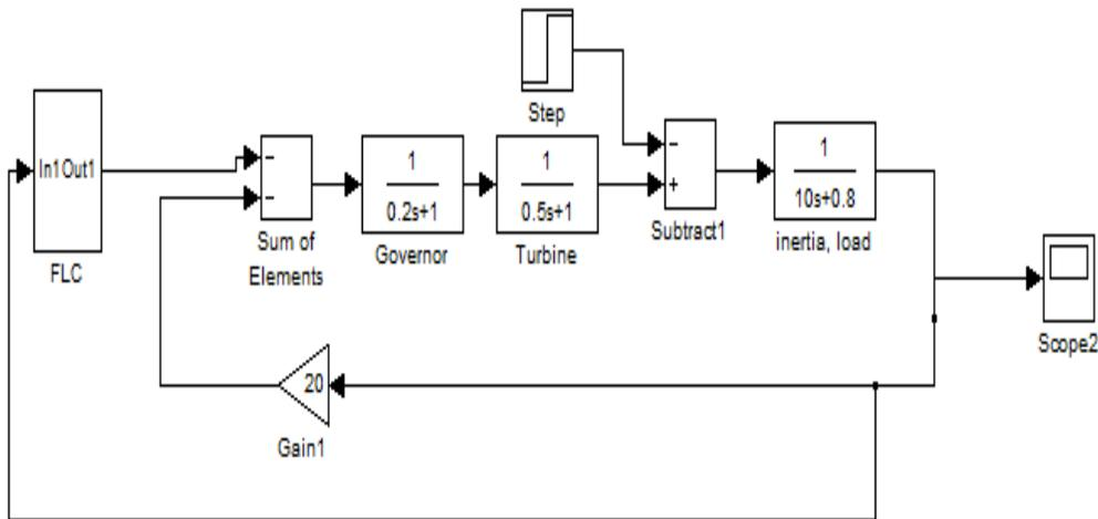
**Figure 5.14:** Simulation block diagram (LFC) with FLC controller
