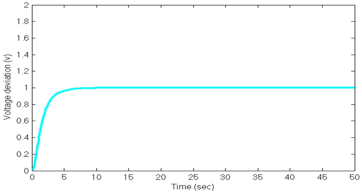
**Figure 5.30:** Terminal voltage response of AGC including excitation system with FLC
