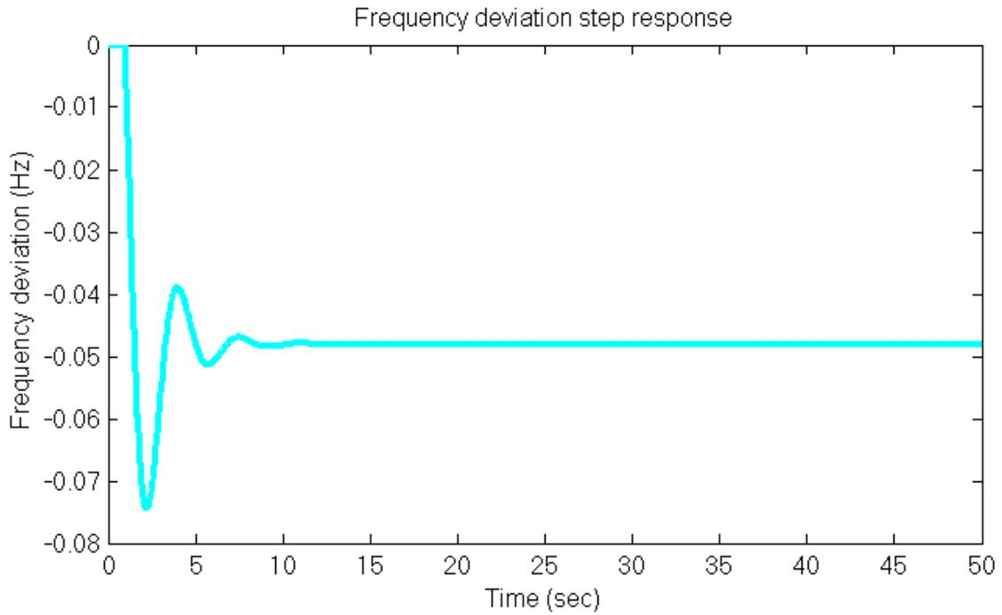
**Figure 5.11:** Frequency deviation response of (LFC) without control loop
