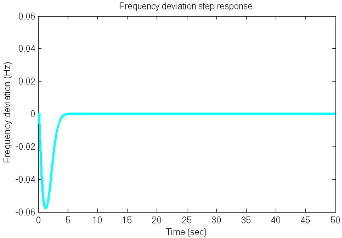
**Fig 5.16:** Frequency deviation step response of (LFC) with FLC controller
