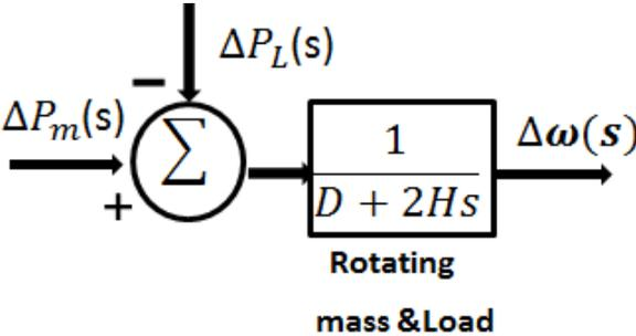
Figure 4.3: Simplified generator and load block diagram
