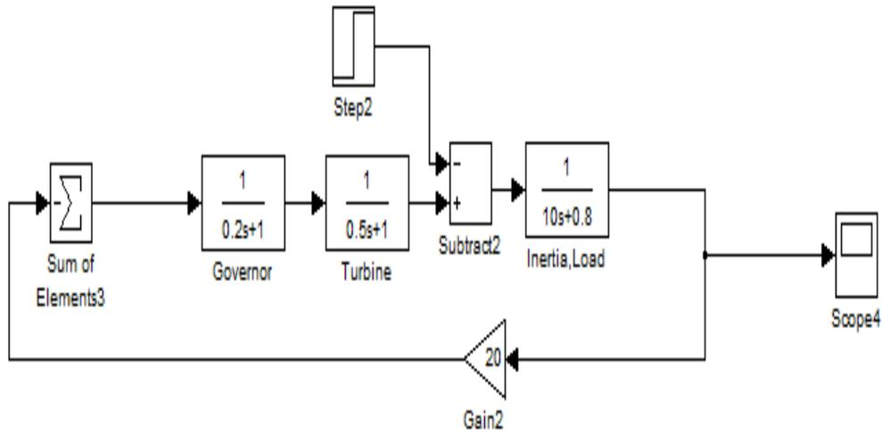
**Figure 5.10:** Simulation block diagram (LFC) without control loop
