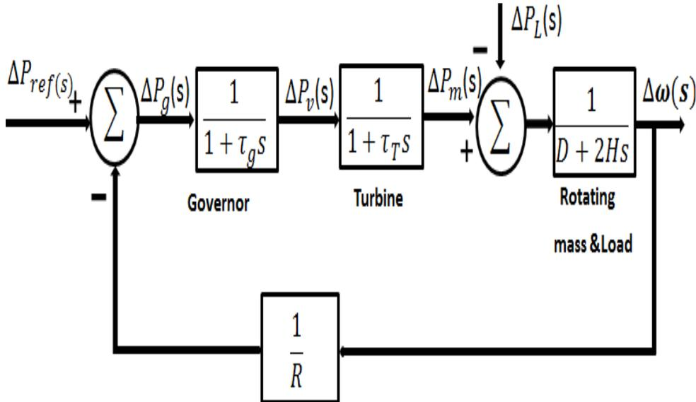
**Figure 4.7:** LFC block diagram of an isolated power system
