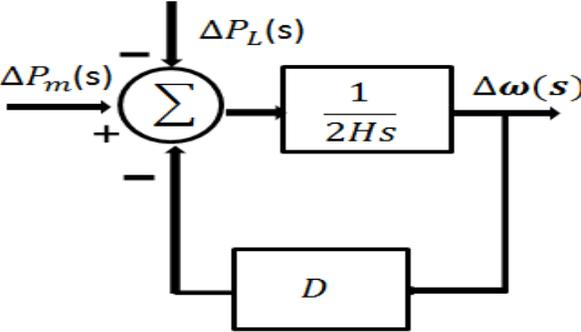
Figure 4.2: Generator and load block diagram
