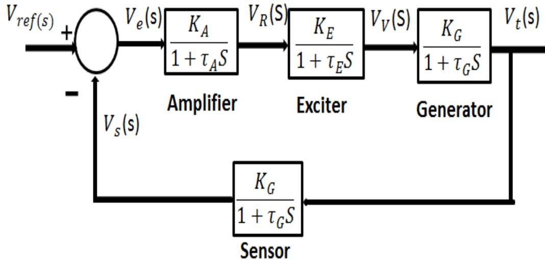
Figure 3.3: A simplified automatic Voltage Regulator (AVR) block diagram
