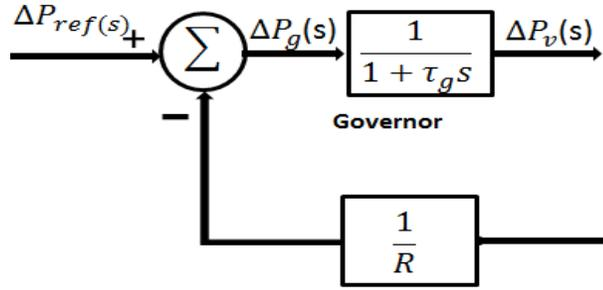
**Figure 4.6:** Block diagram for speed governing system of steam turbine
