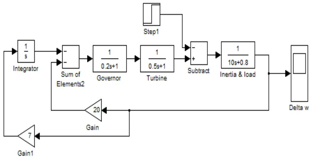
**Figure 5.19:** Simulink diagram for LFC loop with integrator (Rest Action)
