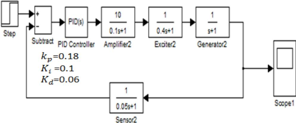
**Figure 5.3:** Simulation block diagram of (SG) with (AVR) with PID controller
