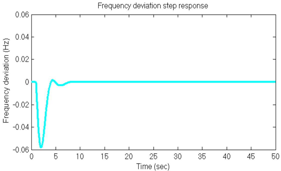
**Figure 5.13:** Frequency deviation step response of (LFC) with PID control loop
