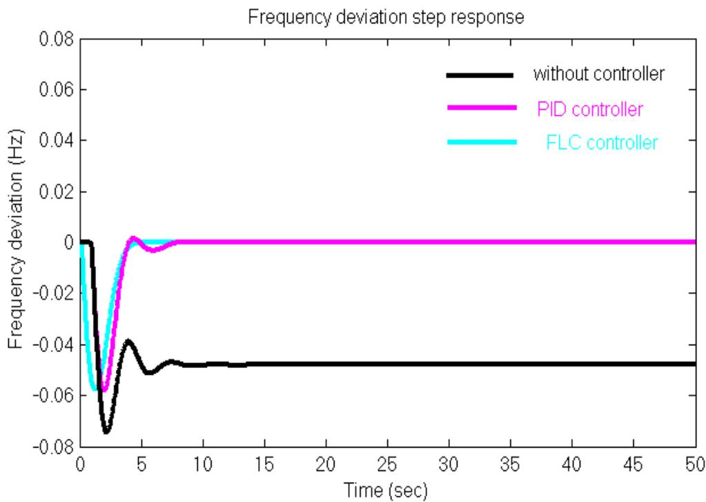
**Figure 5.18:** Frequency deviation step response of the LFC loops using three cases
