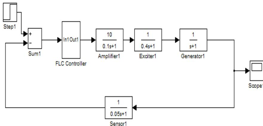
**Figure 5.5:** Simulation block diagram of (SG) with (AVR) with FLC controller
