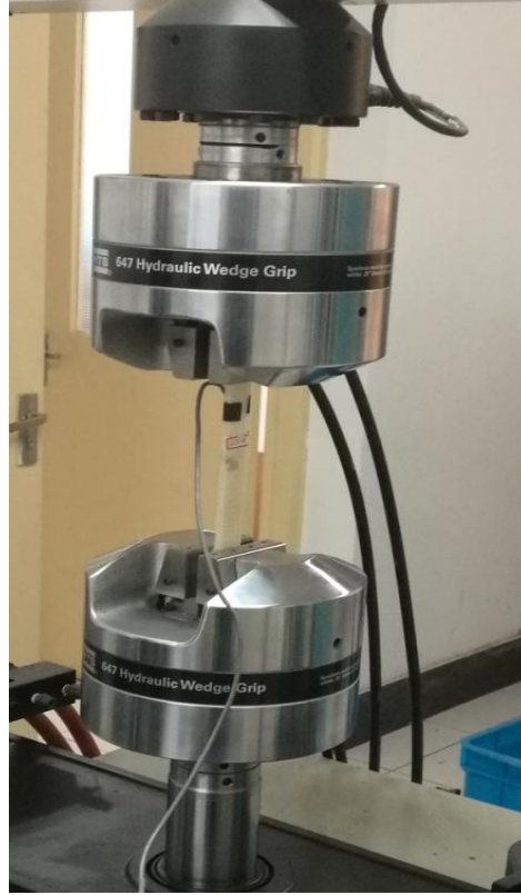
Fig (3.10): MTS 810 Material Test System-647 Hydraulic wedge Grip machine.
