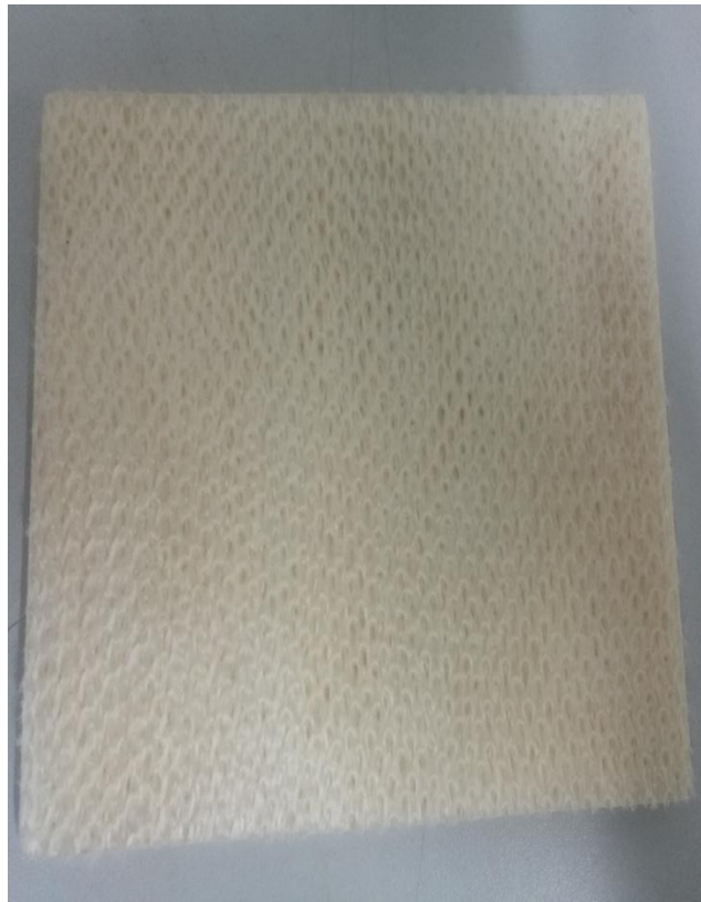
Fig (3.14): Specimen preparation for impact drop weight.
