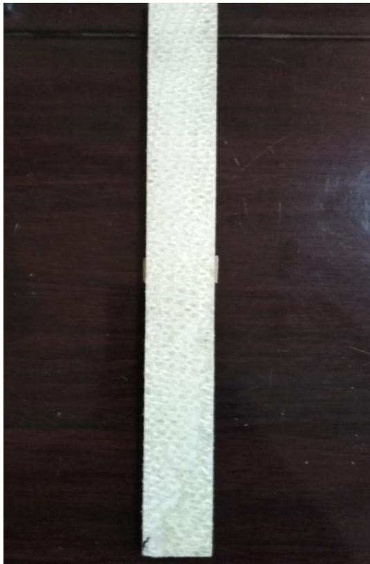
Fig (3.13): Specimen preparation for tensile test.
