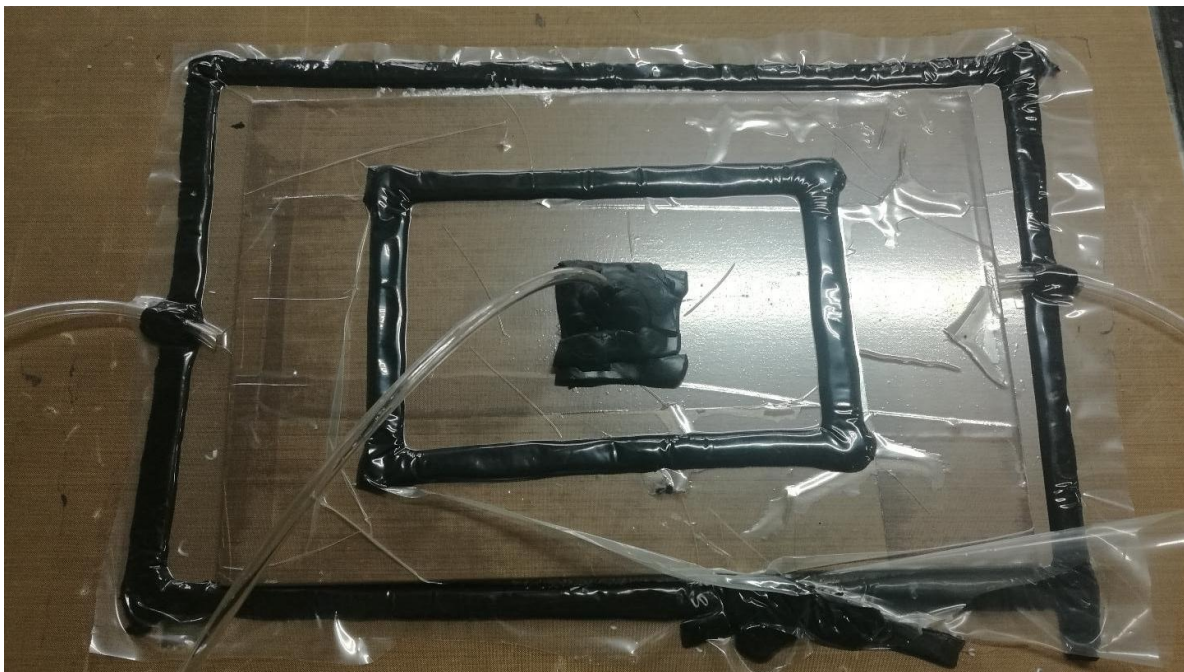
Fig (3.8): Resin Transfer Molding (RTM) process.
