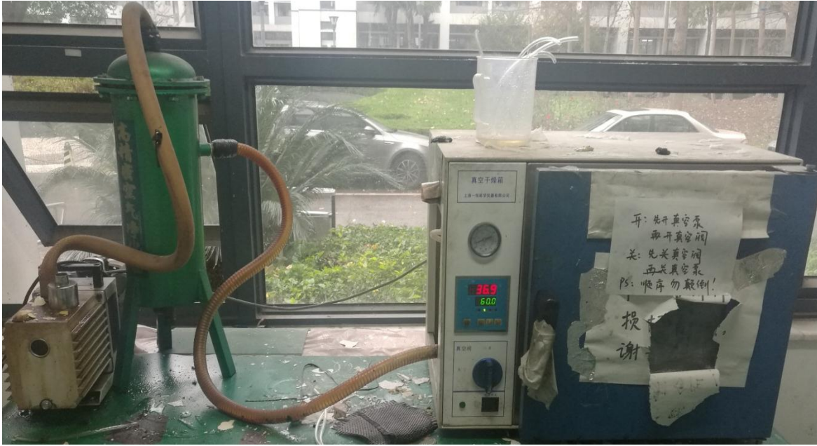
Fig(3.6):Treatment of resin in 60c° ( miniature pressure and temperature).
