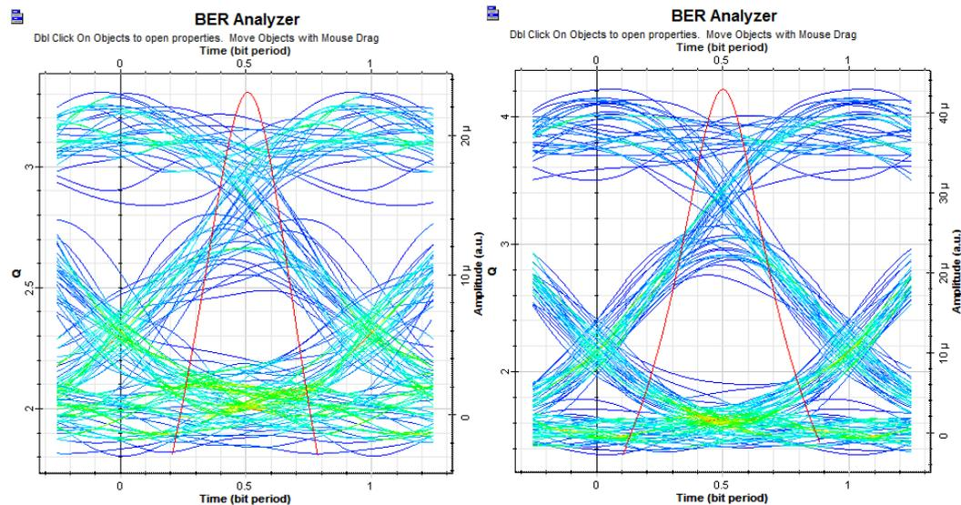
Fig.4.9 Eye diagrams comparing system I (a) and system II (b) under medium rain condition.
