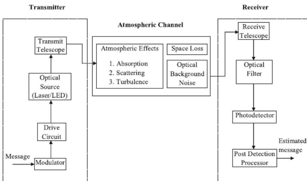
Fig. 2.2 Block diagram of FSO communication link [1].
