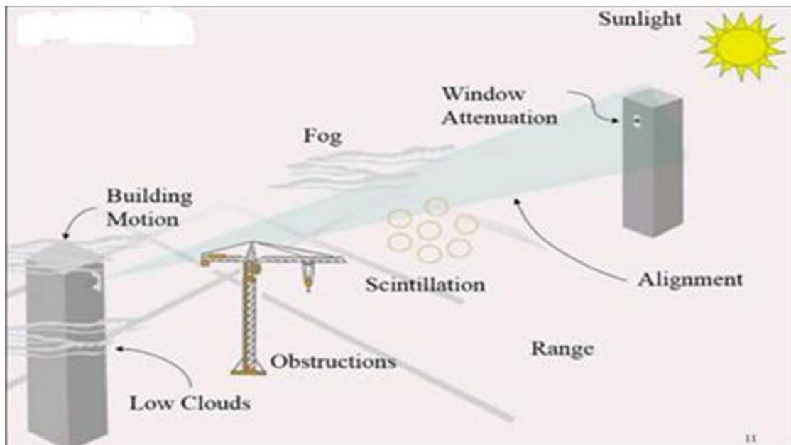
Fig. 3.5 A compact view of degrading elements of an FSO link [2].
