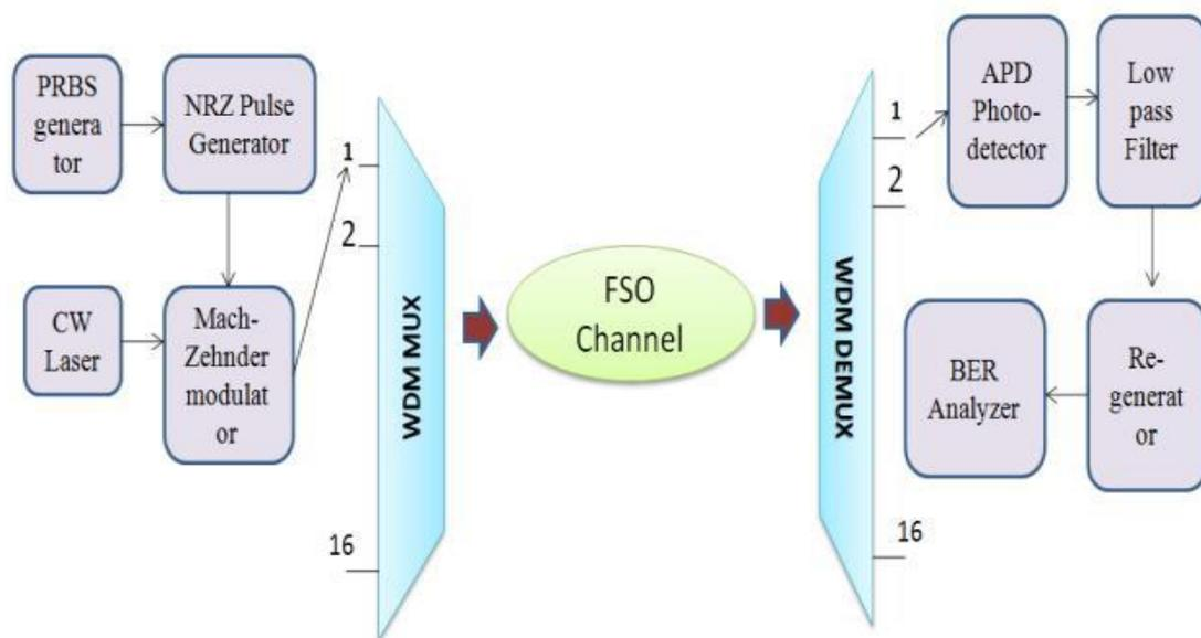
Fig. 3.6: Block diagram of WDM-FSO system [5]
