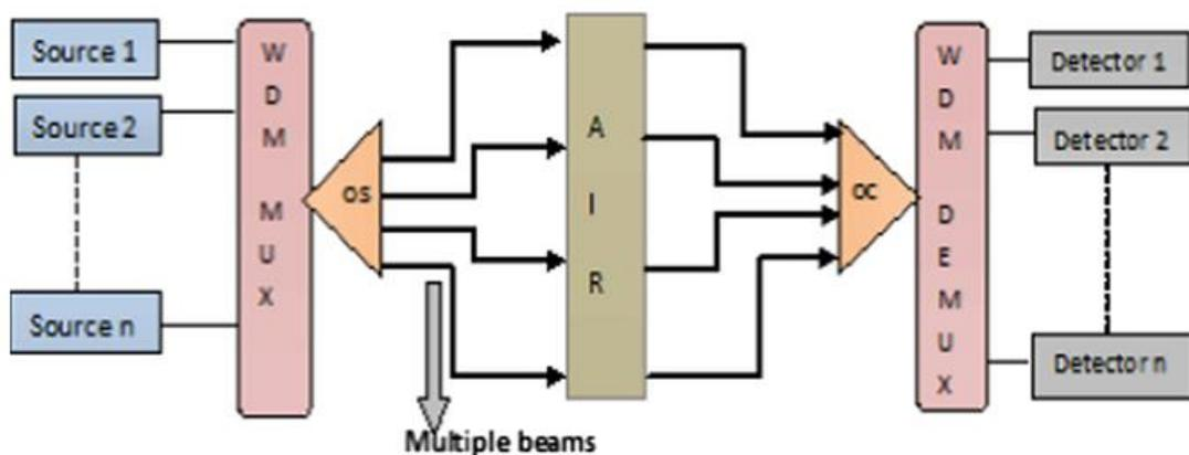
Fig. 3.4 Hybrid Multi beam WDM-FSO System [9]
