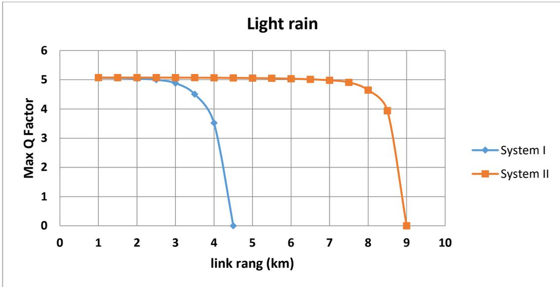
Fig. 4.4 Comparison of system I and II under light rain in terms of Max Q factor v/s link distance graph.
