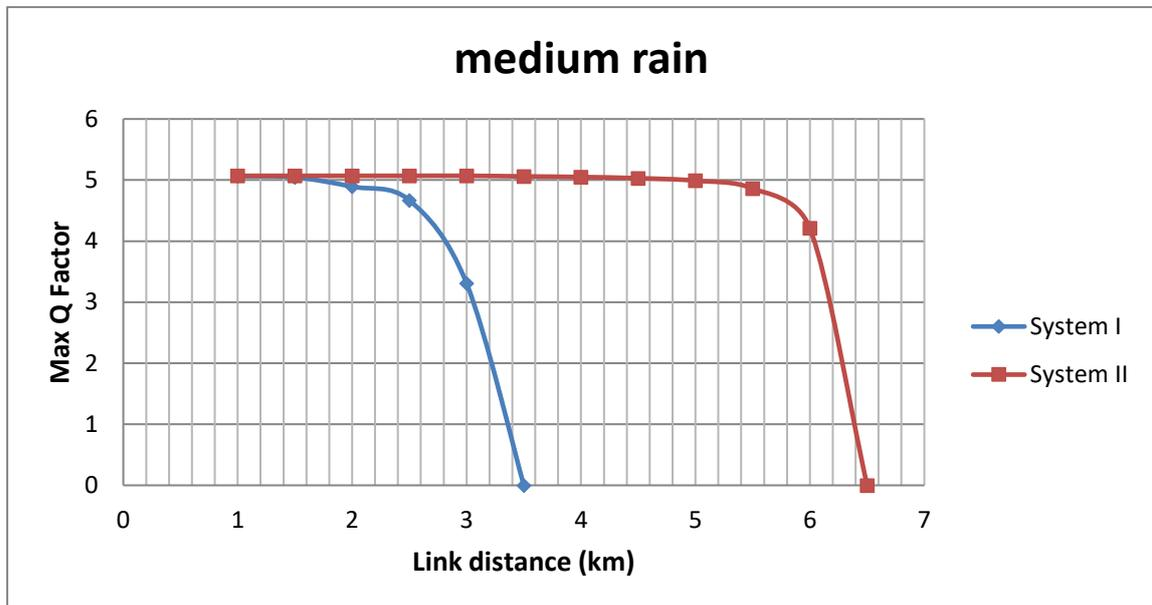
Fig. 4.7 Comparison of system I and II under medium rain in terms of Max Q factor v/s link distance graph.
