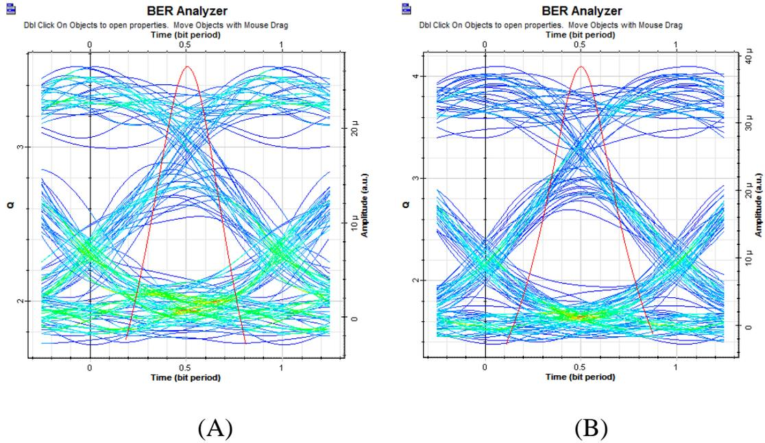
Fig.4.6 Eye diagrams comparing system I (a) and system II (b) under light rain condition.
