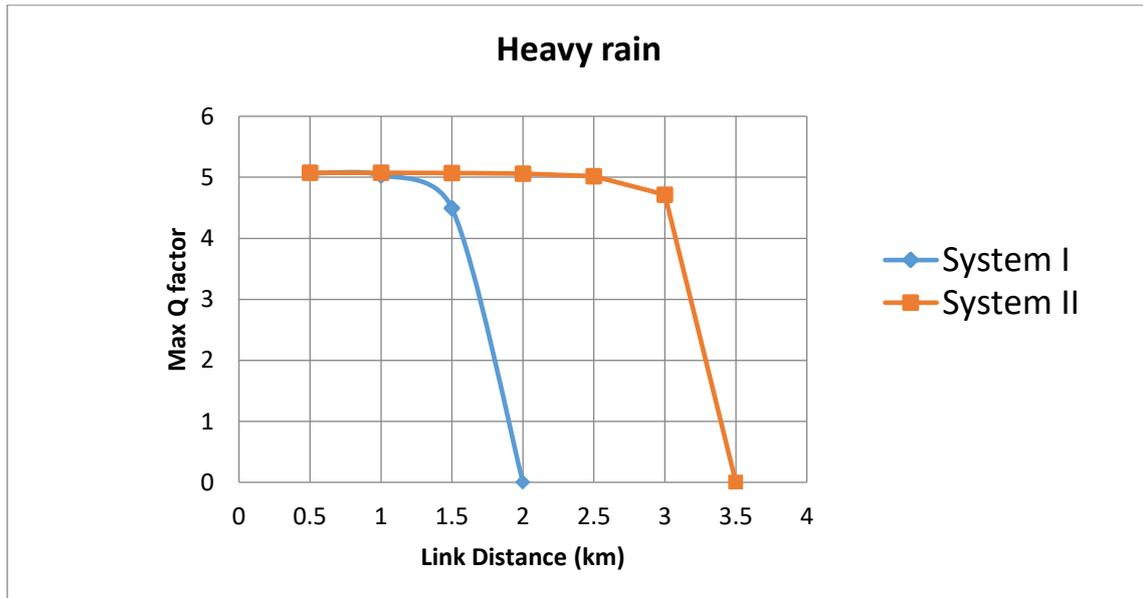
Fig. 4.10 Comparison of system I and II under heavy rain in terms of Max Q factor v/s link distance.
