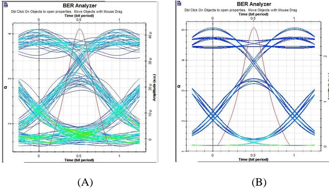
Fig.4.3 Eye diagrams comparing system I (a) and system II (b) under clear weather conditions.
