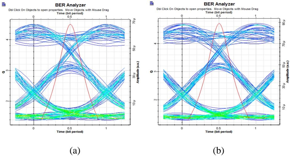
Fig.4.12 Eye diagrams comparing system I (a) and system II (b) under heavy rain condition.
