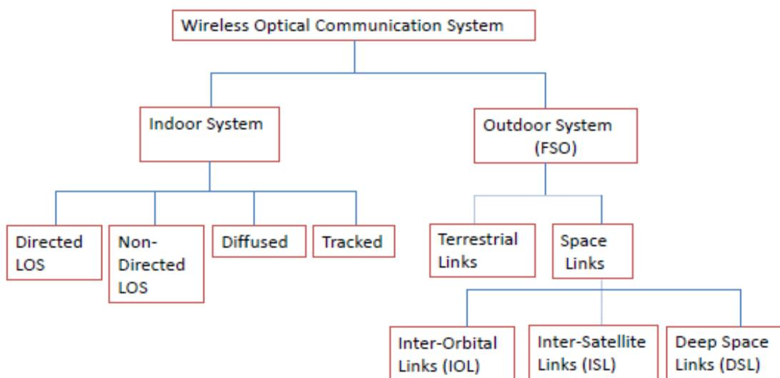
Fig. 2.1 Classification of wireless optical communication system[1]
