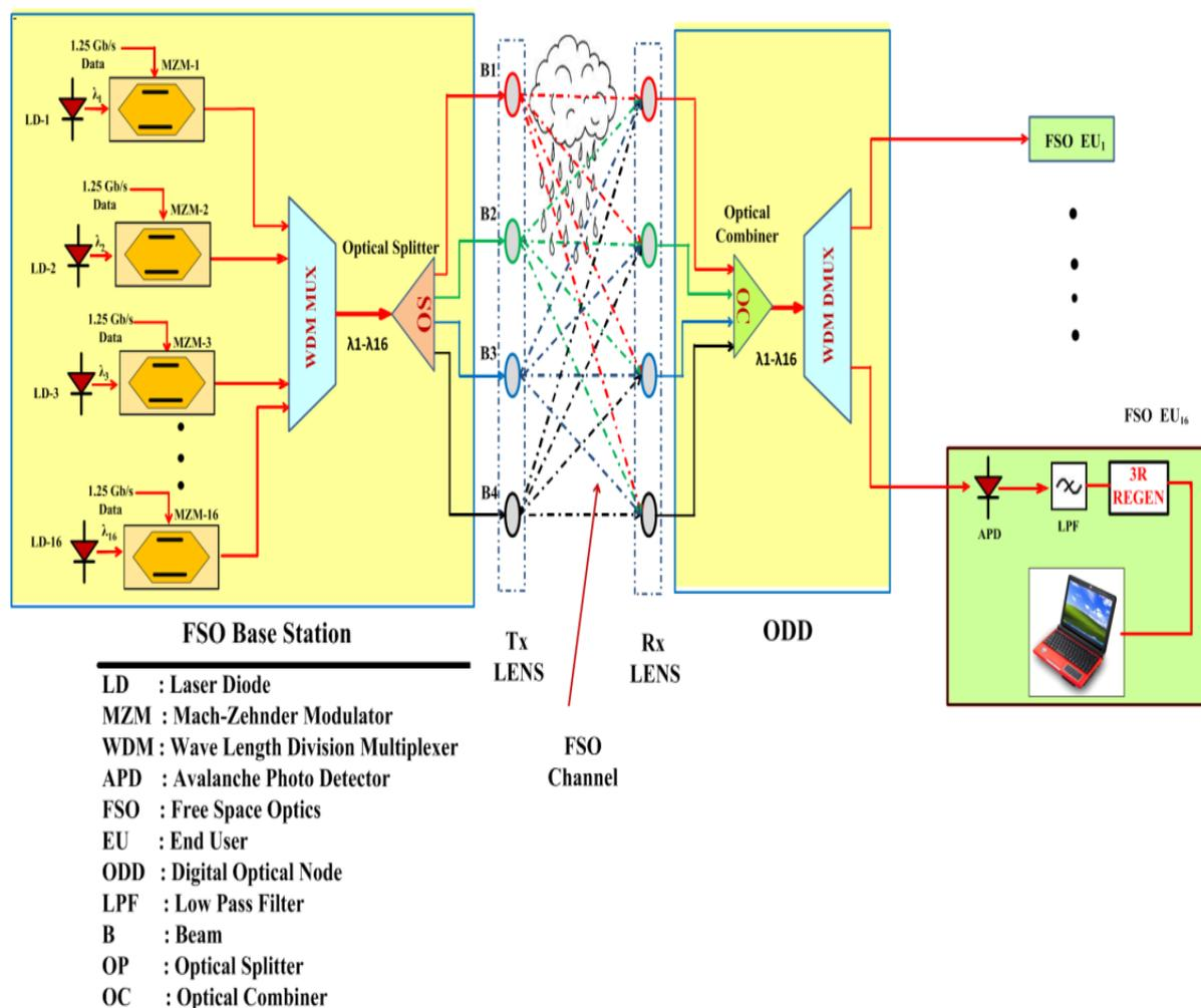
Fig. 3.10 Block diagram of Hybrid WDM/multi-beam FSO system [1]
