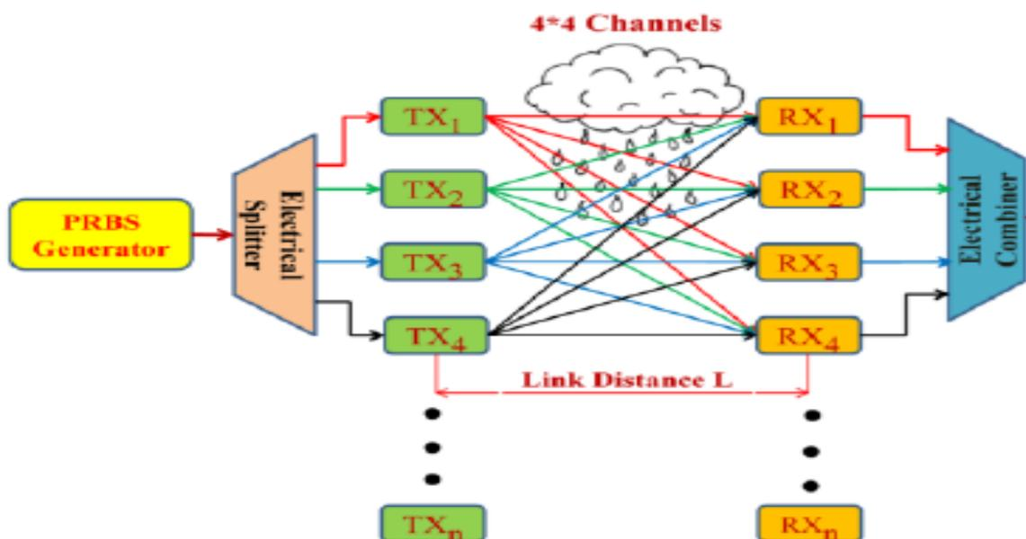
Fig. 3.3: Block diagram of a multi-beam FSO system [6]
