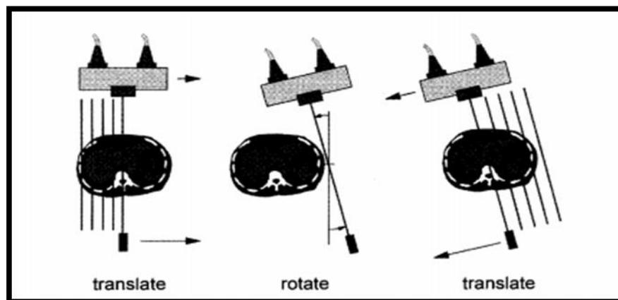
*Fig (2.6):First-generation (rotate/translate) computed tomography CT. The x-ray tube and a single detector translate across the field of view, producing a series of parallel rays. The system then rotates slightly and translates back across the field of view, producing ray measurements at a different angle. This processes repeated at 1-degree intervals over 180 degrees, resulting in the complete CT data set.(Bushberg et al., 2003)*
