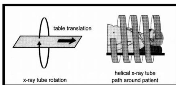
***Fig (2.8): helical computed tomographic scanners.***
