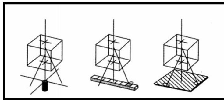
*Pencil beam      Fan beam      Open beam*
