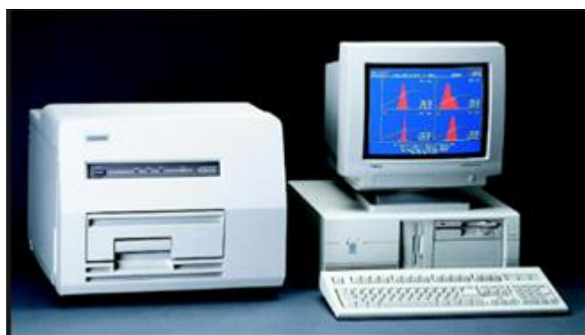
Figure 3.6 shown the TLD reader system (PCL3 from PTW) used in this research
