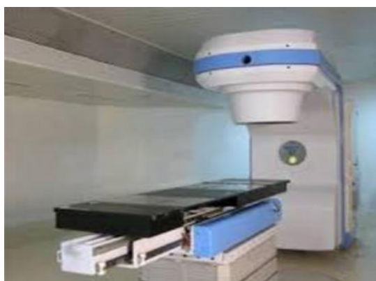
Fig. 3.3 shown the cobalt-60 machine that used to irradiate the films
