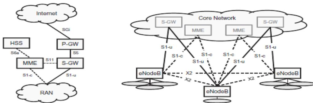
Figure 2.1: Core-network (EPC) architecture and Radio-access-network interfaces [5].
