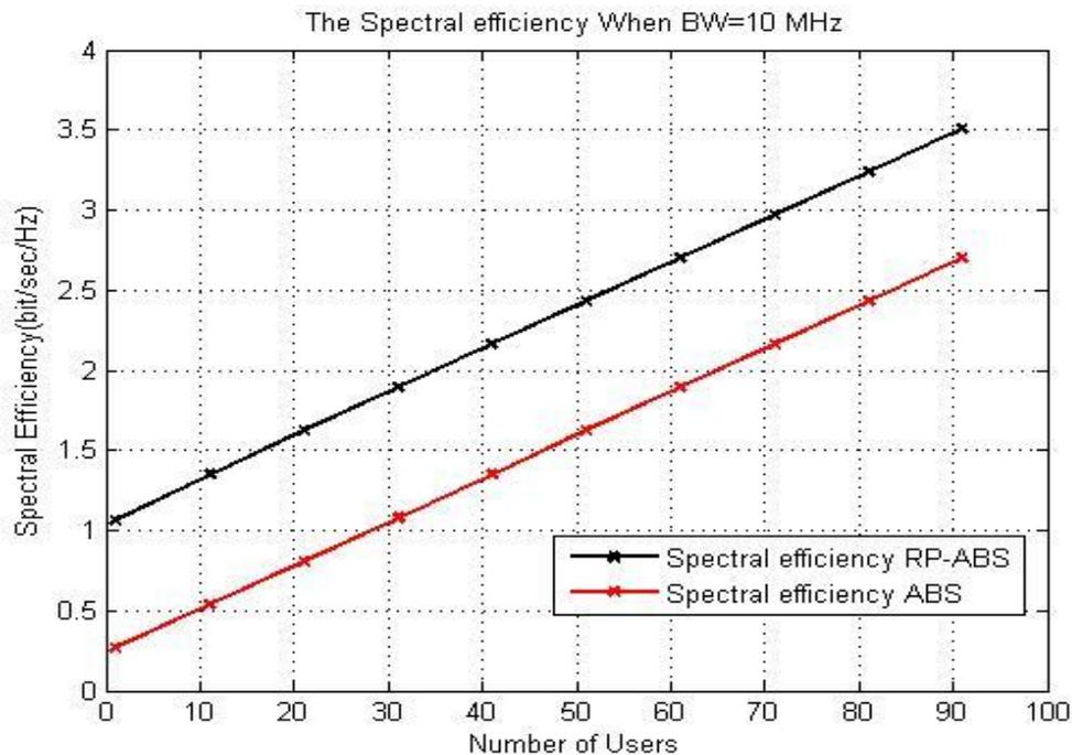
Figure (4.3a): Comparison of Spectral efficiency for RP-ABS and ABS (BW=10MHz)
