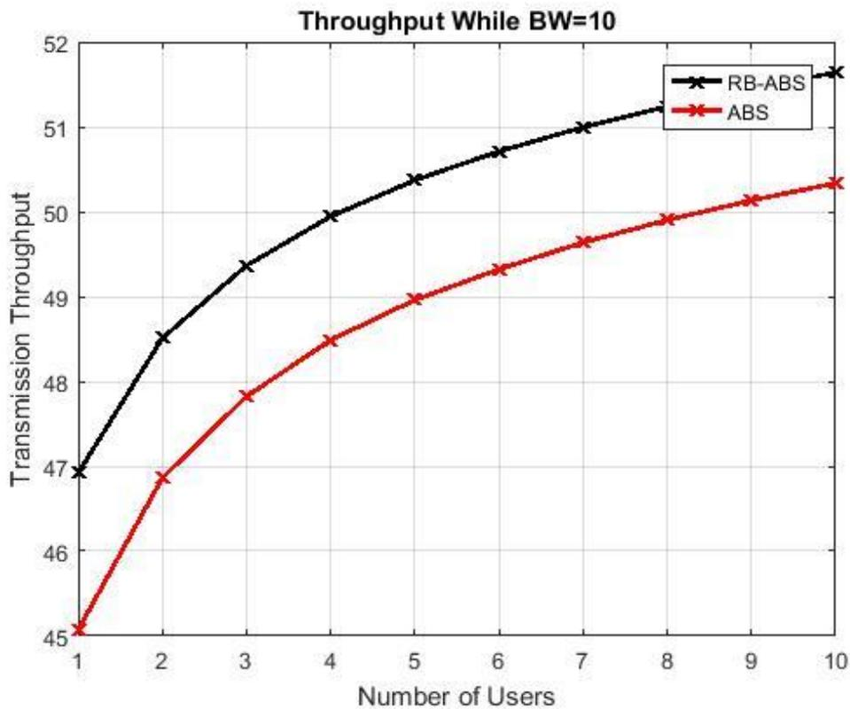
Figure (4.2a): Comparison of Throughput for RP-ABS and ABS (BW=10MHz)
