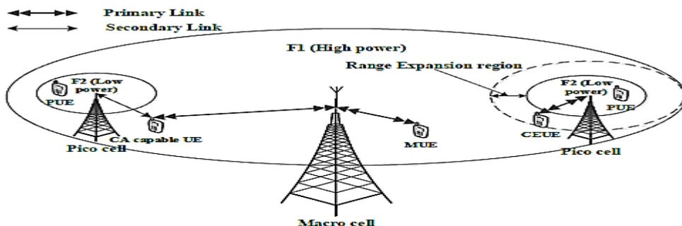
Figure 2.5: Heterogeneous deployment in LTE-Advanced network[9]
