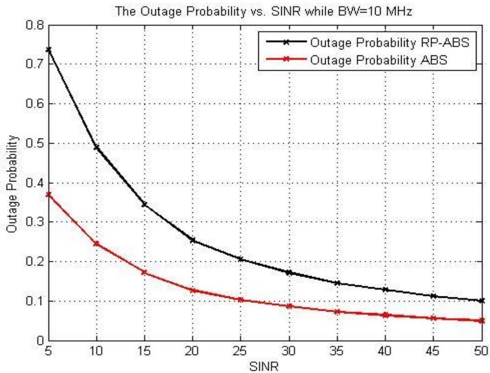
Figure (4.5b): Comparison of outage probability for RP-ABS and ABS (BW=10MHz)
