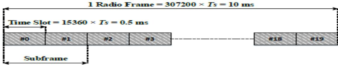
Figure 2.2: Radio Frame Structure (type1)[7]
