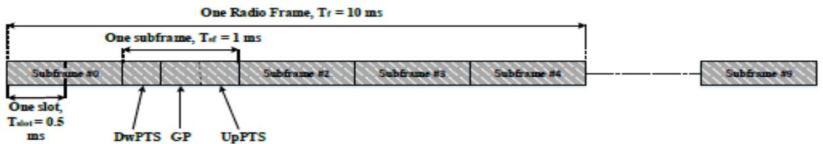
Figure 2.3: Radio Frame Structure (type 2)[7]
