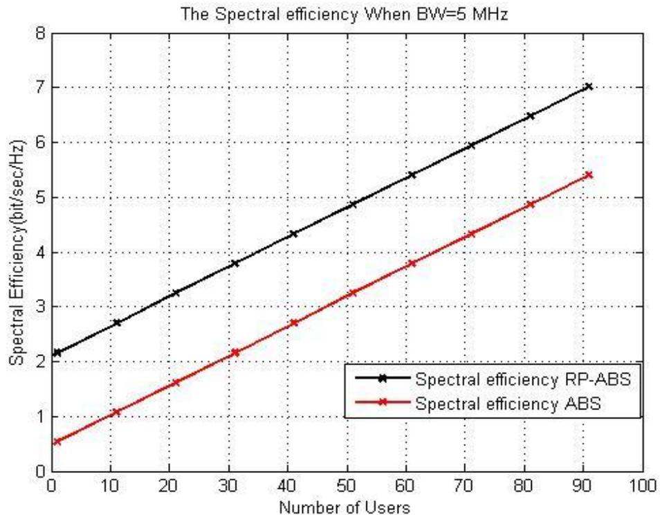
Figure (4.3b): Comparison of Spectral efficiency for RP-ABS and ABS (BW=5MHz)
