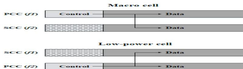
Figure 2.8: Frame configuration for CA-based ICIC scheme[27]
