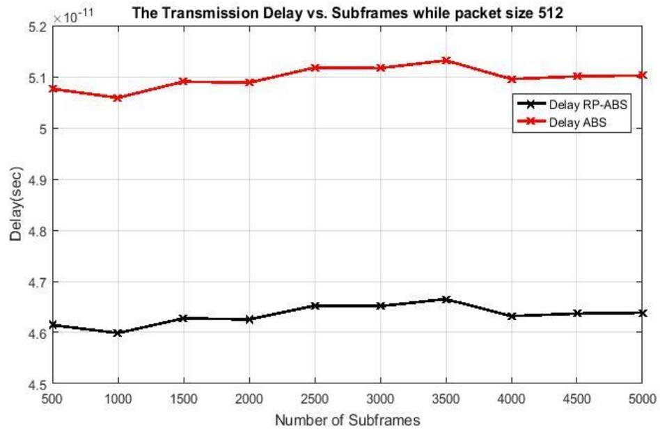
Figure (4.4a): Comparison of delay for RP-ABS and ABS (packet size 512)
