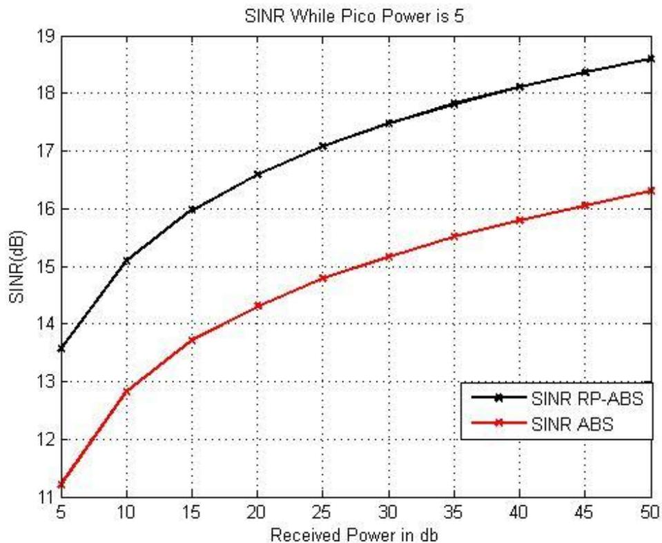
Figure (4.1b): Comparison of SINR for RP-ABS and ABS (pico power 5dB)
