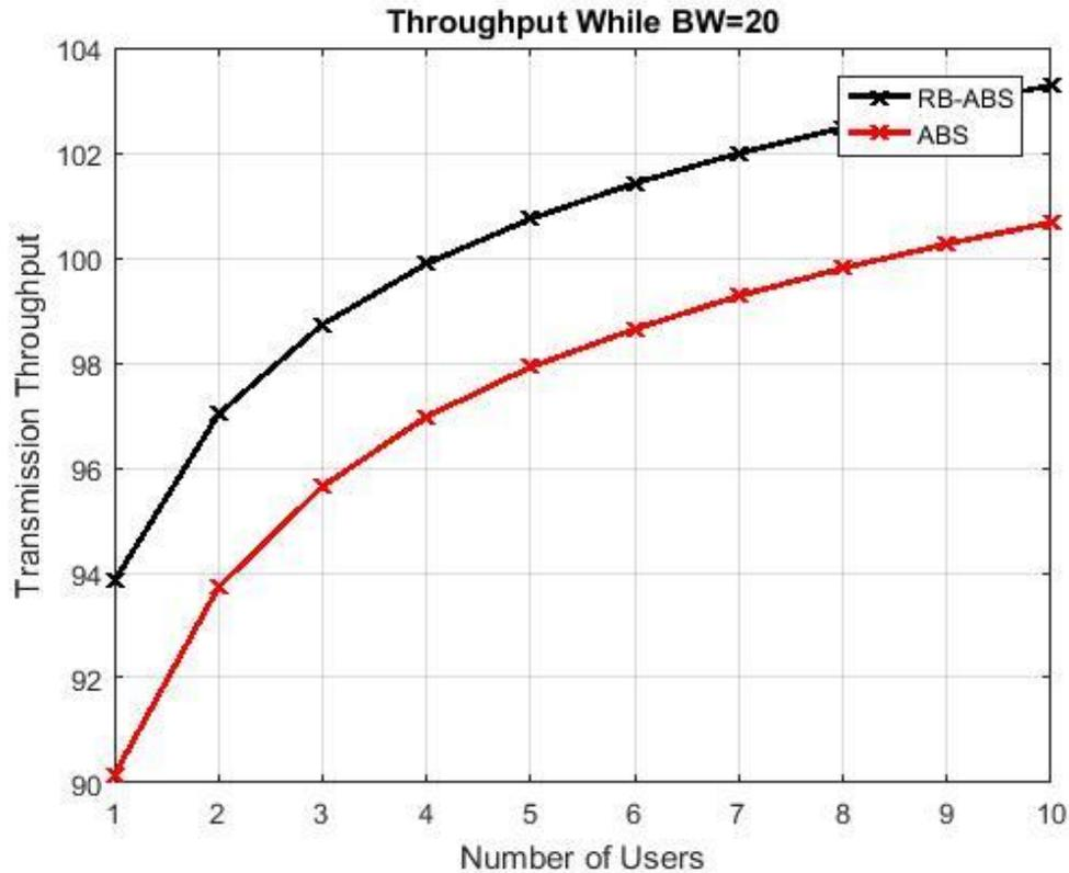
Figure 4.2b: Comparison of Throughput for RP-ABS and ABS (BW=20MHz)
