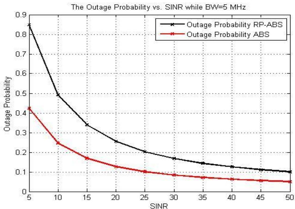
Figure (4.5a): Comparison of outage probability for RP-ABS and ABS (BW=5MHz)
