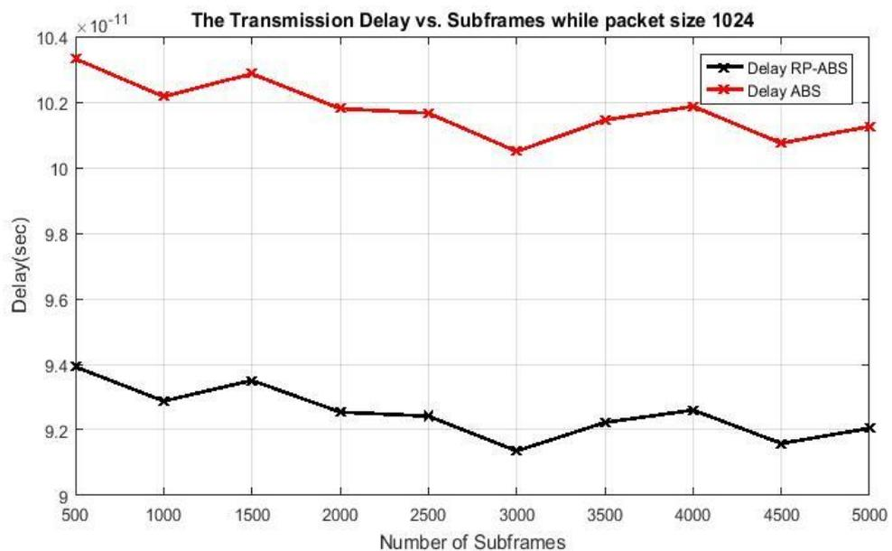
Figure (4.4b): Comparison of delay for RP-ABS and ABS (packet size 1024)
