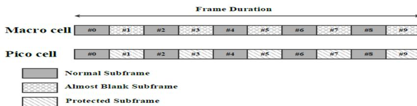
Figure 2.9: (ABS) for range expansion in HetNet [31]
