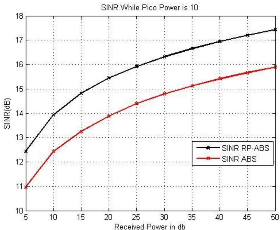
Figure (4.1a): Comparison of SINR for RP-ABS and ABS (pico power 10dB)
