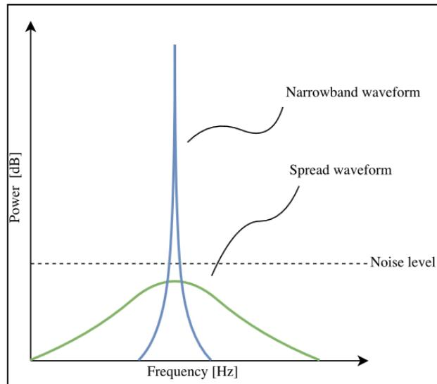
Figure 2.2: Waveforms for UNB and SSM
