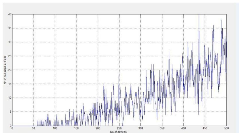
Figure 4.2 collisions of packets in 125 KHz bandwidth (500 devices)
