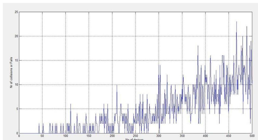
Figure 4.3: collisions of packets in 250 KHz bandwidth (500 devices)
