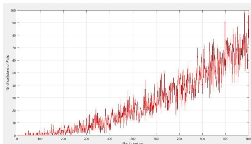
Figure 4.21: collisions of packets in 200 KHz bandwidth (1000 devices)
