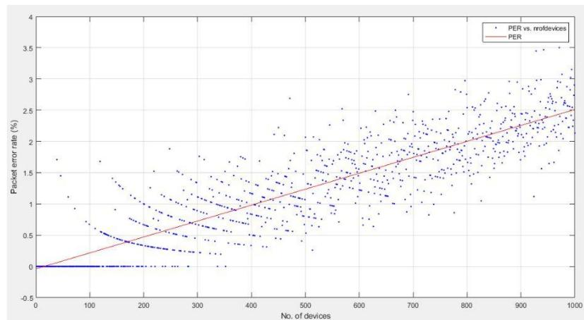
Figure 4.23: PER in 200 KHz bandwidth (1000 devices)
