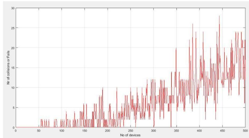
Figure 4.20: collisions of packets in 200 KHz bandwidth (500 devices)
