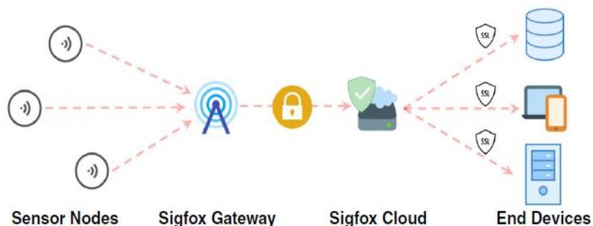
Figure 2.4: High level description of the Sigfox network architecture
