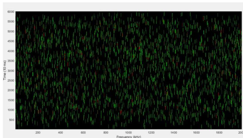
Figure 4.25: Spectrum in 200 KHz (1000 devices)
