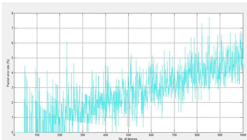
Figure 4.12: PER in 250 KHz bandwidth (1000 devices)
