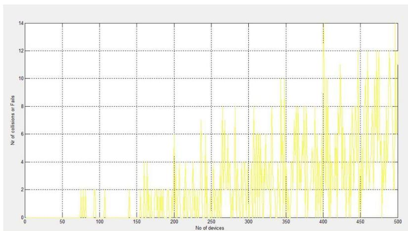
Figure 4.10: PER in 500 KHz bandwidth (500 devices)
