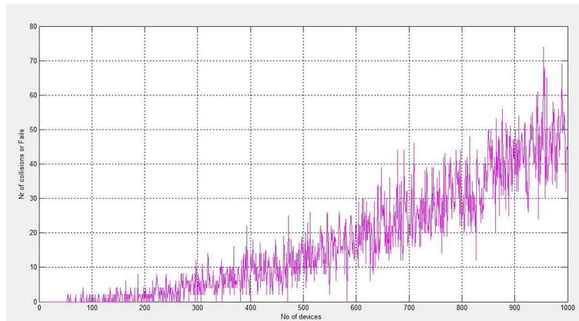
Figure 4.6: collisions of packets in 250 KHz bandwidth (1000 devices)
