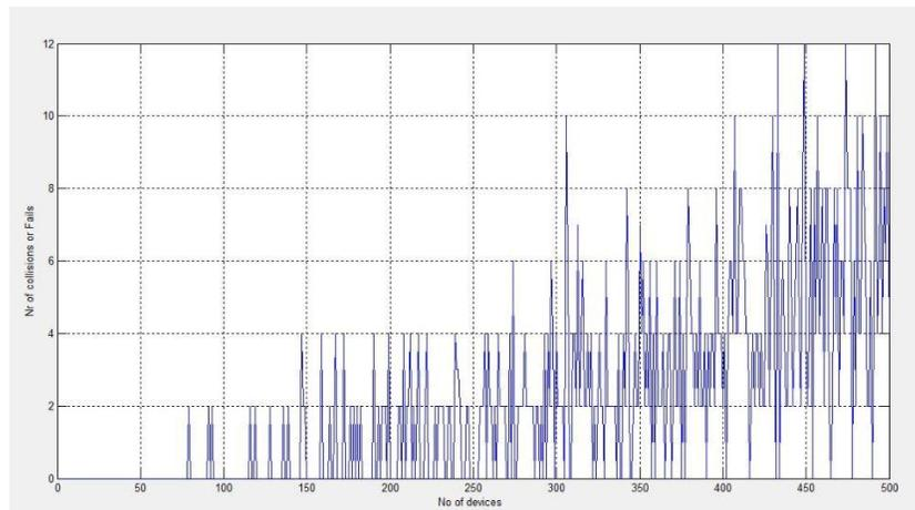
Figure 4.4: collisions of packets in 500 KHz bandwidth (500 devices)
