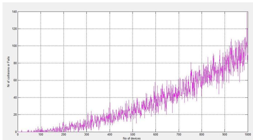
Figure 4.5: collisions of packets in 125 KHz bandwidth (1000 devices)
