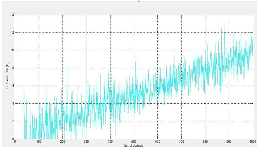
Figure 4.11: PER in 125 KHz bandwidth (1000 devices)
