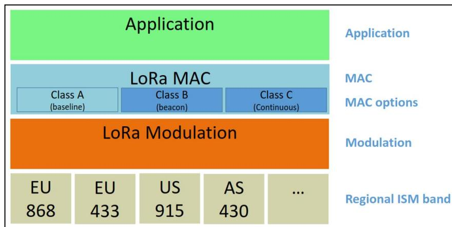
Figure 2.1: LoRaWAN Classes and layers
