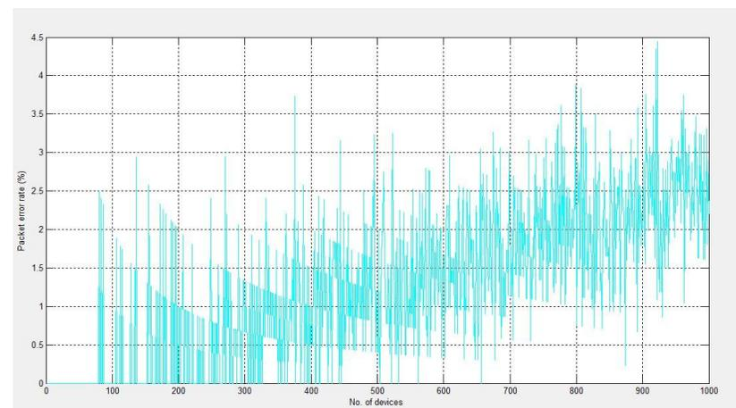
Figure 4.13: PER in 500 KHz bandwidth (1000 devices)
