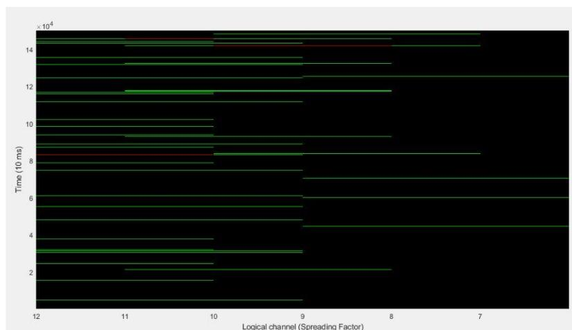
Figure 4.15: Spectrum in 250 KHz (500 devices)
