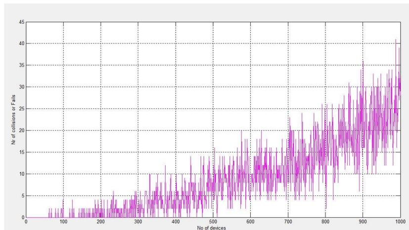
Figure 4.7: collisions of packets in 500 KHz bandwidth (1000 devices)
