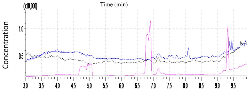
Figure 5 Standards Chromatograms, retention time (min), total areas and concentration of 3-MCPD.
