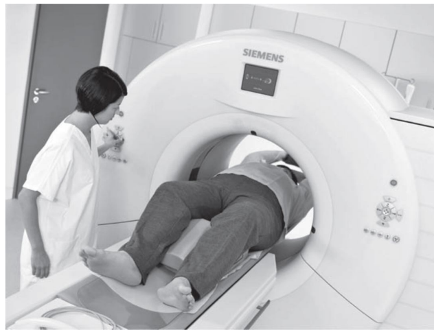
Figure (2.12): CT scanner .The gantry and patient table are Major components of a CT image system. . (Lois ,2011)
