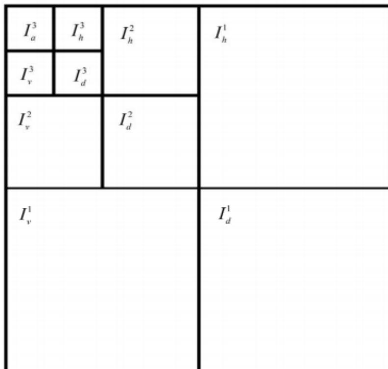
**Fig (2-15):Pyramidal structure of DWT up to level 3.**
