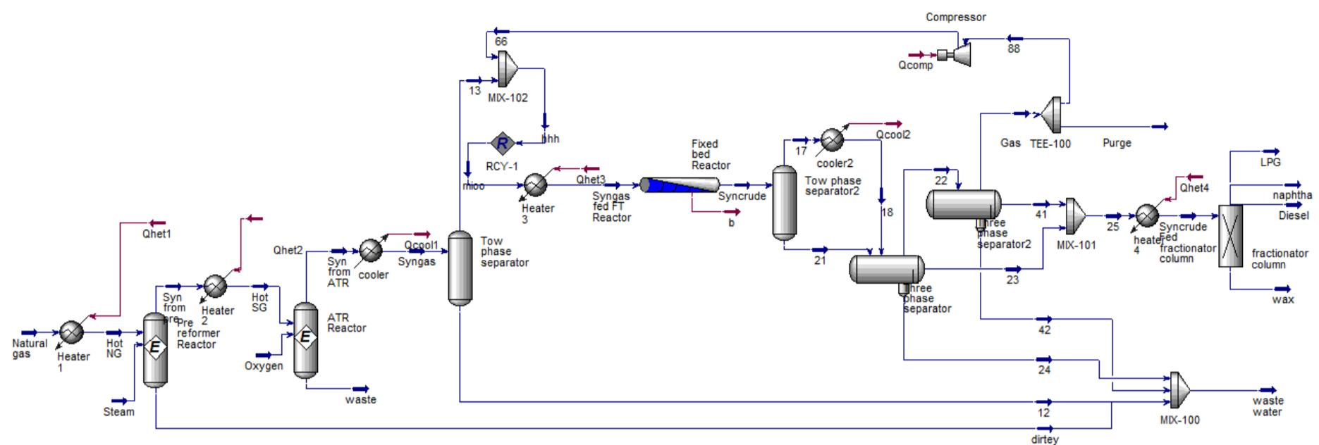
Figure 9.6 HYSYS simulation flow sheet
