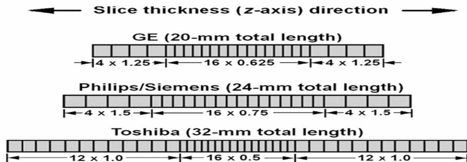
Figure: 2.3 Diagrams of various 16-slices detector designs (in z-direction). Innermost elements can be used to collect 16 thin slices or linked in pairs to collect 16 thicker slices [D.Tack 2007].
