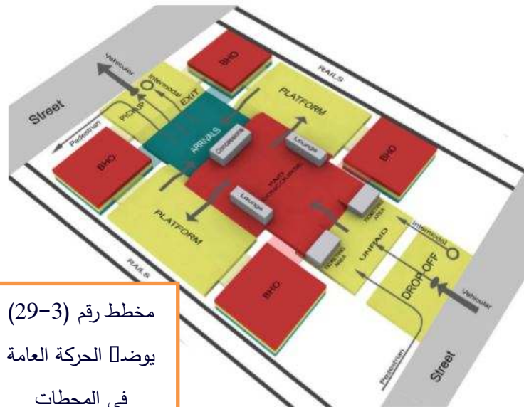
Fig. 1 of 4.5.3: Schematic diagram showing Passenger Circulation Flow within the Station
