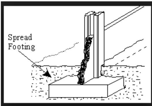
FIGURE 4-14 STRUCTURAL DETAIL
