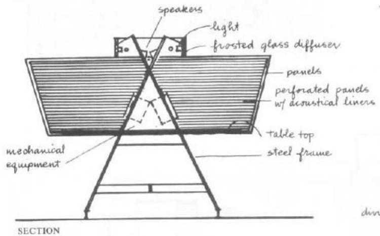
FIGURE 3-15 Closed carrels for sound and visual equipment:
