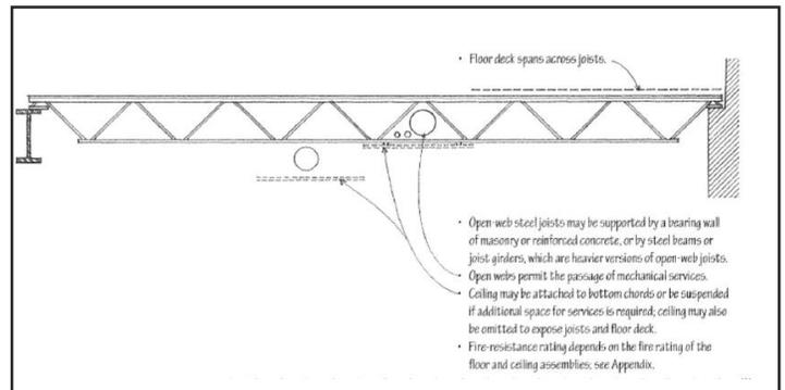
FIGURE 4-13 STRUCTURAL DETAIL
