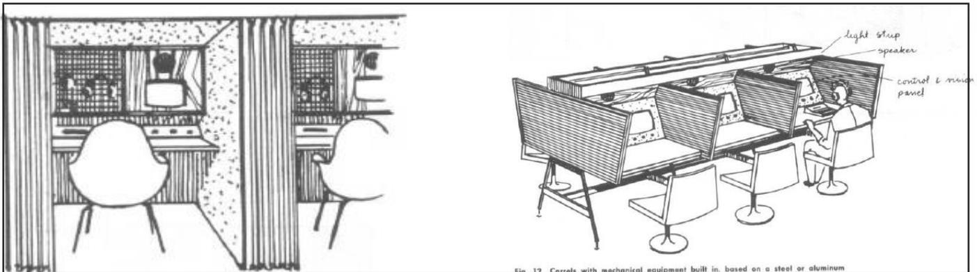
Fig. 13 Carrels with mechanical equipment built in, based on a steel or aluminum "X" frame. Frame folds up like a card table, can be used for other purposes as well.
