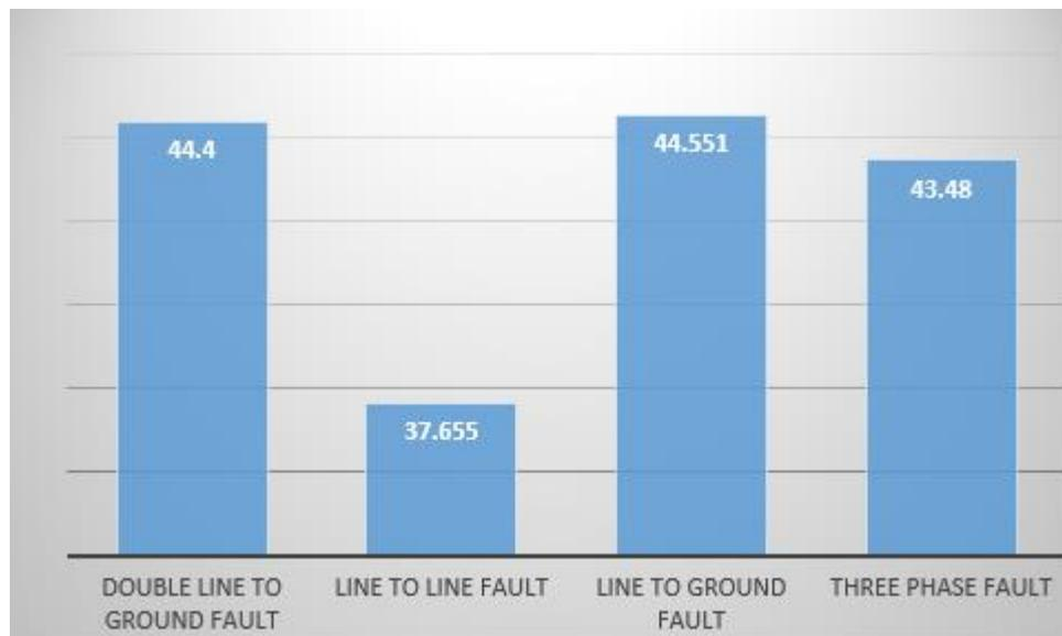
Figure 4.15: Comparison between different short circuit current at 11kv at parallel operation (2)
