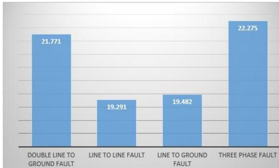
Figure 4.18: Comparison between different short circuit current at 0.415kv at parallel operation (2)
