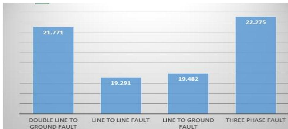
Figure 4.13: Comparison between different short circuit current at 0.415kv at parallel operation (1)
