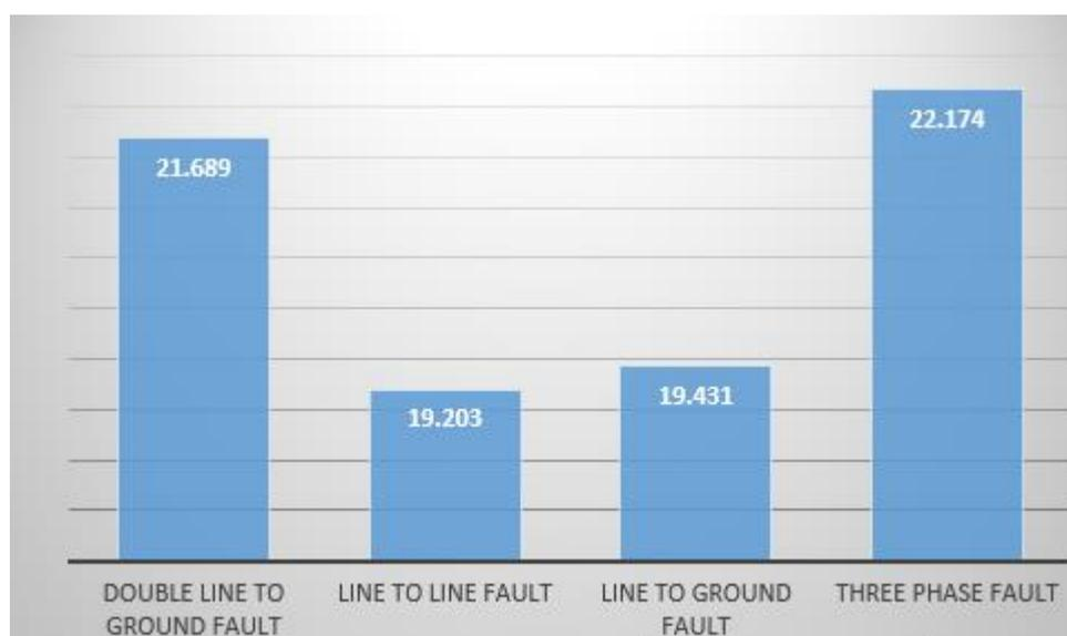
Figure 4.8: Comparison between different short circuit current at 0.415kv
