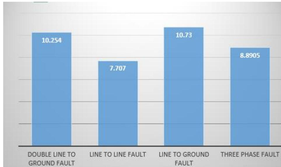
Figure 4.7: Comparison between different short circuit current at 110kv
