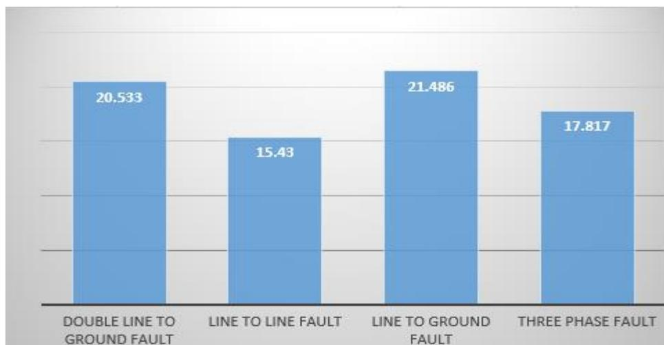
Figure 4.17: Comparison between different short circuit current at 110kv at parallel operation (2)
