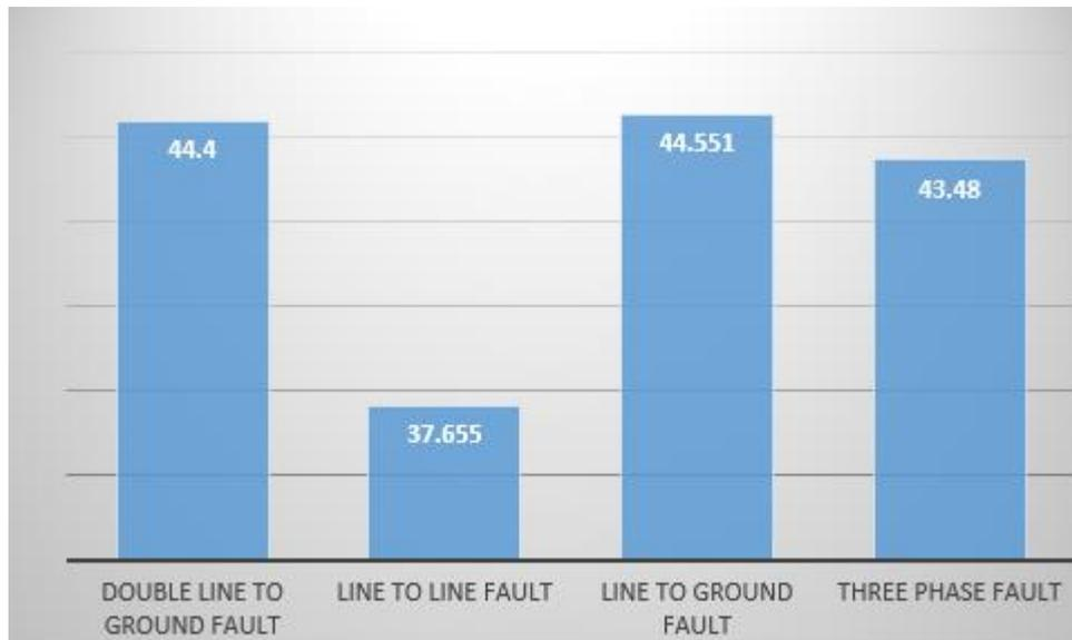
Figure 4.10: Comparison between different short circuit current at 11kv at parallel operation (1)
