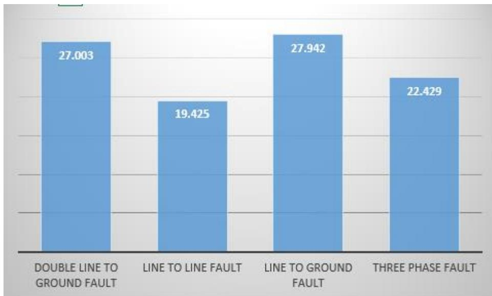
Figure 4.6: Comparison between different short circuit current at 33kv
