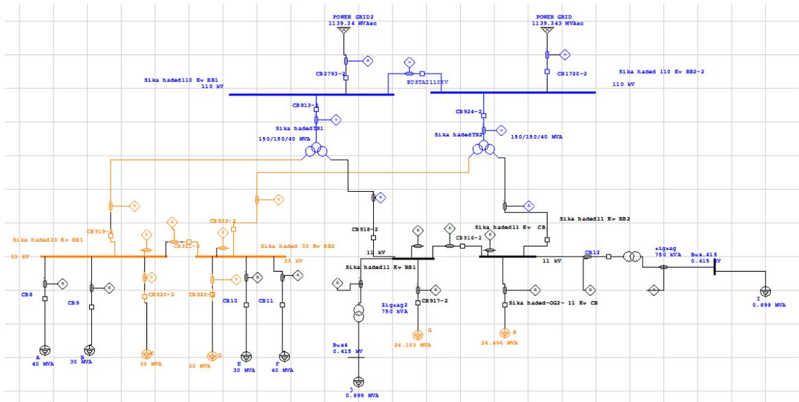
Figure 4.14: Substation at parallel (2) operation
