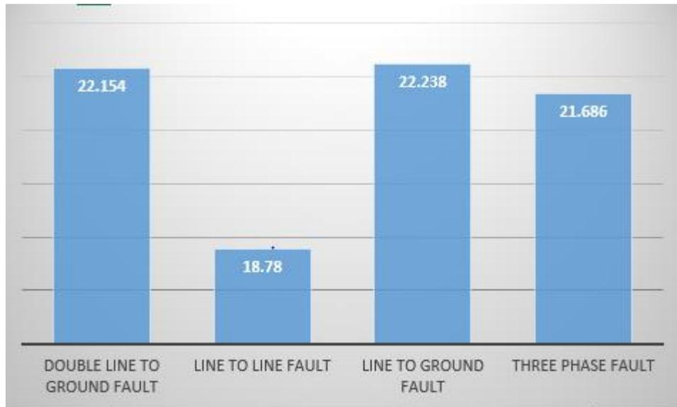
Figure 4.5: Comparison between different short circuit current at 11kv
