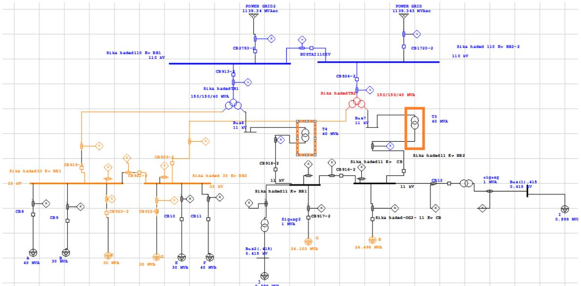
figure 4.19: Adding zigzag transformer to measure line to ground fault
