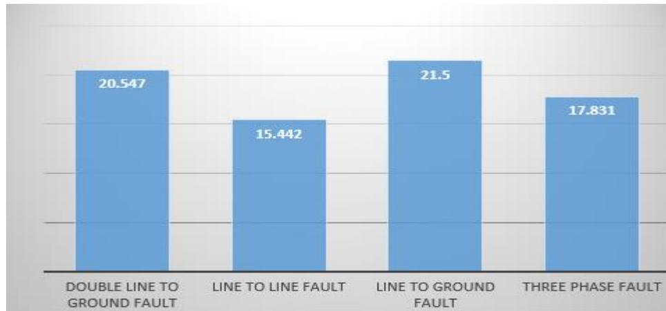
Figure 4.12: Comparison between different short circuit current at 110kv at parallel operation (1)
