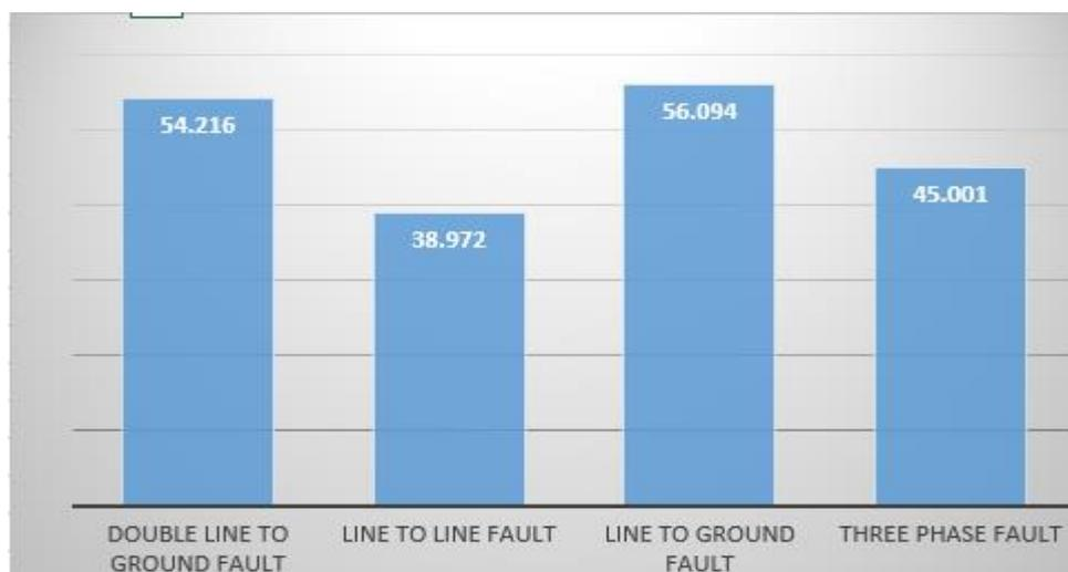
Figure 4.11: Comparison between different short circuit current at 33kv at parallel operation (1)
