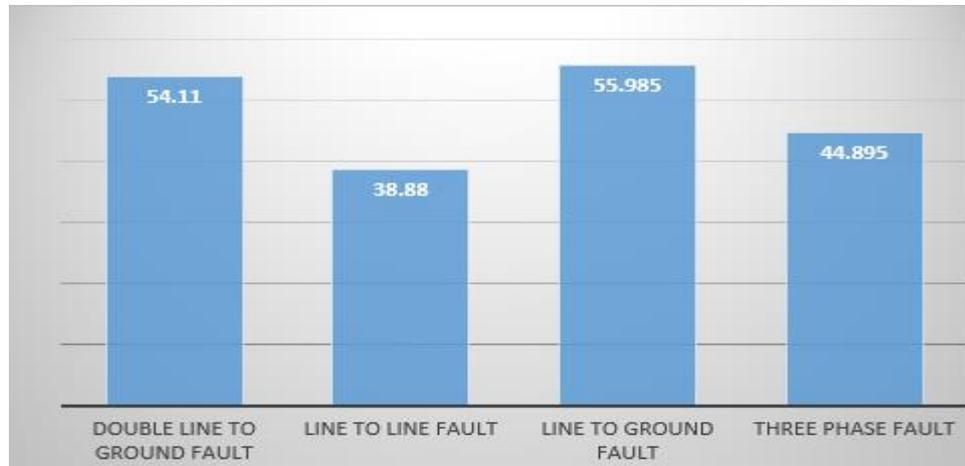
Figure 4.16: Comparison between different short circuit current at 33kv at parallel operation (2)
