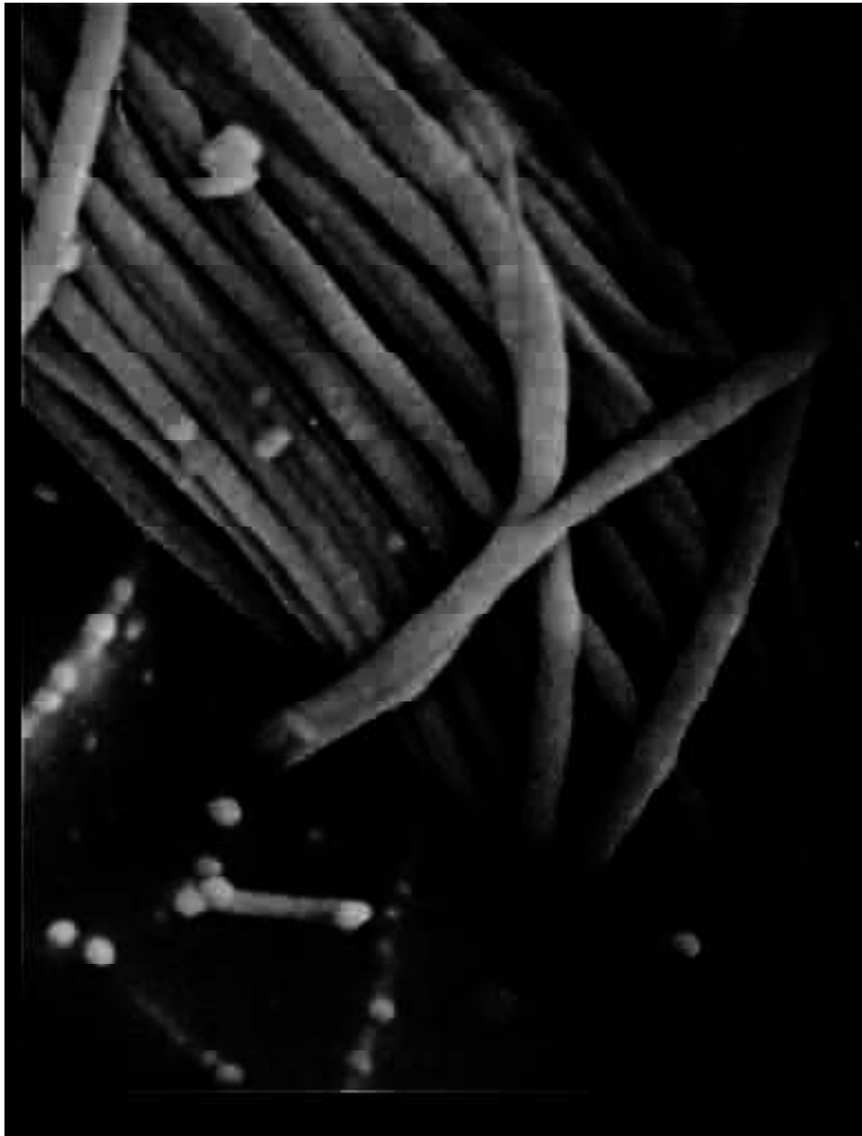
Figure 1.2 Cryo-scanning electron photomicrograph of a wet blue fibril bundle.( A. D. Covington et al,1993)
