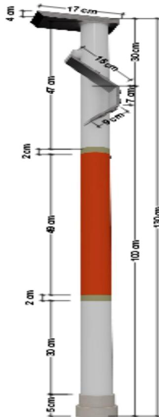
Figure 4.1: Dimension of guide cane
