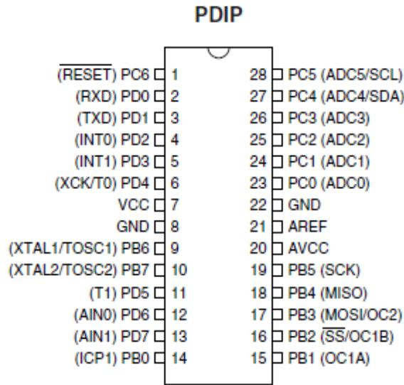
**Figure3.4: AT mega 81 pin configurations**
