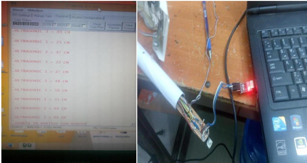
Figure 4.5:HCSR04 sensor distance test
