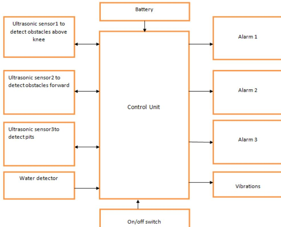
**Figure 3.1: Block diagram of the interactive cane**
