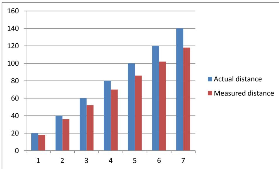
**Figure 4.6: Relationship between actual distance and measured distance.**
