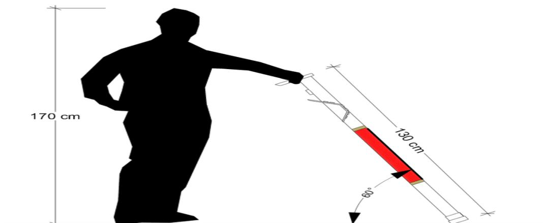
Figure 4.3: Side elevation of guide cane and height of blind person.
