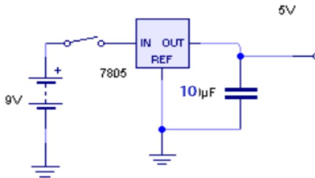
Figure 3.7: The power stage of interactive cane
