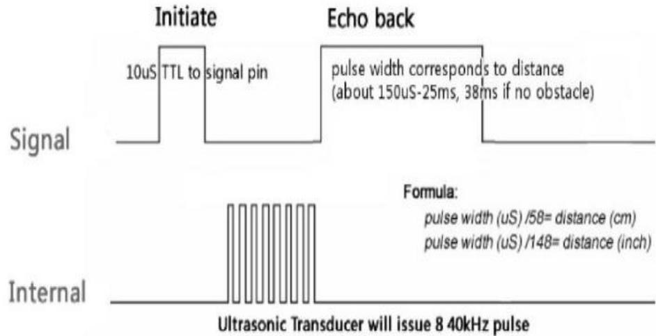
**Figure 3.6: Ultrasonic Trigger and echo pulse**
