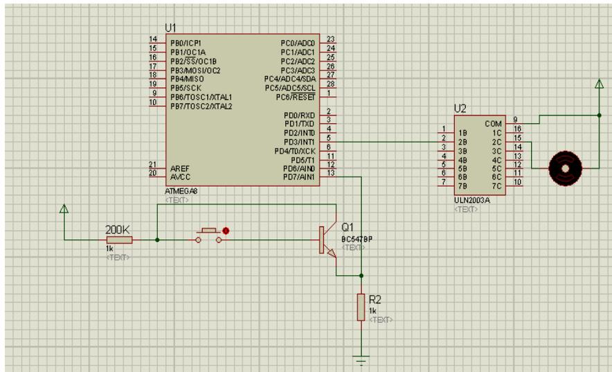
**Figure 3.9: water detector circuit**
