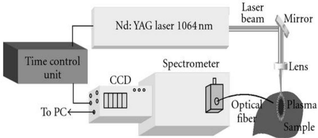
**Figure (1.4): Typical LIBS set-up** (F. Anabitarate et al, 2012).
