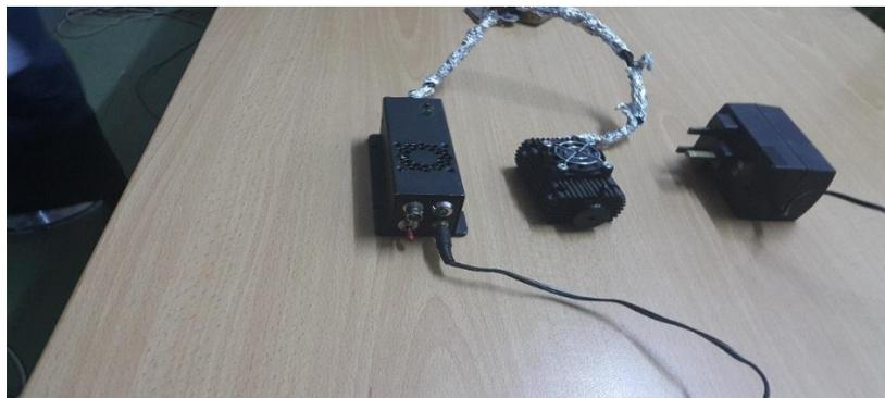
**Figure (2.6): The green diode laser (532nm).**
