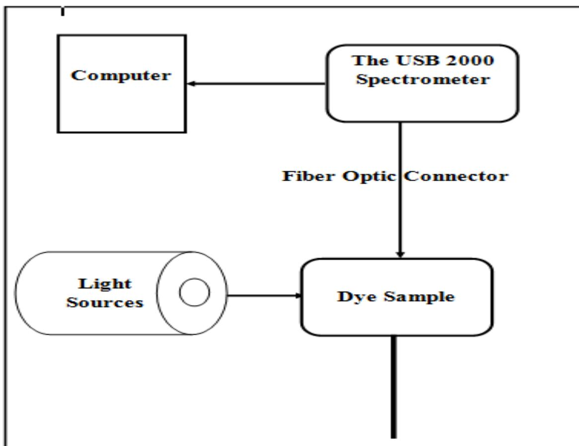
**Figure(2.8):The arrangement of the experimental setup**
