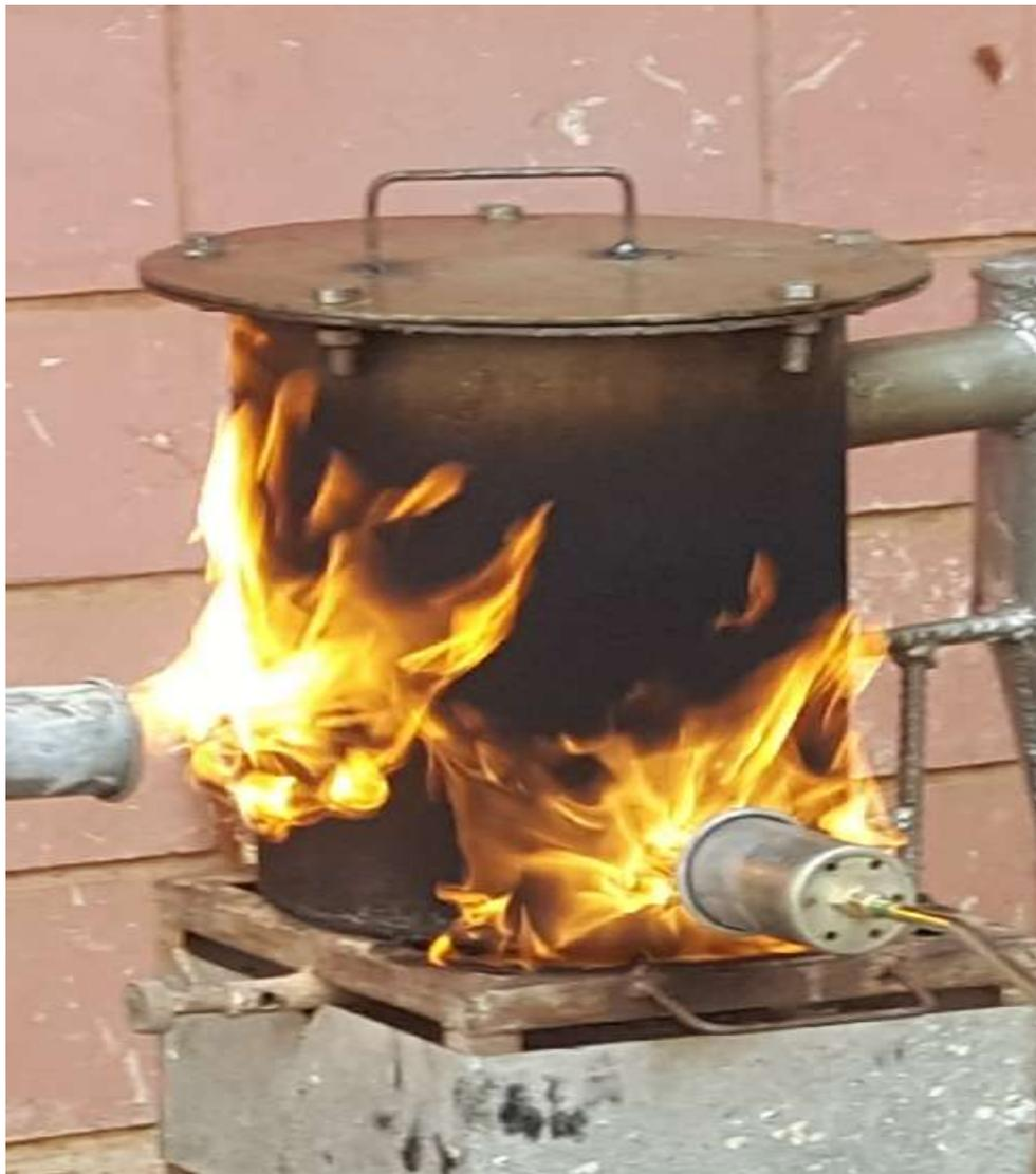
**Figure (3.2) Pyrolysis Reactor**
