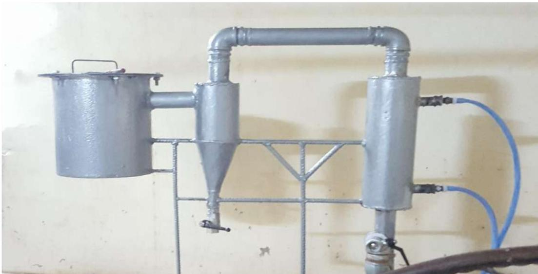
**Figure (4.1) Testing rig for slow pyrolysis of sugarcane bagasse**
