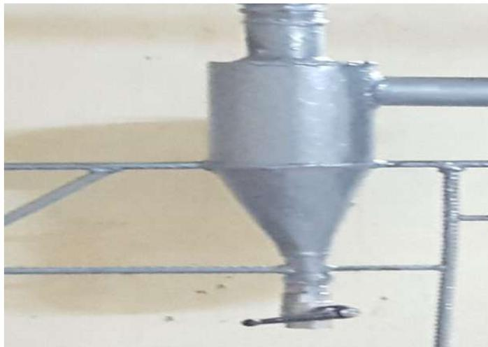
Figure (3.5) cyclone separator
