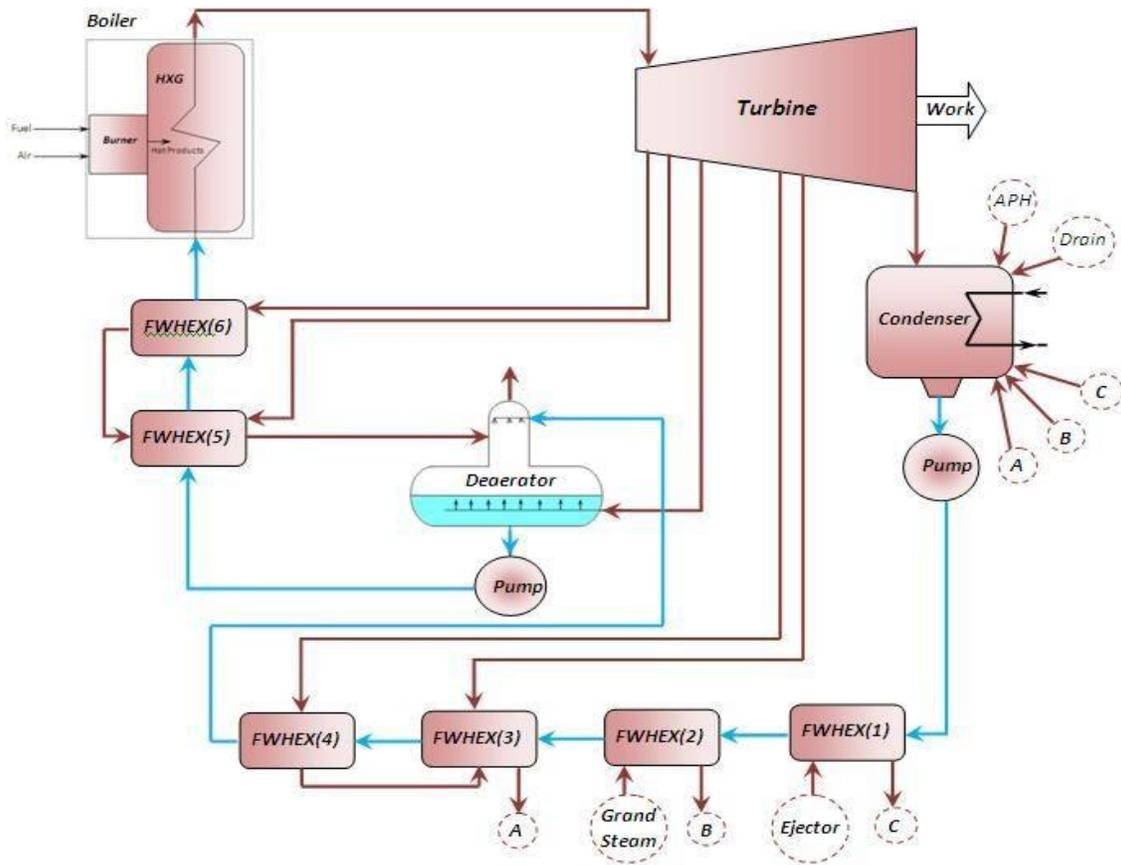
Figure 3.4 The schematic diagram of {KNPSP(6)}
