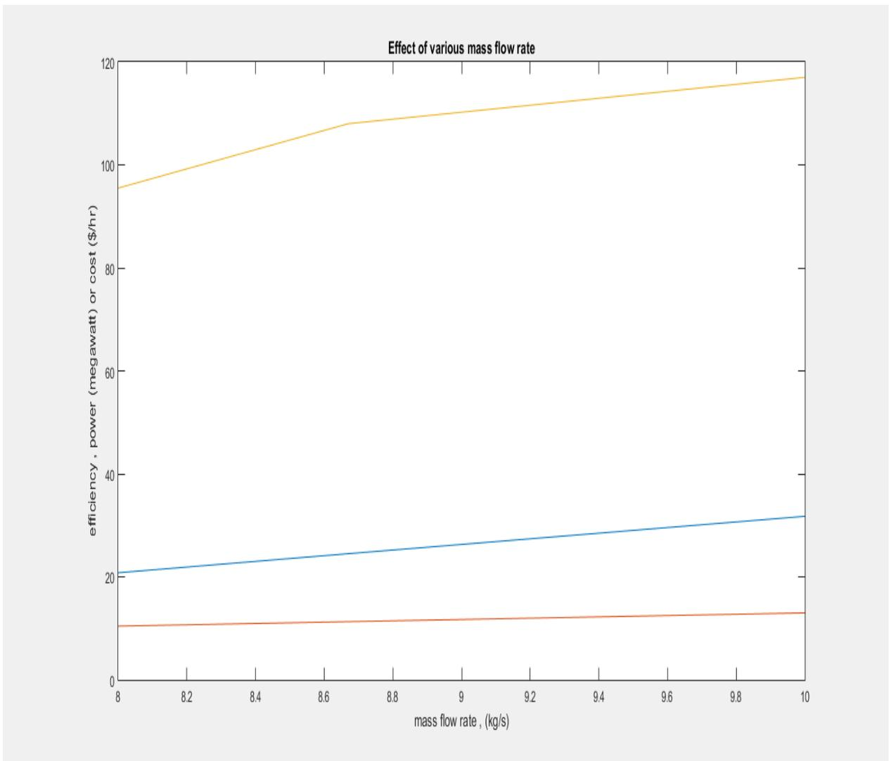
Figure (4.1): The effect of mass flow rate at (efficiency, load and fuel cost)
