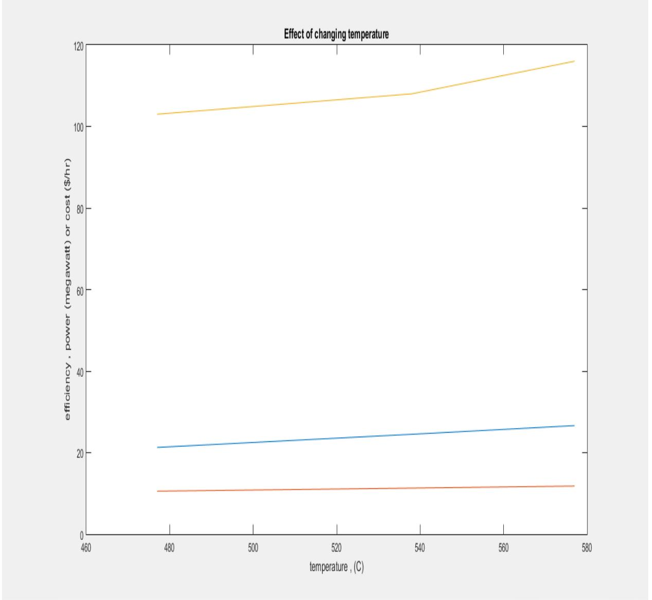
Figure (4.2): The effect of temperature of the boiler
