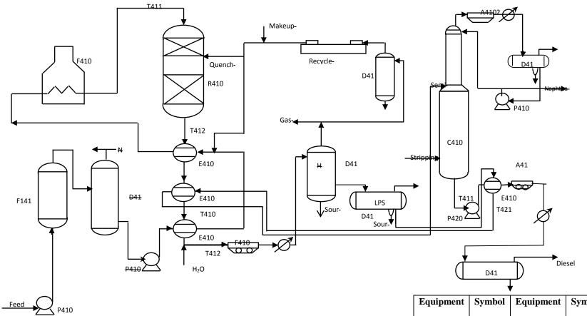
Figure (3.1): Flow Chart of Diesel Hydrotreating unit
