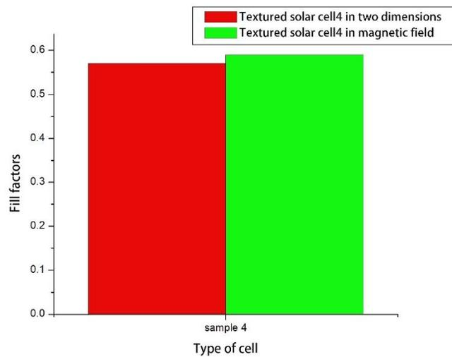
**Fig (4.17): chart shows the changes of fill factors for texturedcell<sub>4</sub>and after operated in magnetic field.**
