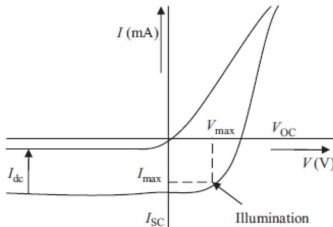
**Fig (2.4): I–V characteristics of a solar cell with and without illumination.**
