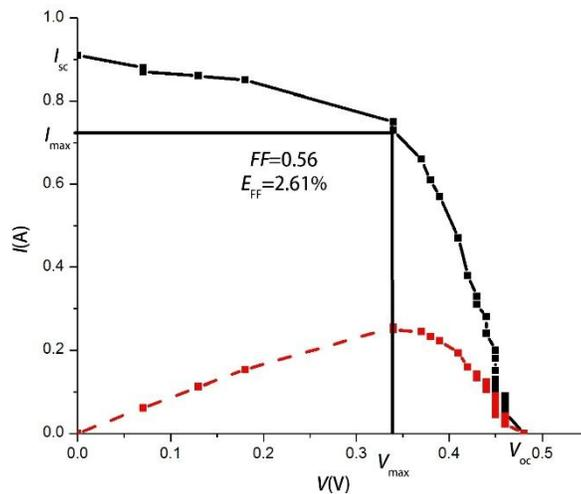
Fig (4.8) shows the I-V Curve Characteristics of solar cell<sub>2</sub>in horizontal magnetic field.
