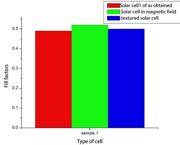
**Fig (4.5) chart shows the changes of fill factors for cell<sub>1</sub> of as obtained and after operated in vertical magnetic field and finally textured.**
