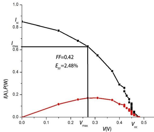
**Fig (4.11): plot of the I-V Curve characteristics of the textured solar cell<sub>3</sub> in one dimension.**
