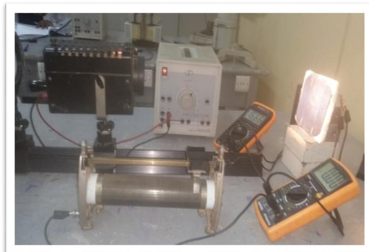
Fig (3.9): setup arrangement to measure I-V characteristics of textured solar cell.
