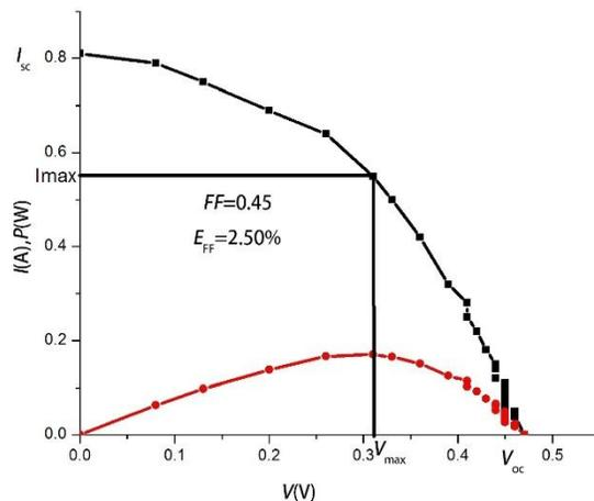
Fig (4.12): shows the I-V curve characteristics of the textured solar cell<sub>3</sub> in magnetic field.
