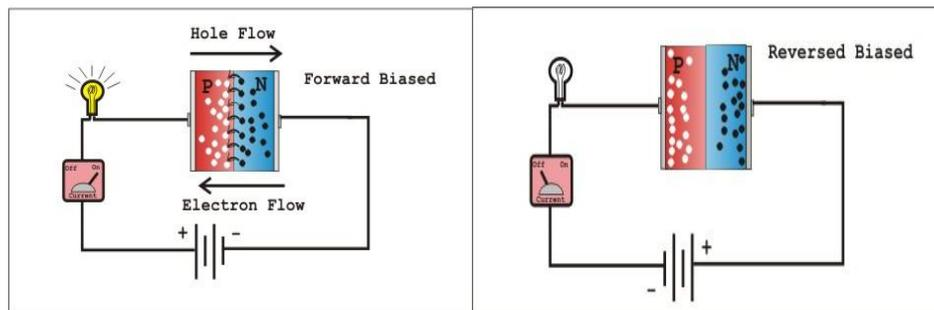
**Fig (2.2): forward biased & reversed biased in diode.**
