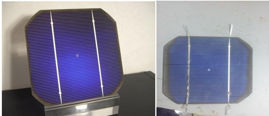
**Fig (3.1): 125x125 mono-crystalline solar cells**
