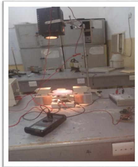
Fig (3.8): setup arrangement to measure I-V characteristics of solar cell in magnetic field.
