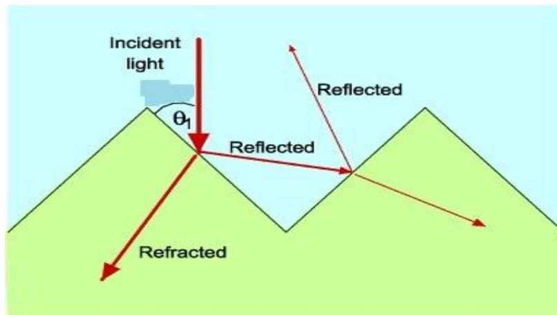
**Fig (2.6): Reflection and transmission of light for a textured silicon solar cell.**
