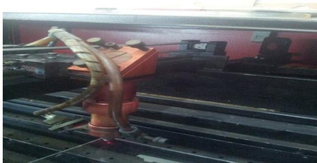
**Fig (3.3): Technique of deliver laser beam to working area by mirrors.**
