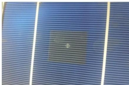
**Fig (4.3):** textured area on the cell<sub>1</sub> in one dimension.
