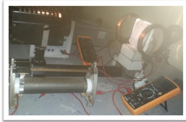
Fig (3.10): setup arrangement to measure I-V characteristics of textured solar cell in magnetic field.
