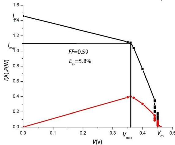
Fig (4.16): shows the I-V curve characteristics of the textured solar cell<sub>3</sub> in magnetic field.
