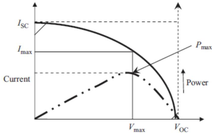
**Fig (2.5): Characteristic and power curve for determining the fill factor (FF).**
