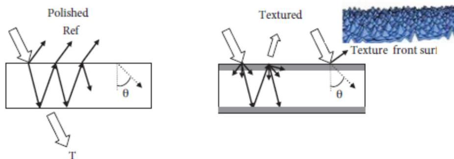
**Fig (1.1): Texturing Surface of Solar cell.**
