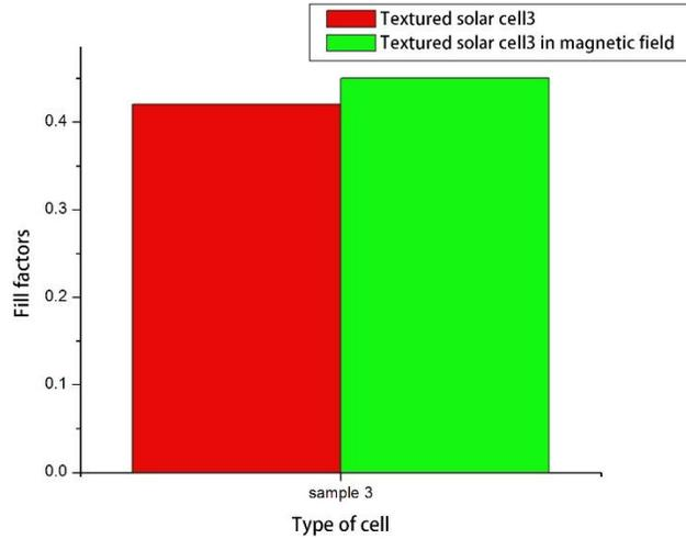
**Fig (4.13):** chart shows the changes of fill factors for texturedcell<sub>3</sub>and after operated in magnetic field.
