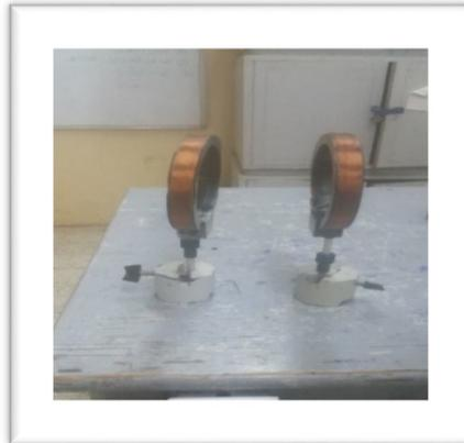
**Fig (3.4): Helmholtz coils used to generate magnetic field.**
