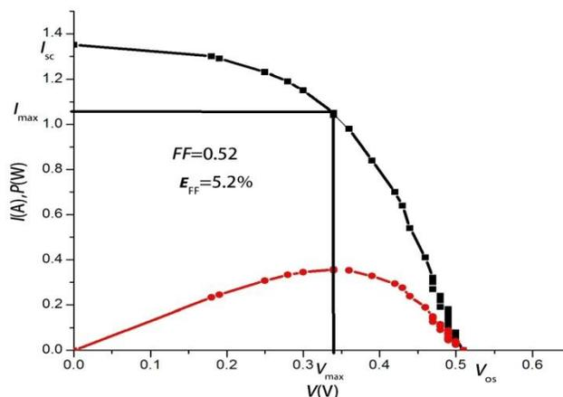
**Fig (4.2):** plot of the I-V characteristics curve of solar cell<sub>1</sub> in vertical magnetic field.
