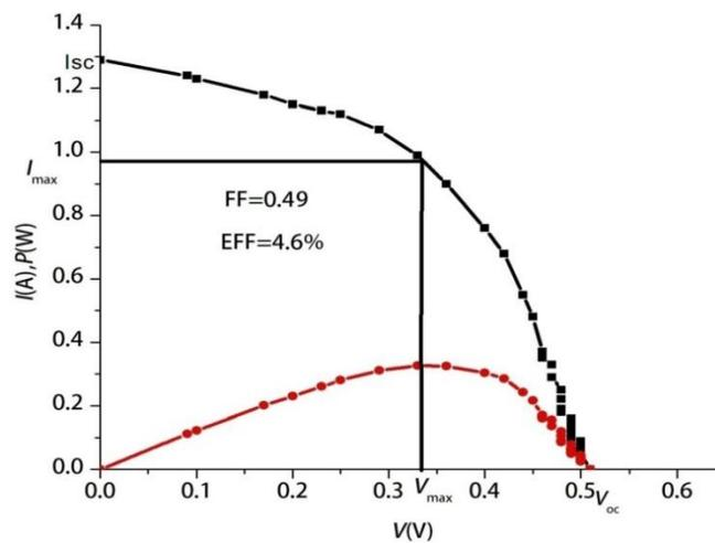
Fig (4.1) plot of the I-V characteristics curve of as obtained solar cell<sub>1</sub>.
