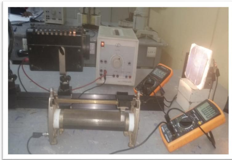
Fig (3.6): setup arrangement to measure I-V characteristics of solar cell.
