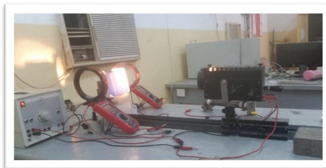
Fig (3.7): setup arrangement to measure I-V characteristic of solar cell in vertical magnetic field.
