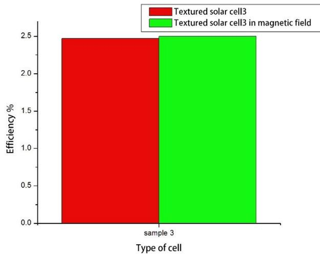
**Fig (4.14):** chart shows the changes of efficiency for texturedcell<sub>3</sub>and after operated in magnetic field.
