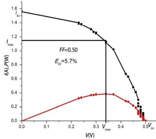
**Fig (4.4) plot of the I-V Characteristics curve of the textured solar cell<sub>1</sub> in one dimension.**
