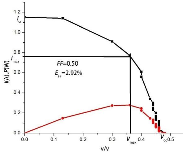
Fig (4.7) plot of the IV Curve characteristics of as obtained solar cell<sub>2</sub>.
