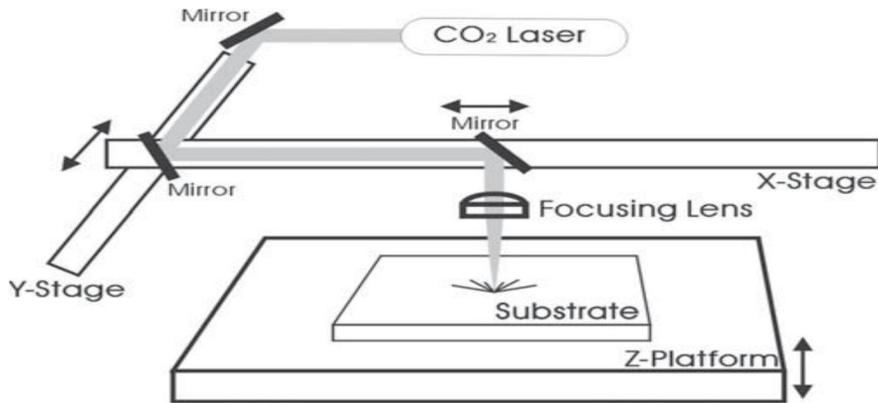
Fig (2.)7: Schematic illustration of a laser direct-write system.
