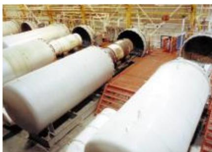
Figure (6.13). A bank of autoclaves used for feeding  $UF_6$  to a plant.
