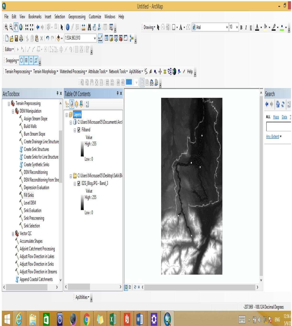
Figure 4-2: Fill Sinks output
