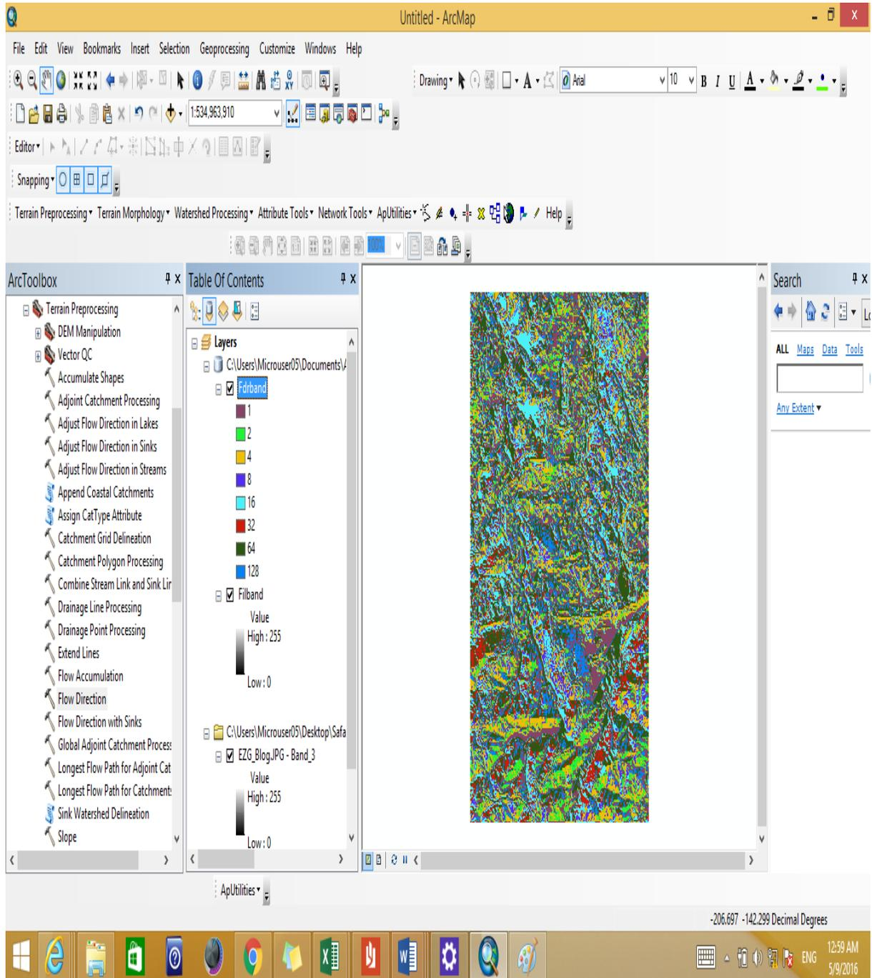
Figure 4-3: Flow Direction output
