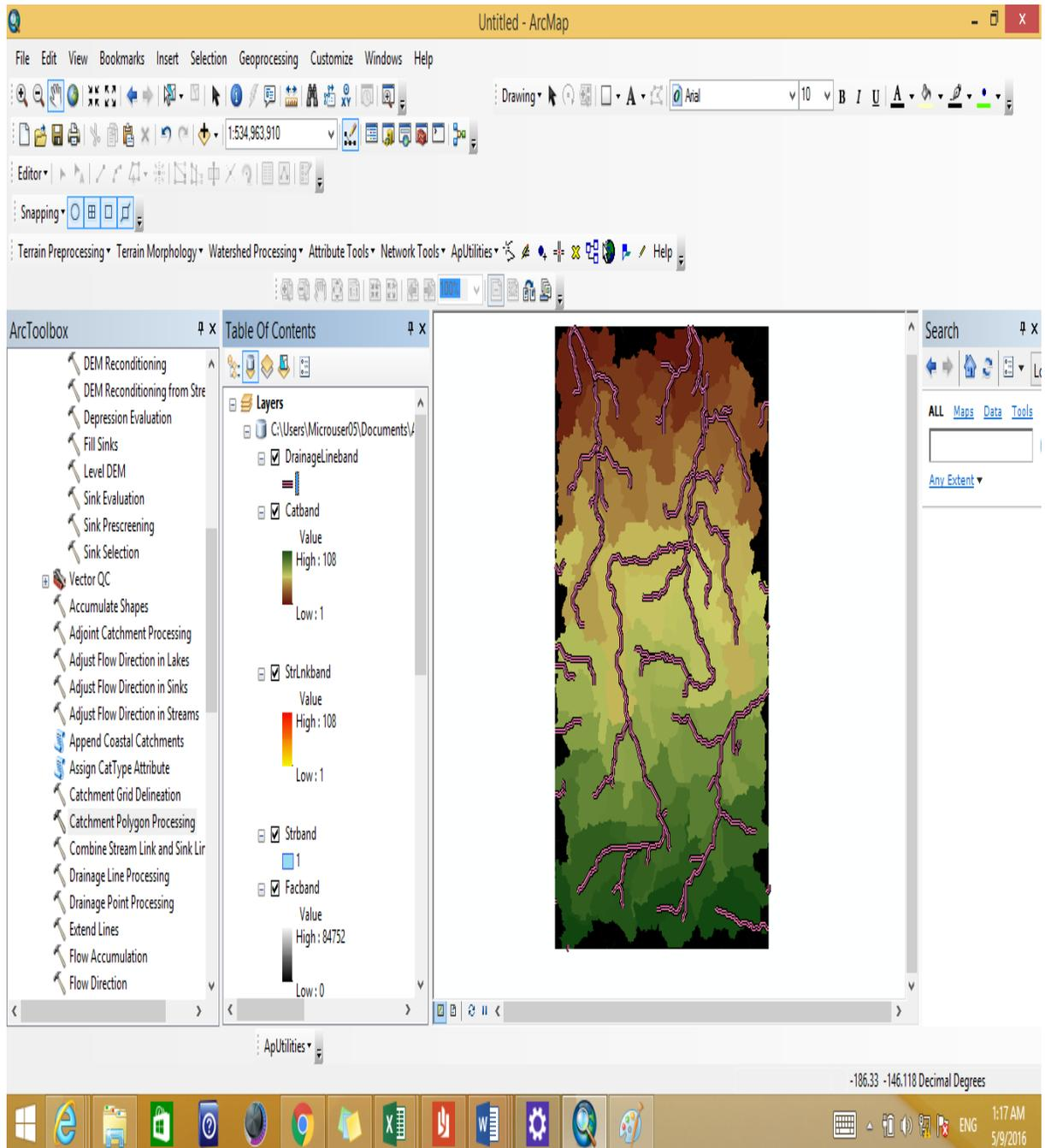
Figure 4-7: Drainage Line Processing output
