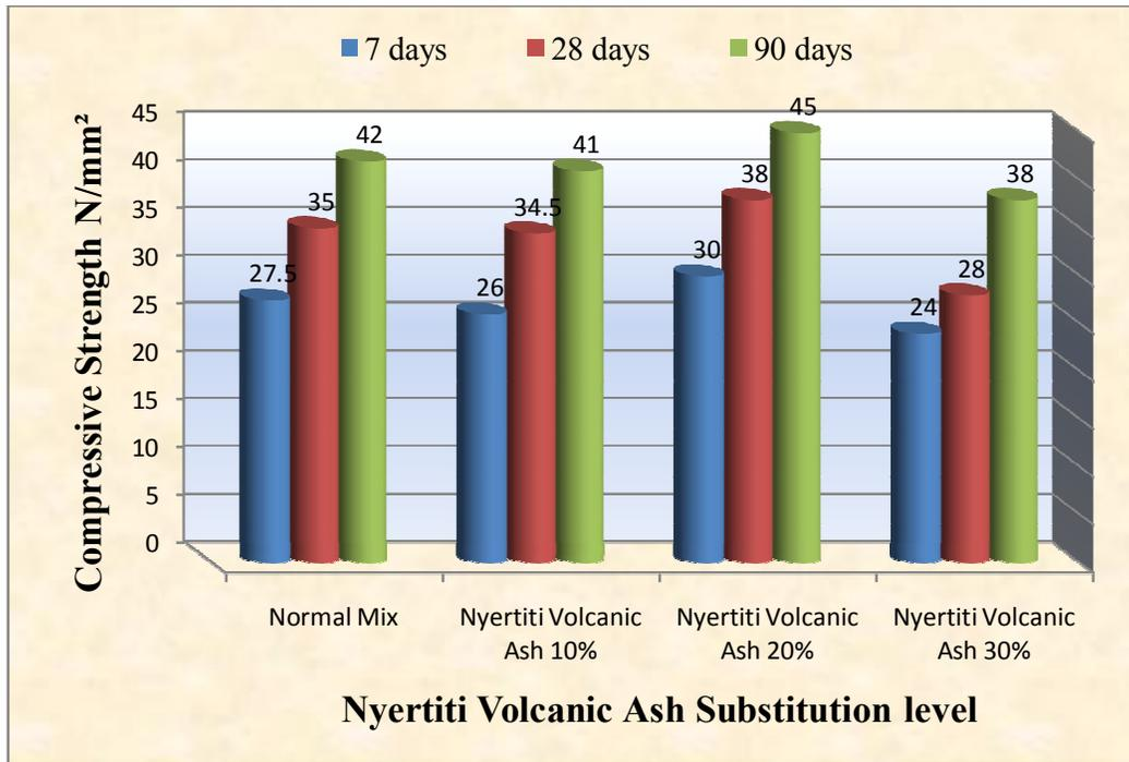
Figure 2. Compressive strength of mixes
