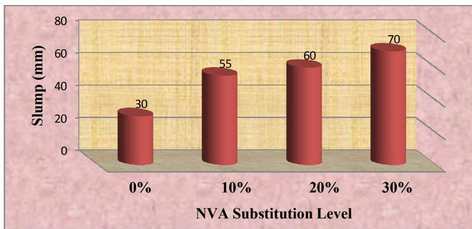
Figure 1. The effect of NVA replacement on workability
