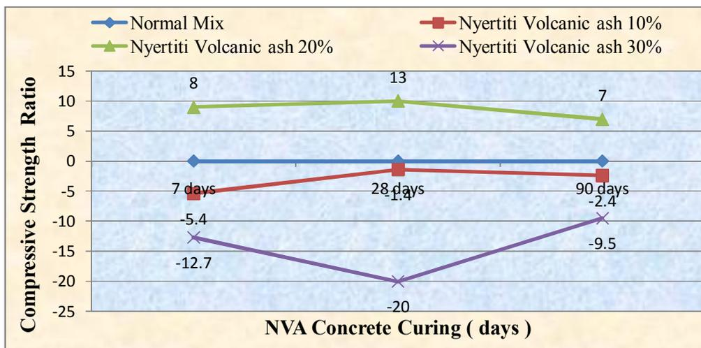
Figure 3. Variation of Relative compressive strength of concrete
