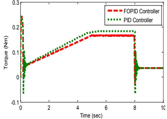
Figure 9: DC motor torque responses under load torque disturbance
