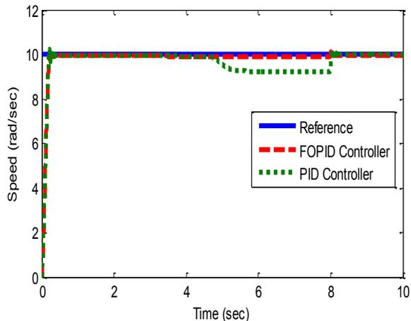
Figure 8: Speed responses of two controllers against sudden change in torque load
