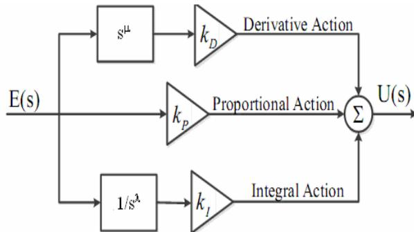
Figure 2: Block diagram of the FOPID controller
