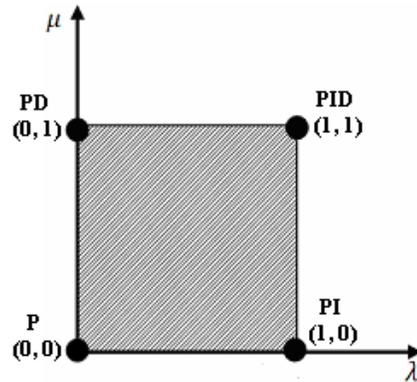
Figure 3: Pictorial representation of the fractional order PID controller
