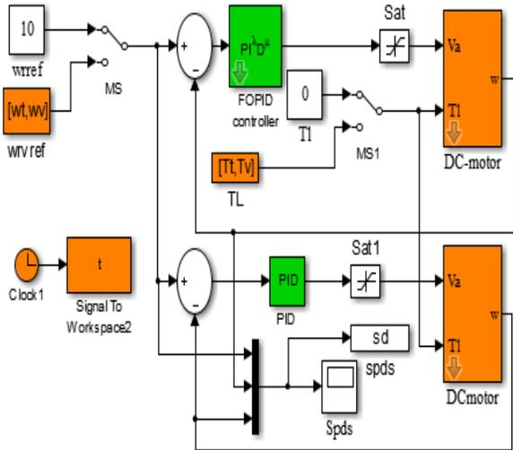
**Figure 4: MATLAB/SIMULINK overall model of speed control of DC motor using FOPID and PID**
