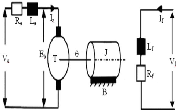
Figure 1: A separately excited DC motor model
