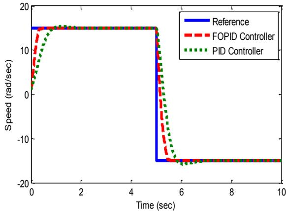
Figure 7: Speed responses of FOPID and ordinary PID controllers with reversing speed
