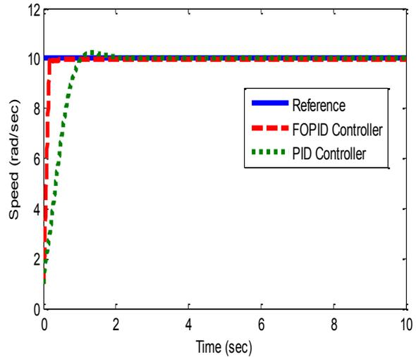
**Figure 5: Step response of SEDC using ordinary PID and FOPID controllers**
