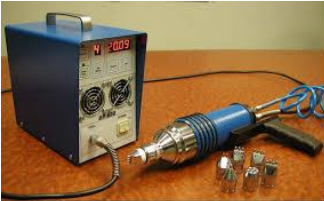
Fig.( 2.7): Basic UP-600 system for fatigue life improvement of parts elements
