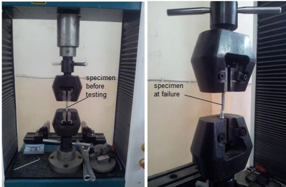
Fig.(3.6): Tensile test machine WDW-200E with tensile specimen during the test
