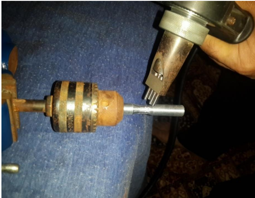
Fig.(3.21):Specimen of 2017A-T3 under UP work
