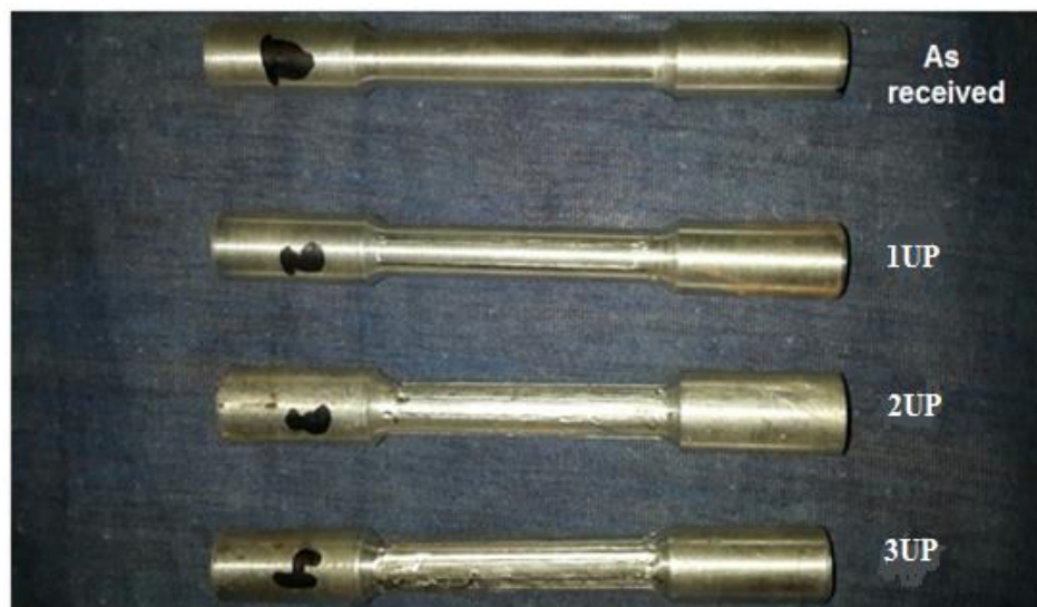
Fig.(3.18); A number of post treatment operation on tensile specimens under UP
