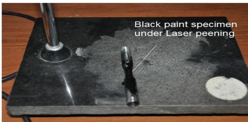
Fig.(3.13): Specimen under black paint laser peening (BLP)
