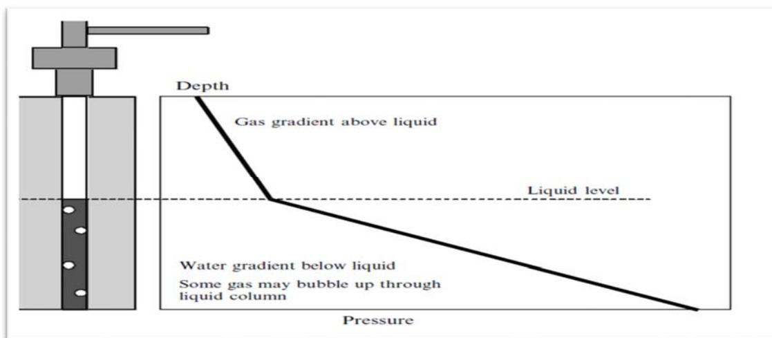
Figure 1.3: Pressure Survey Schematic to determine Liquid Loading (James et al. 2003:20).
