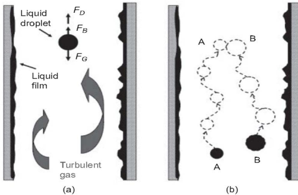
Figure 2.3 Encountering two liquid droplets in turbulent gas stream (Zhou & Yuan 2010:175)
