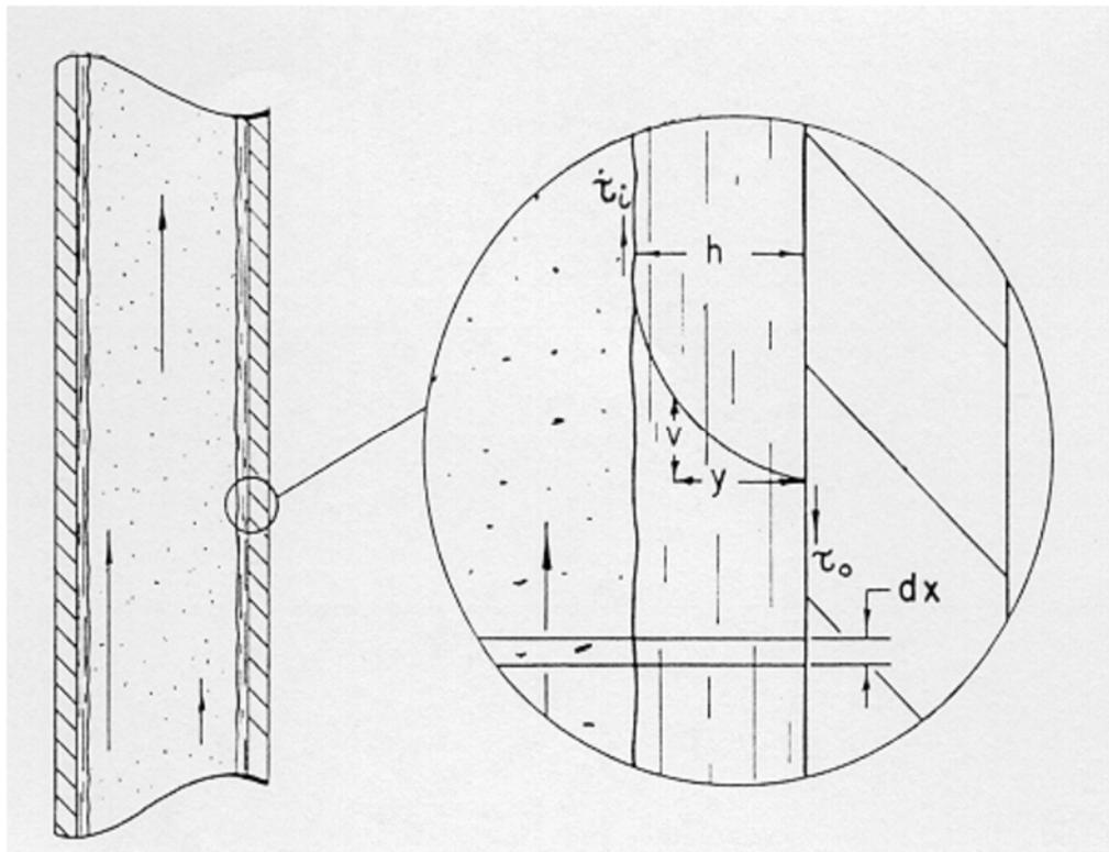
Figure 2.5 Liquid Film movement (Turner et al. 1969:1482)
