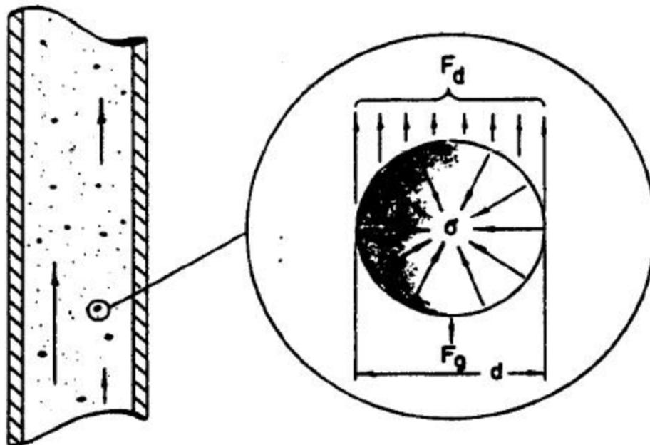
Figure 2.6 Liquid Droplet Movement (Turner et al. 1969:1477)
