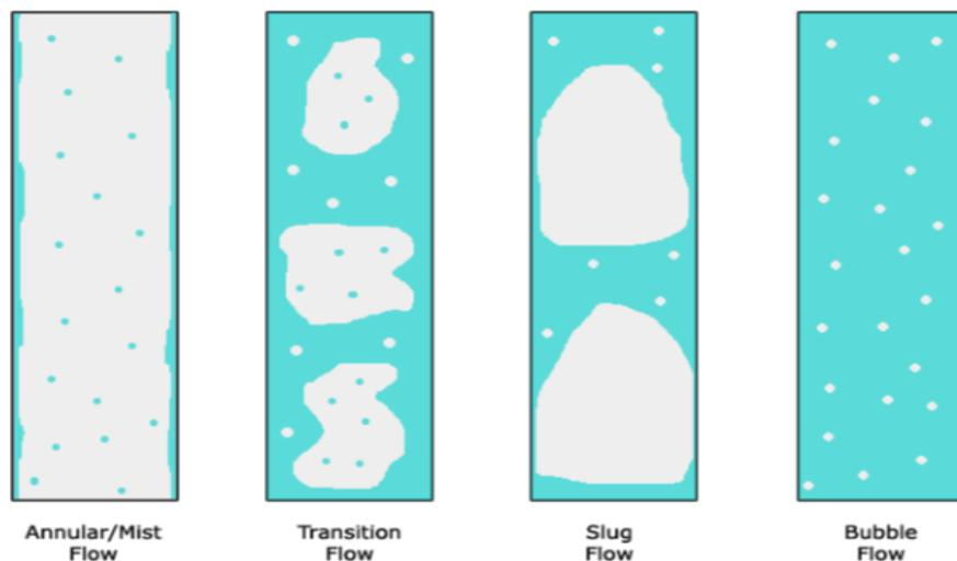
Figure 1.1 Basic profile of Multiphase flow in the well.
