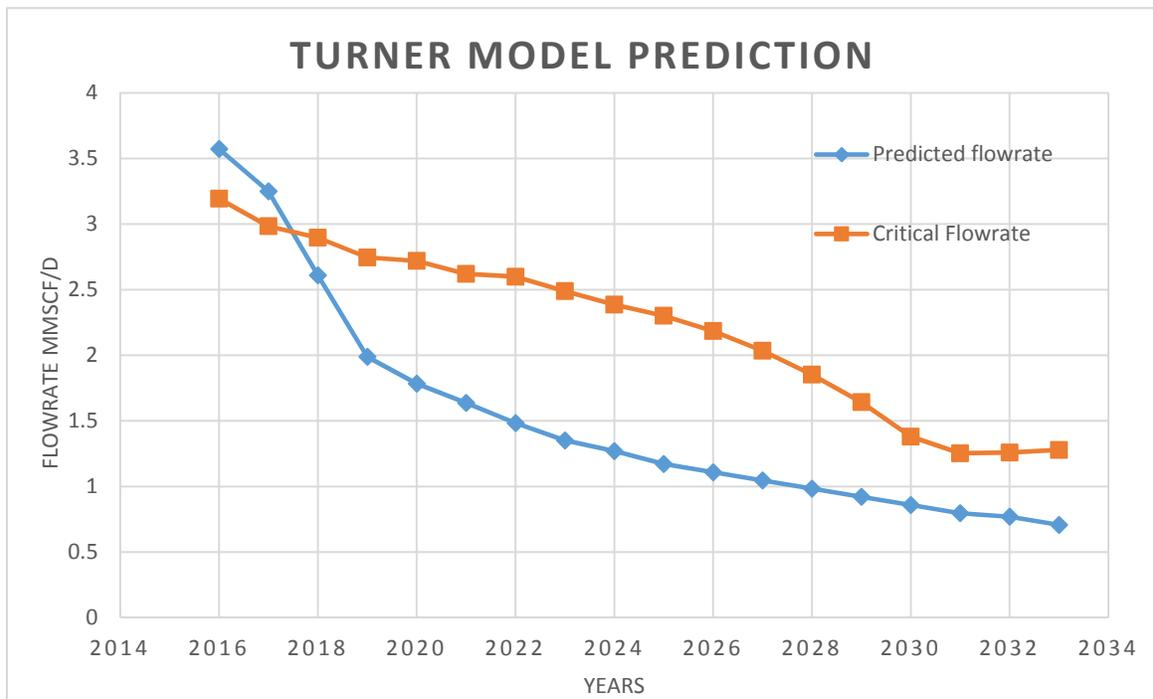
Figure 4.1 Turner Model Prediction loading
