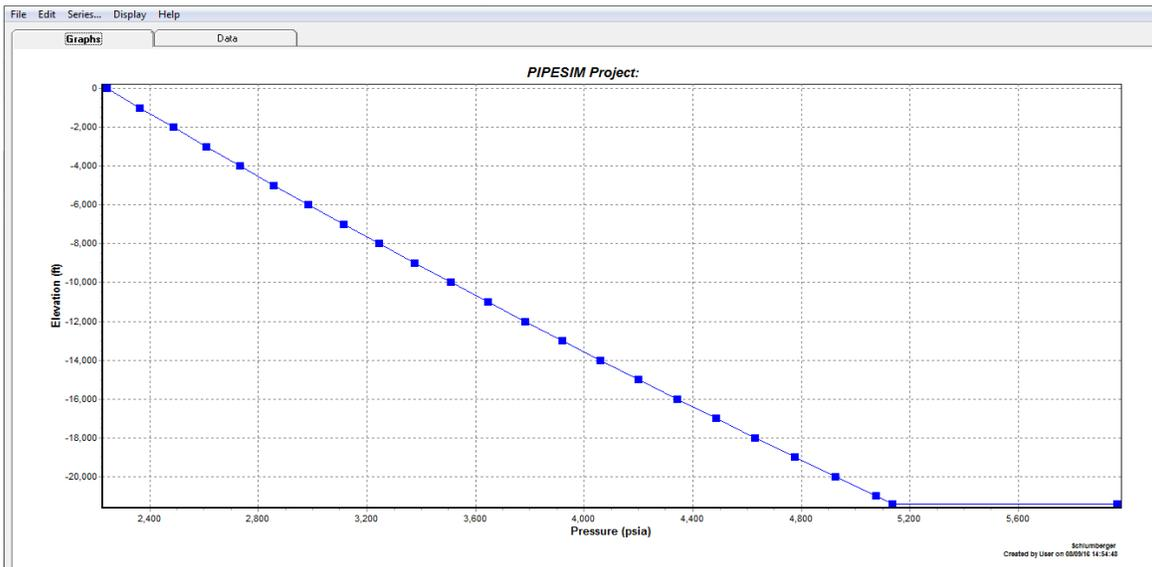
Figure 3.6 pressure distribution along the well
