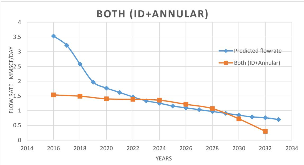
Figure 4.7 Flow rates From Both (Coiled tubing & Annular)
