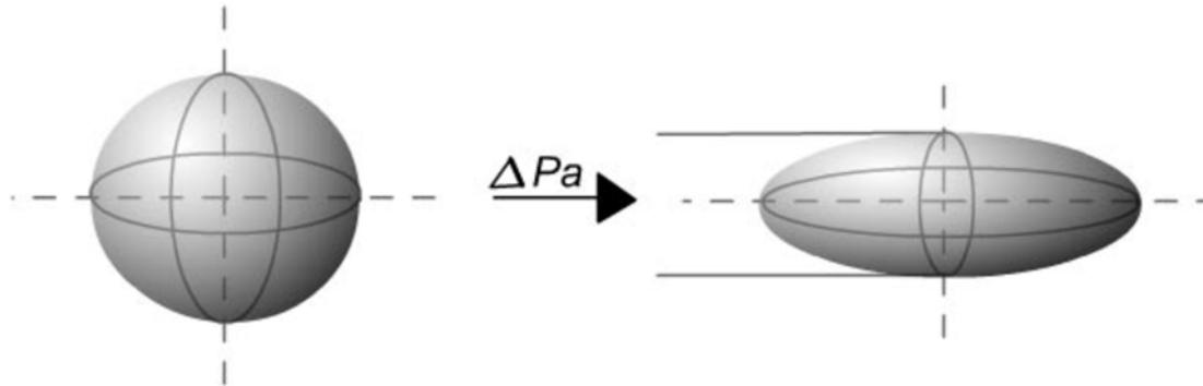
Figure 2.2 Shape of Entrained Drop in a High Velocity Gas
