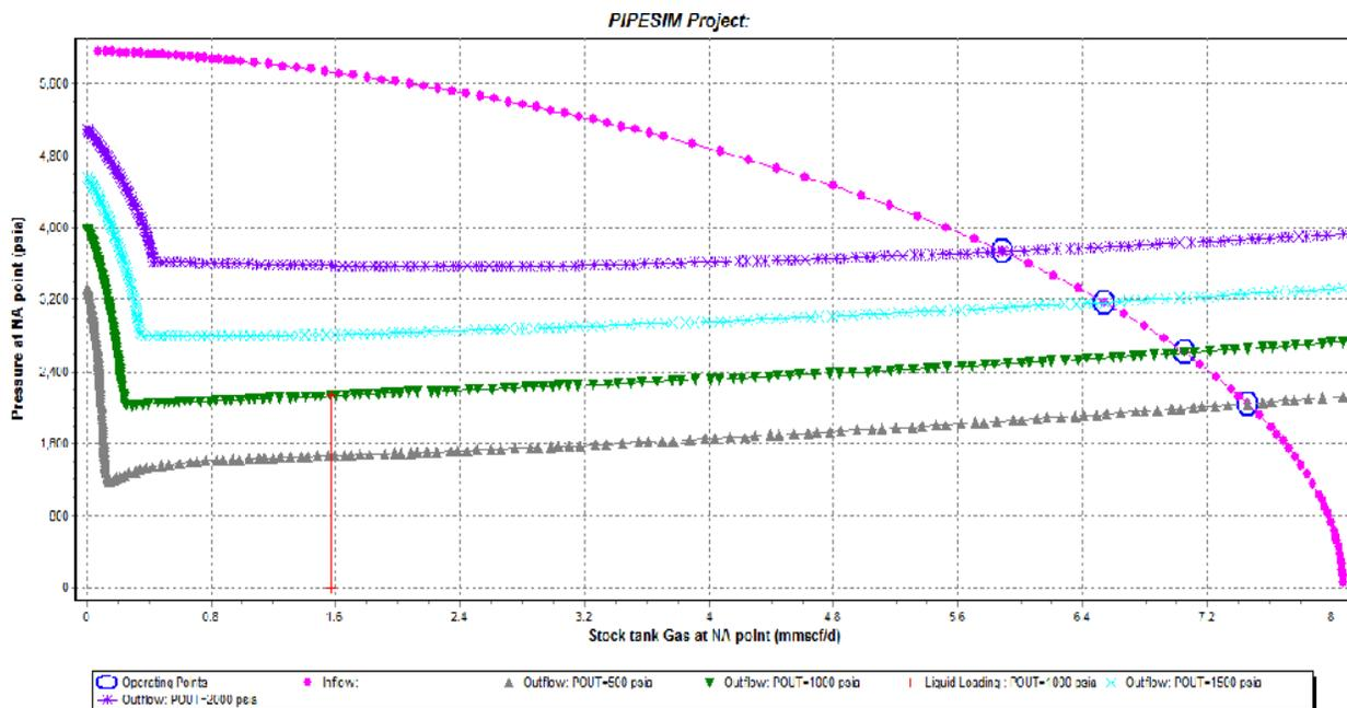
Figure 4.3 Select optimum outlet pressure using PIPESIM software
