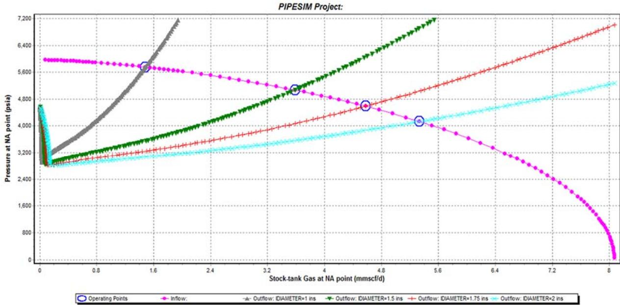
Figure 4.4 Select optimum Coiled tube size
