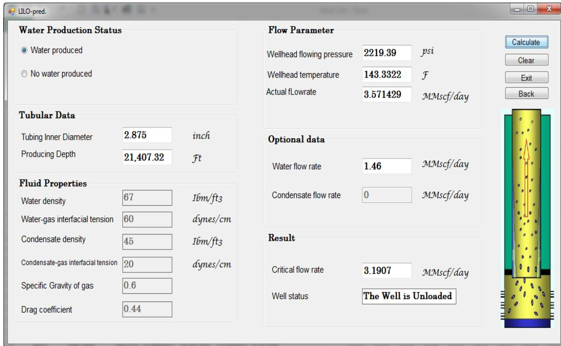
Figure 3.9 Turner et al. Model Input and Result Screen (Our software)
