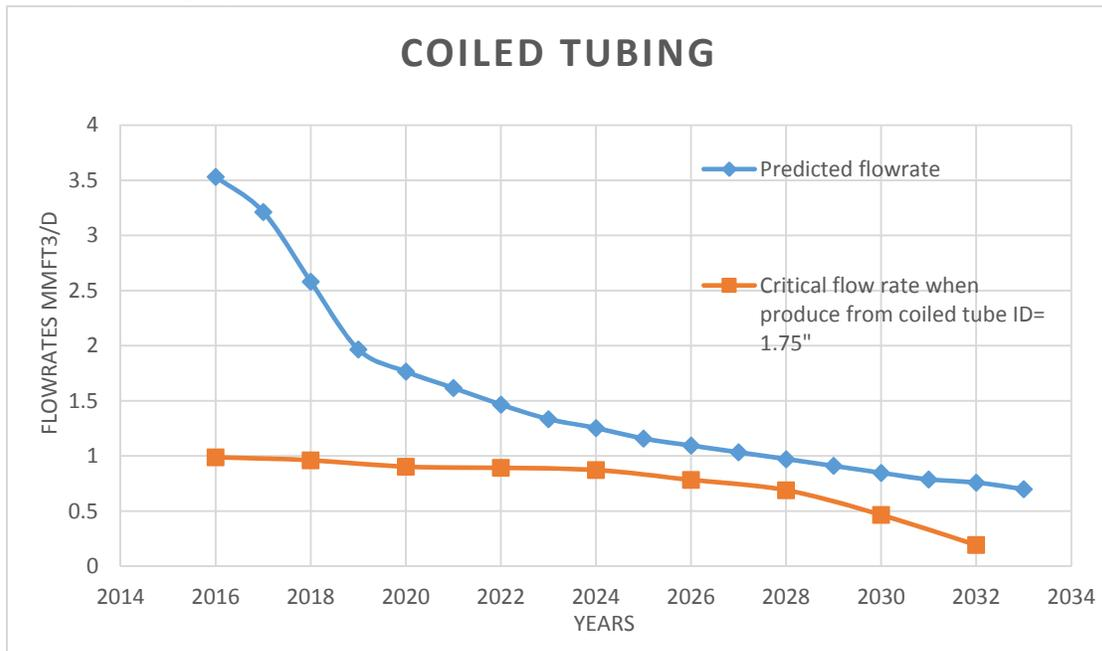
Figure 4.5 Flow rates inside Coiled Tubing
