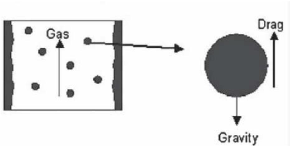
Figure 2.1 the concept of gas velocity at ‘critical’ (James et al. 2003:18)
