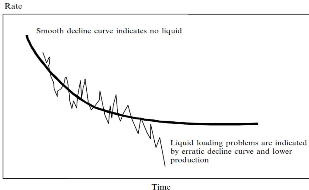
Figure 1.2: Decline Curve as indicator of Liquid Loading (James et al. 2003:18)
