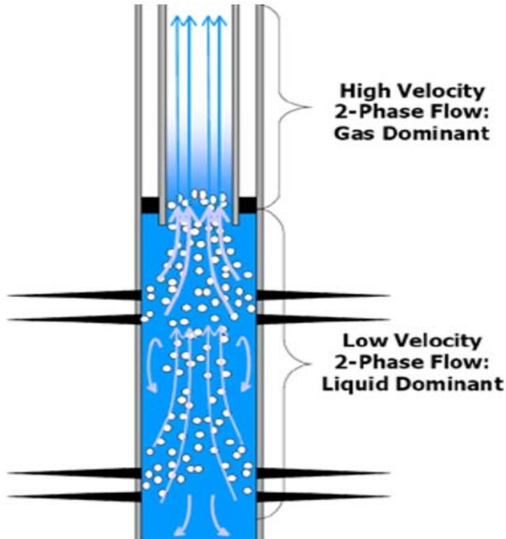
Figure 1.5 Effect of a velocity string on production
