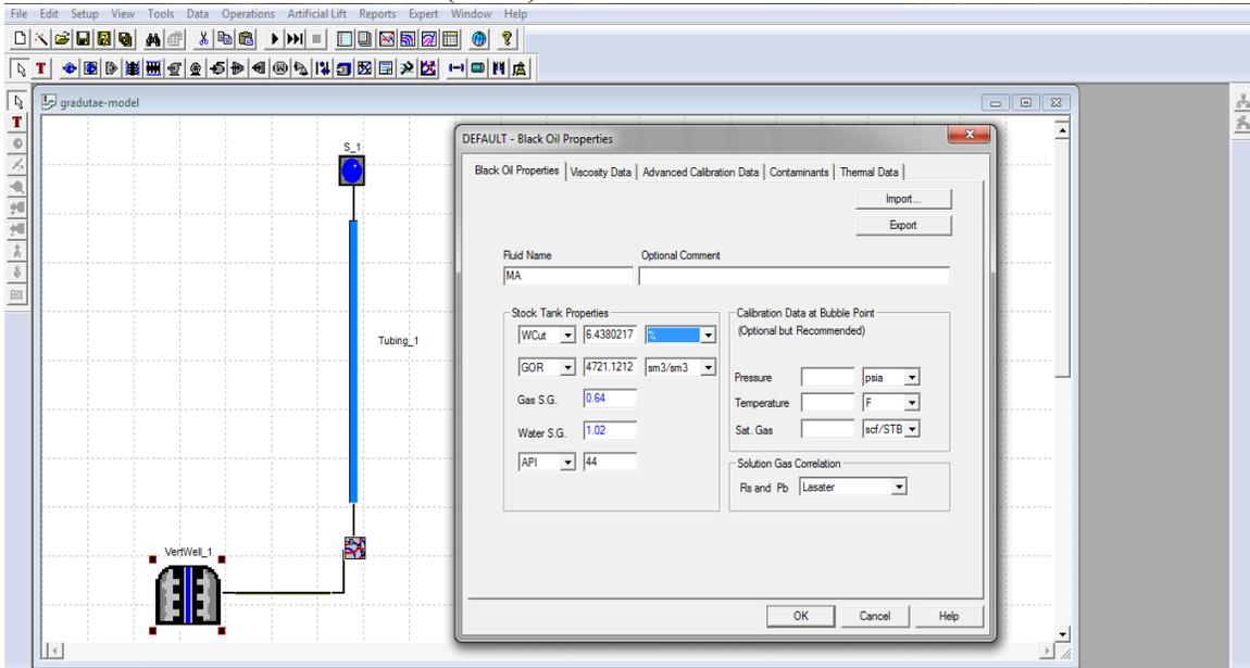
Figure 3.4 Stock tank properties values input
