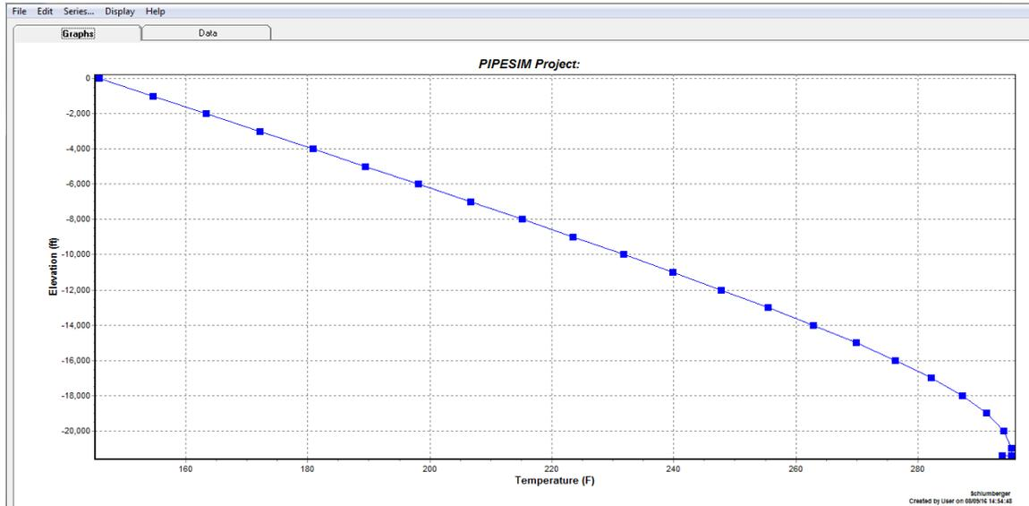
Figure 3.7 temperature distribution along the well
