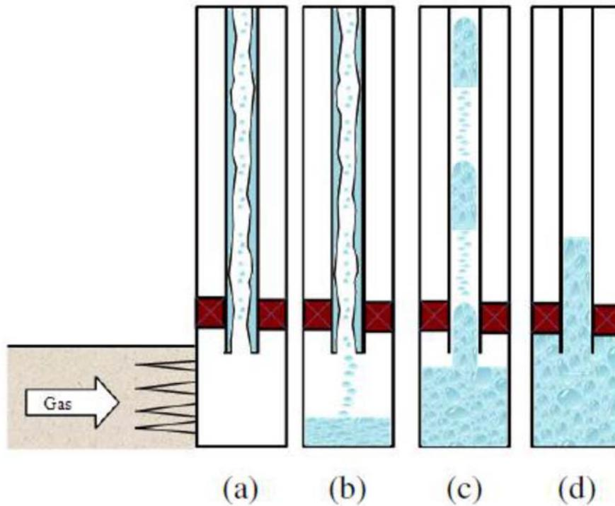
Figure 2.4 Stages of liquid loading process. (a) 1st stage, (b) 2nd stage, (c) 3rd stage and (d) 4th stage
