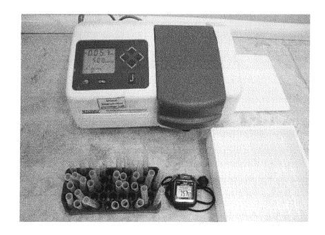
Spectrophotometer machine used for analysis of serum biochemical parameters.
