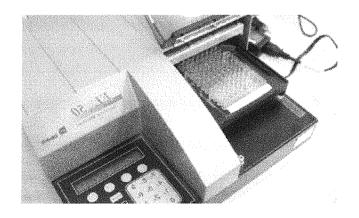
Figure (1) Show ELISA Reader on the left side and ELISA washer on the right side that used for measuring antibodies titers of NDV and IBDV.
