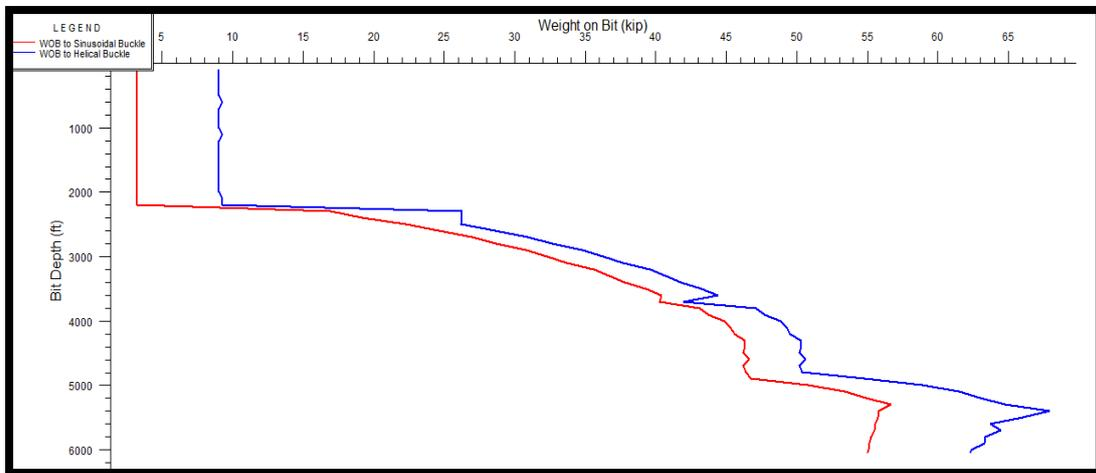
Fig.4.24: 2<sup>nd</sup> Build Section Minimum WOB Chart (Wellplan).
