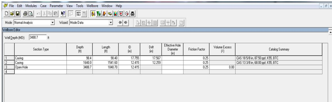
Fig.3.4: 1<sup>st</sup> Build Section Wellbore Editor (Wellplan).
