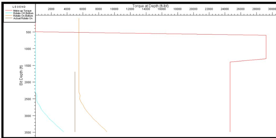
Fig.4.25: 1<sup>st</sup> Build Section Torque Point Chart (Wellplan).
