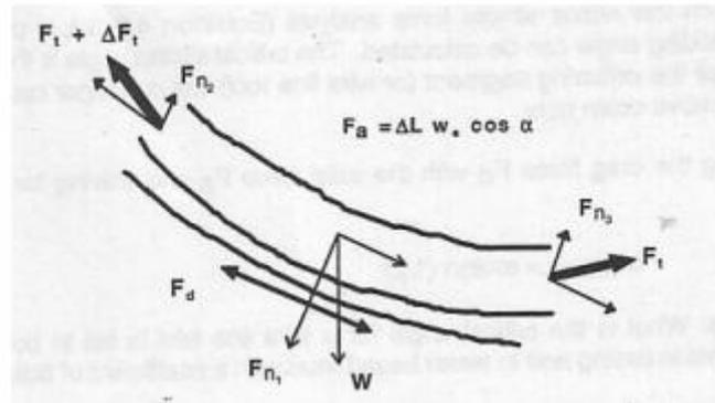
Fig.2.8: Drill string Free Body Diagram (Raksagati, 2008).
