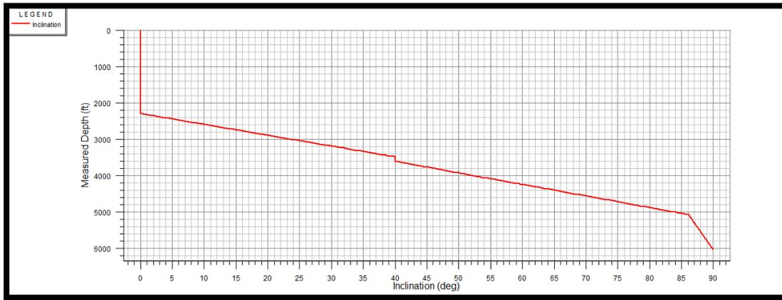
Fig.4.9: 2<sup>nd</sup> Build Section Inclination (Wellplan).
