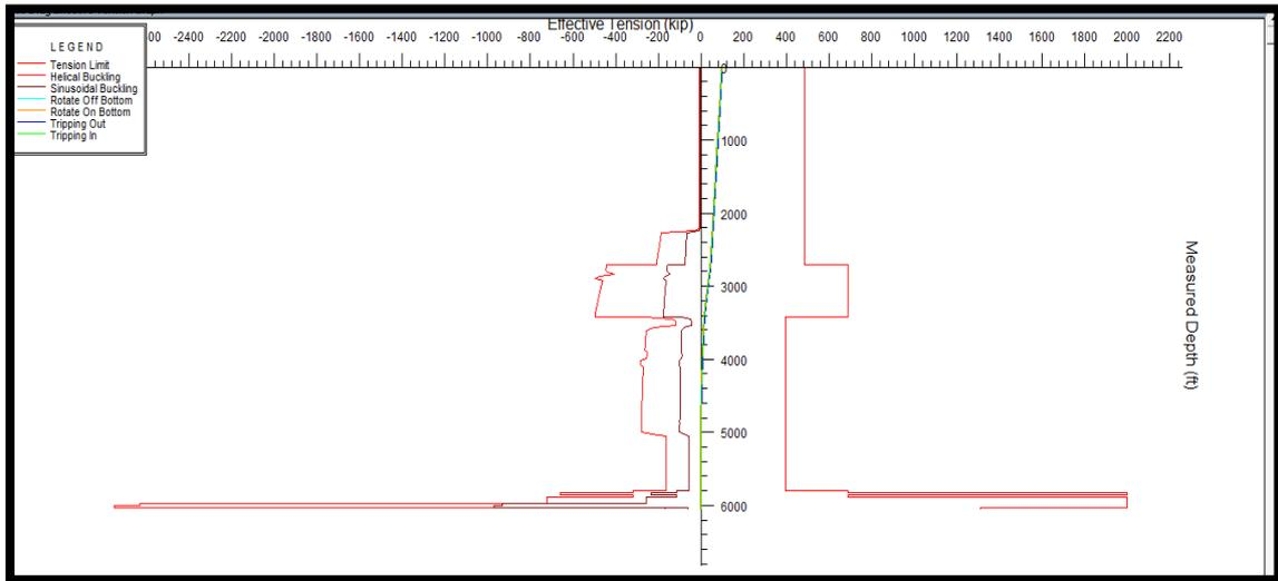
Fig.4.12: 2<sup>nd</sup> Build Section Effective Tension during Tripping in, Tripping out, and Rotating on and off Bottom (Wellplan).
