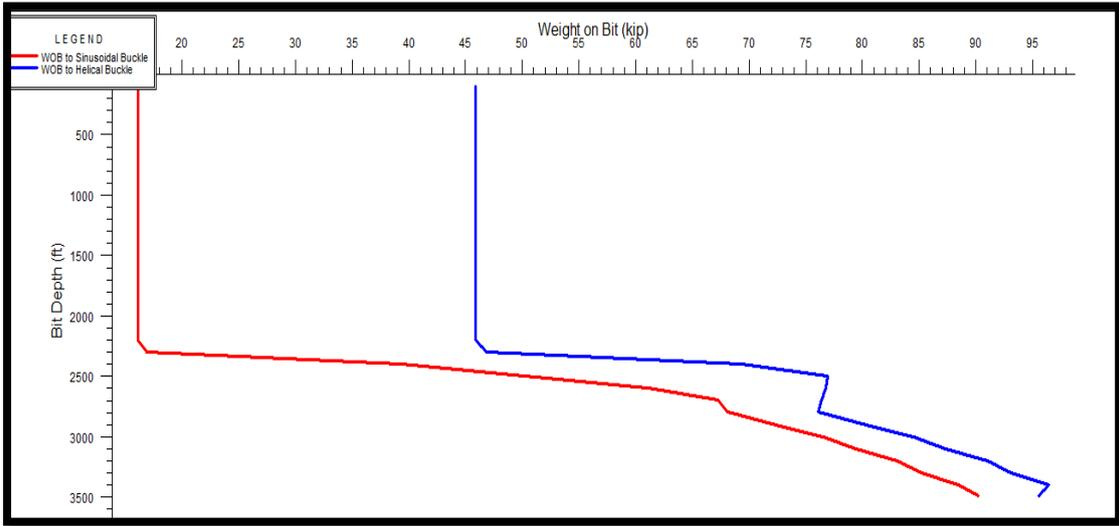
Fig.4.22: 1<sup>st</sup> Build Section Minimum WOB Chart (Wellplan).
