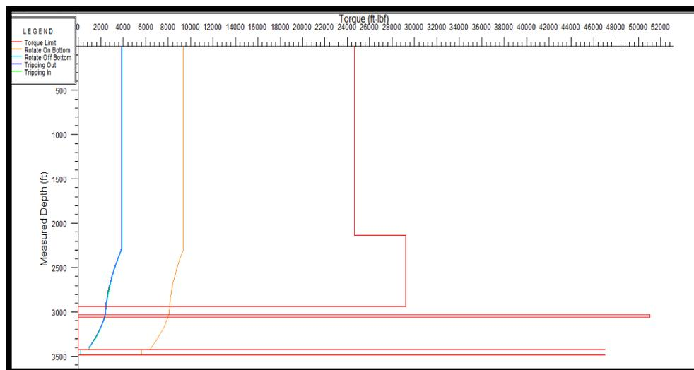
Fig.4.16: 1<sup>st</sup> Build Section Torque Plot (Wellplan).
