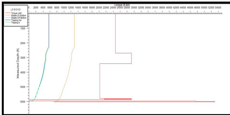
Fig.4.18: 2<sup>nd</sup> Build Section Torque Plot (Wellplan).
