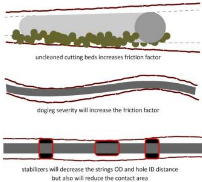
Fig.2.6: Illustration of Factors that Impact the Friction Factor (Raksagati, 2008).
