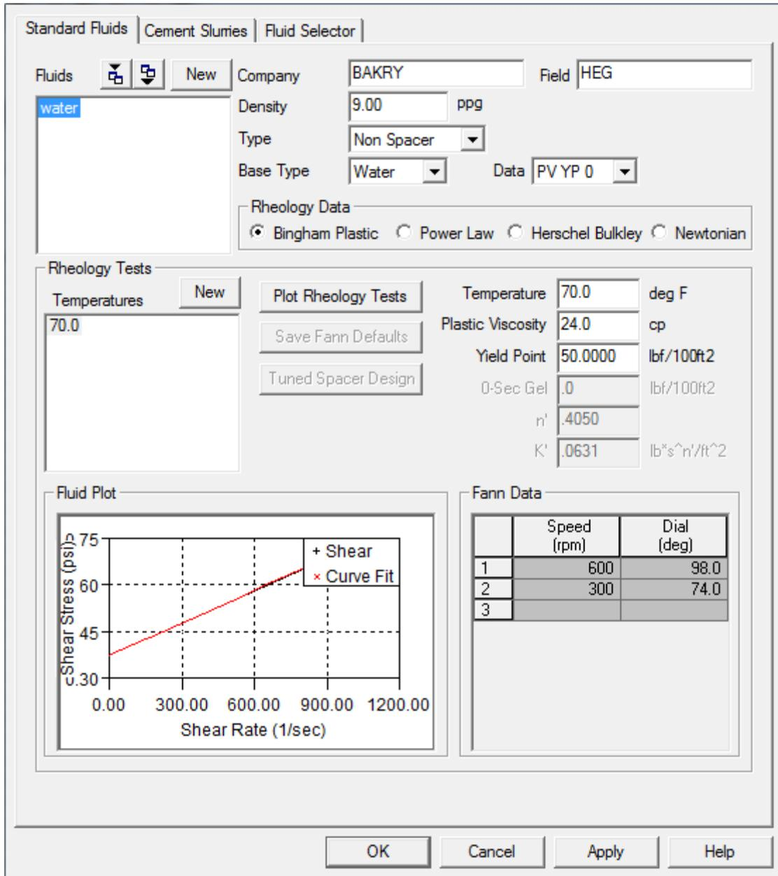
Fig.3.15: 2<sup>nd</sup> Build Section Fluid Editor (Wellplan).
