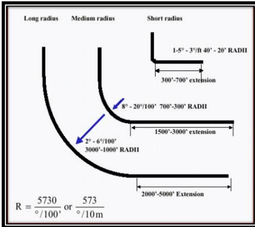
Fig.1.1: Horizontal Well Types (Rabia, Well Engineering and Construction)
