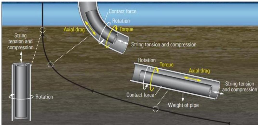
Fig.2.7: Side Forces on the String in Wellbore Orientations (Bennetzen et al. 2010).
