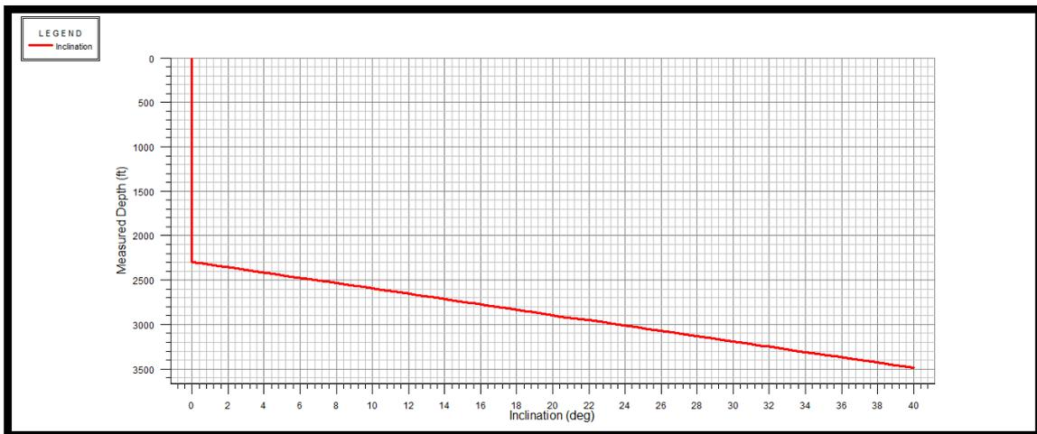
Fig.4.3: 1<sup>st</sup> Build Section Inclination (Wellplan).
