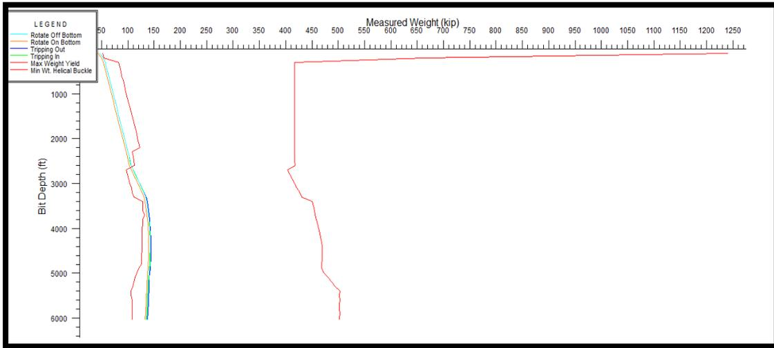
Fig.4.21: 2<sup>nd</sup> Build Section Calculated Weights during Tripping in, Tripping out, Rotating on and off Bottom (Wellplan).
