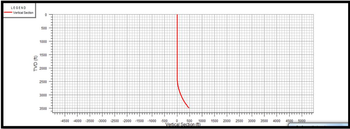
Fig.4.4: Tangent Section Vertical Section (Wellplan).
