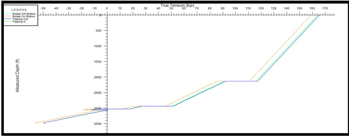
Fig.4.13: 1<sup>st</sup> Build Section True Tension during Tripping in and Tripping out (Wellplan).
