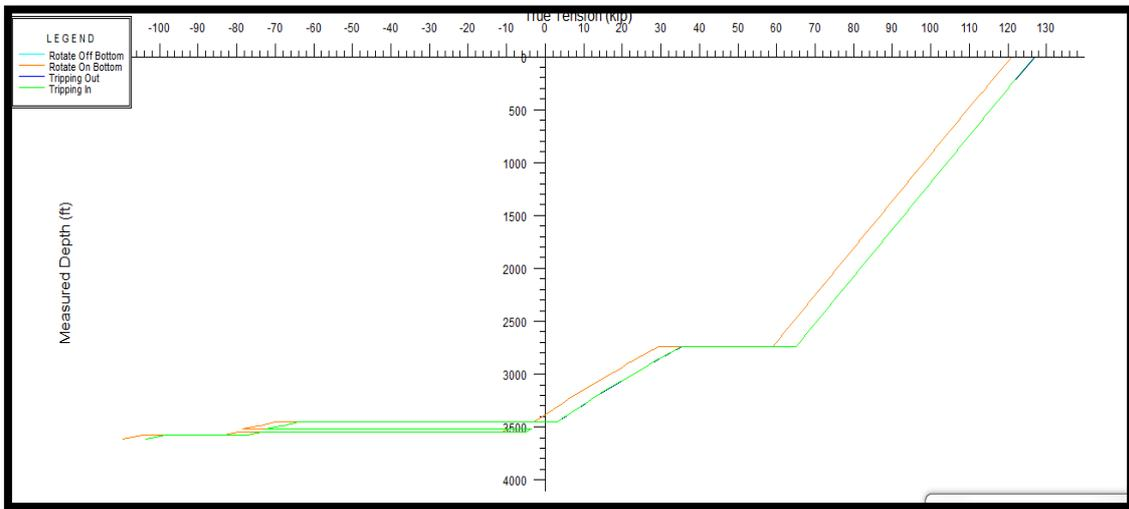
Fig.4.14: Tangent Section True Tension during Tripping in and Tripping out (Wellplan).
