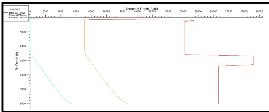
Fig.4.27: 2<sup>nd</sup> Build Section Torque Point Chart (Wellplan).
