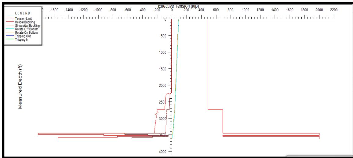
Fig.4.11: Tangent Section Effective Tension during Tripping in, Tripping out, Rotating on and off Bottom (Wellplan).
