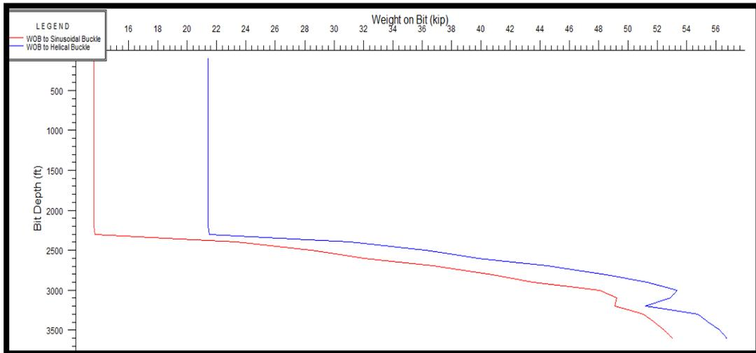
Fig.4.23: Tangent Section Minimum WOB Chart (Wellplan).
