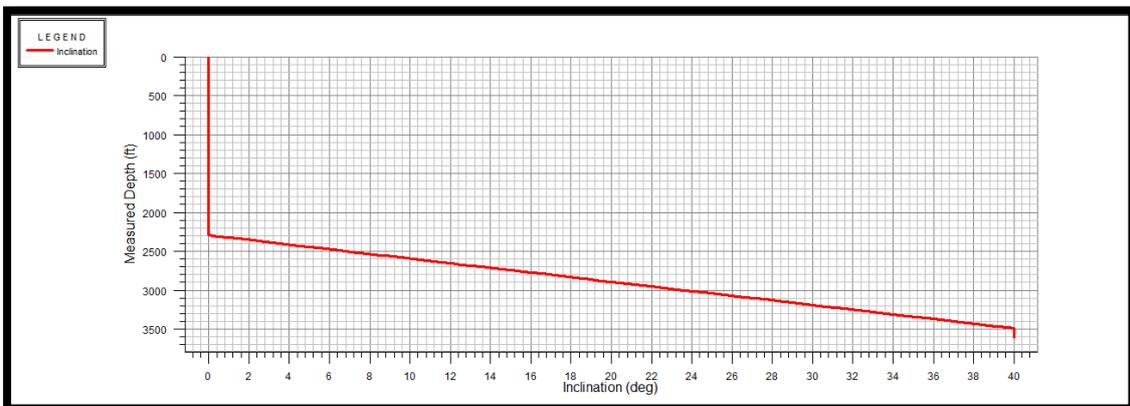
Fig.4.6: Tangent Section Inclination (Wellplan).
