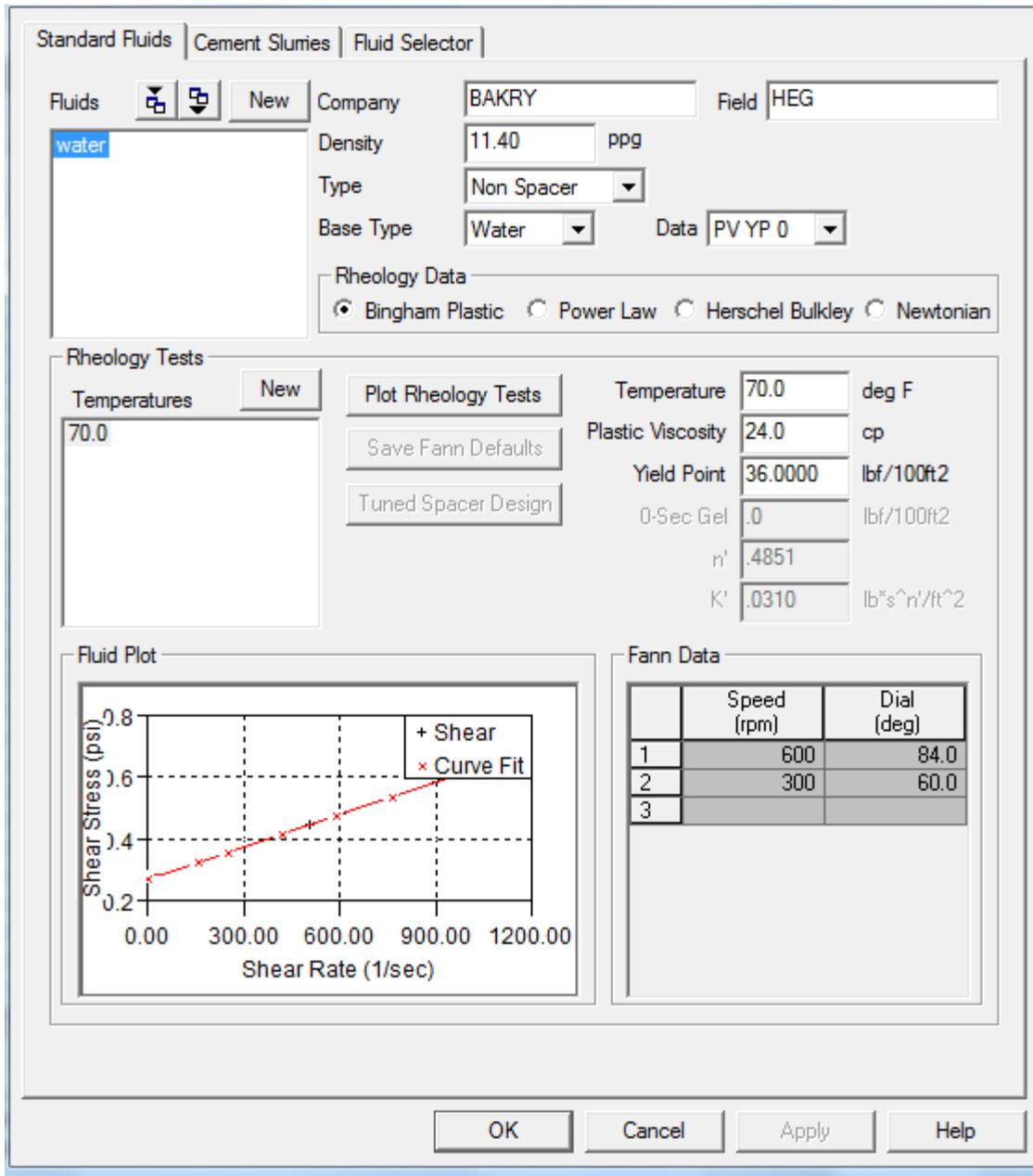
Fig.3.14: Tangent Section Fluid Editor (Wellplan).
