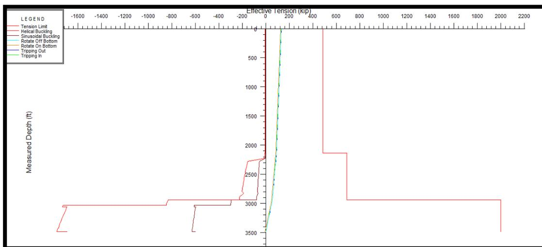
Fig.4.10: 1<sup>st</sup> Build Section Effective Tension during Tripping in, Tripping out, Rotating on and off Bottom (Wellplan).
