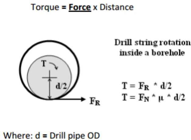
Fig. 2.3: Diagrammatic Representation of Torque Generating Forces (Agbaji, 2009).
