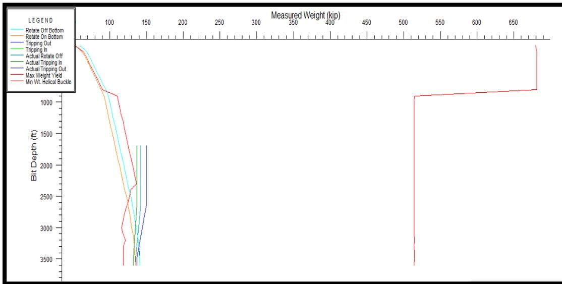
Fig.4.20: Tangent Section Measured and Calculated Weights during Tripping in, Tripping out, and Rotating on Bottom (Wellplan).
