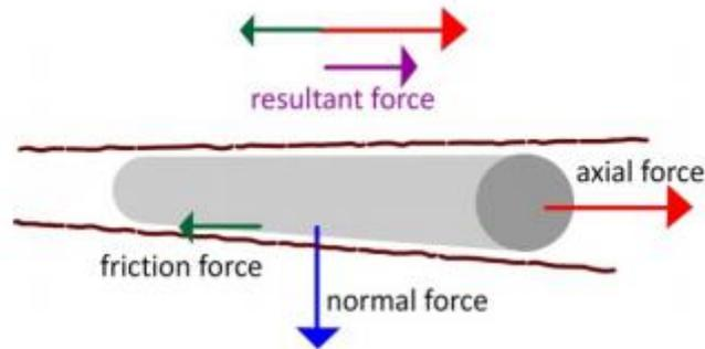
Fig.2.5: Simple Effect of Friction Force (Raksagati, 2008).
