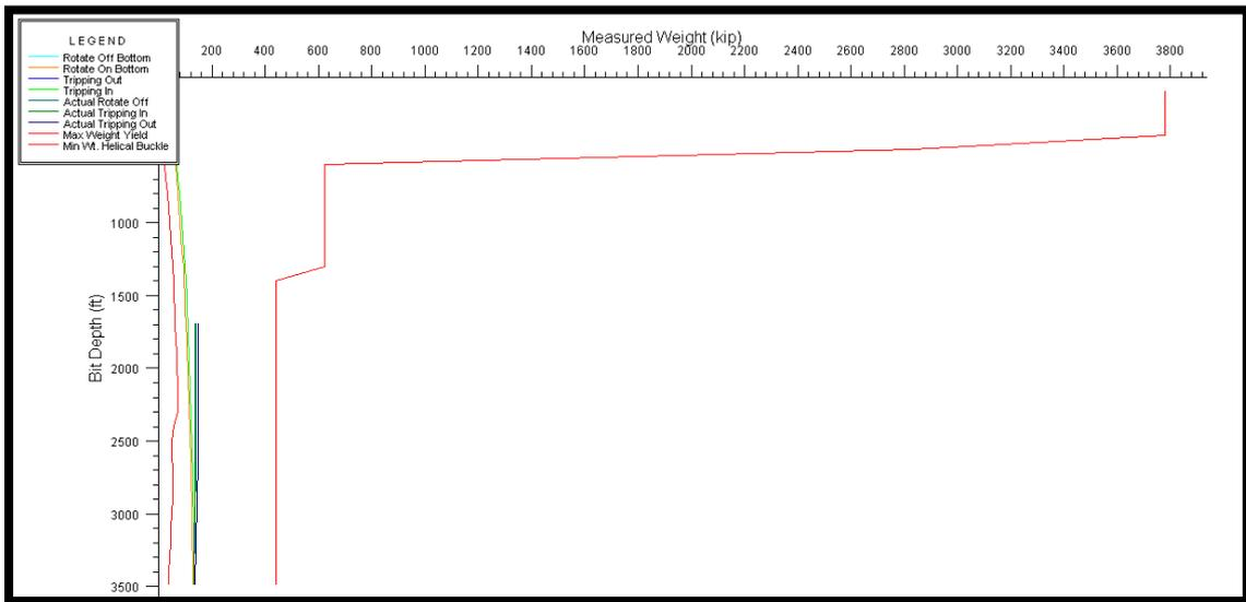
Fig.4.19: 1<sup>st</sup> Build Section Calculated Weights during Tripping in, Tripping out, and Rotate off Bottom (Wellplan).
