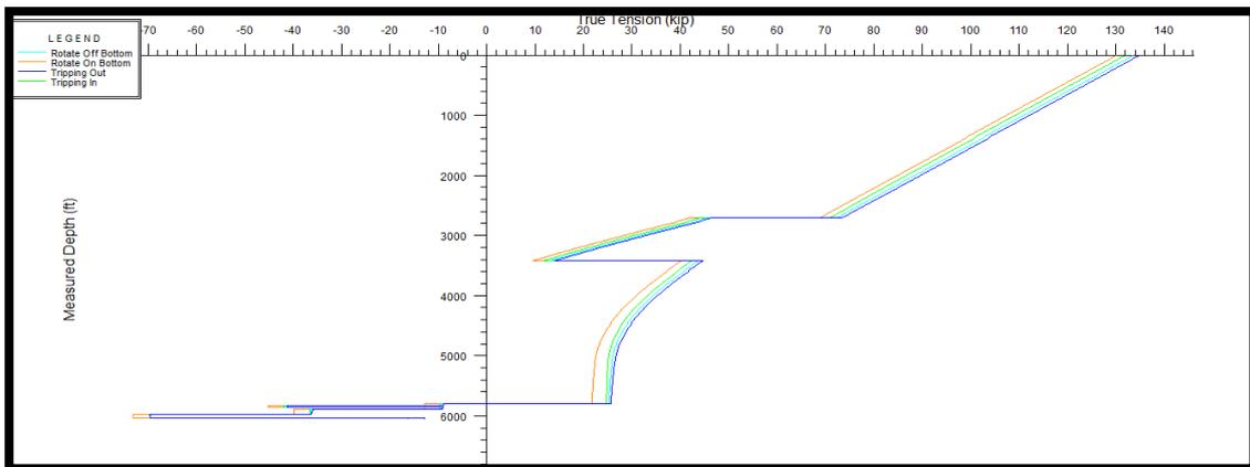
Fig.4.15: 2<sup>nd</sup> Build Section True Tension during Tripping in, Tripping out, rotating on and off Bottom (Wellplan).
