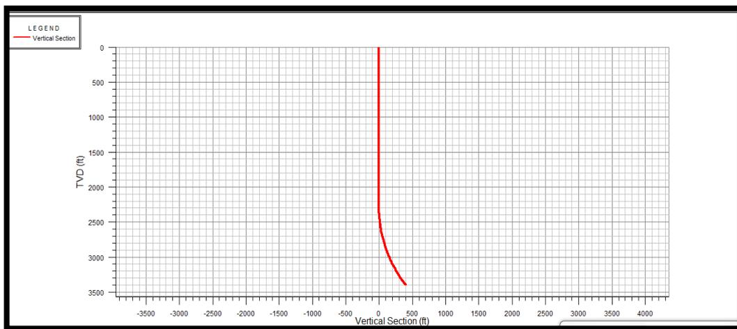
Fig.4.1: 1<sup>st</sup> Build Section Vertical Section (Wellplan).
