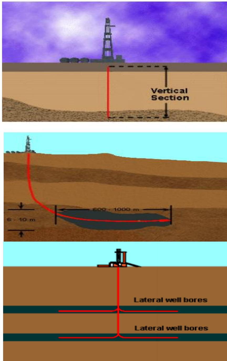
Fig. 1.2: The Difference between Vertical, Horizontal and Multilateral Drilling.
