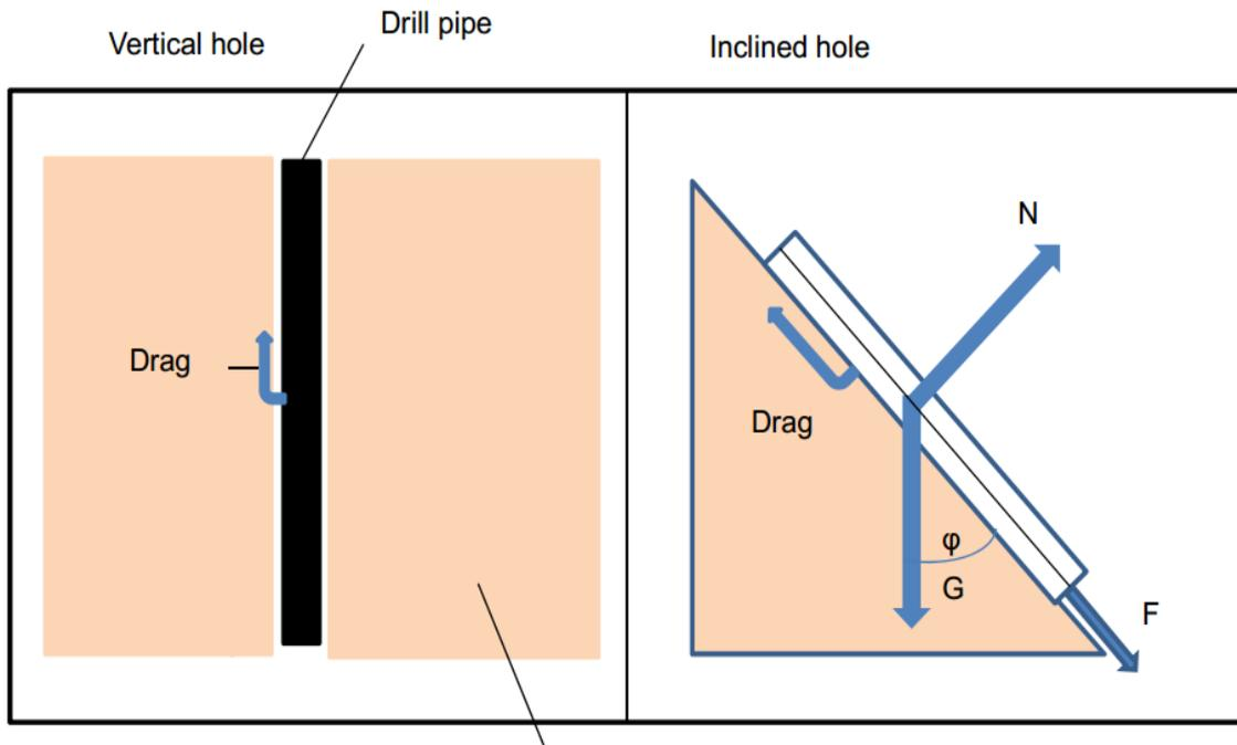
Fig.2.4: Drag in Vertical and Inclined Hole (Borinb, 2012).
