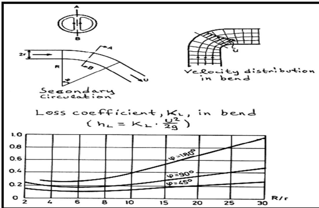
**Fig 2.14: Head loss at smooth pipe bends**
