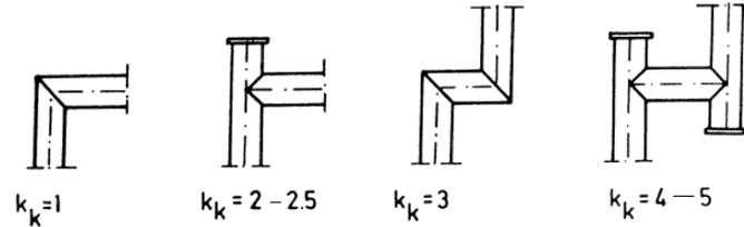
**Fig 2.15: Loss coefficients at right angle bends [7]**
