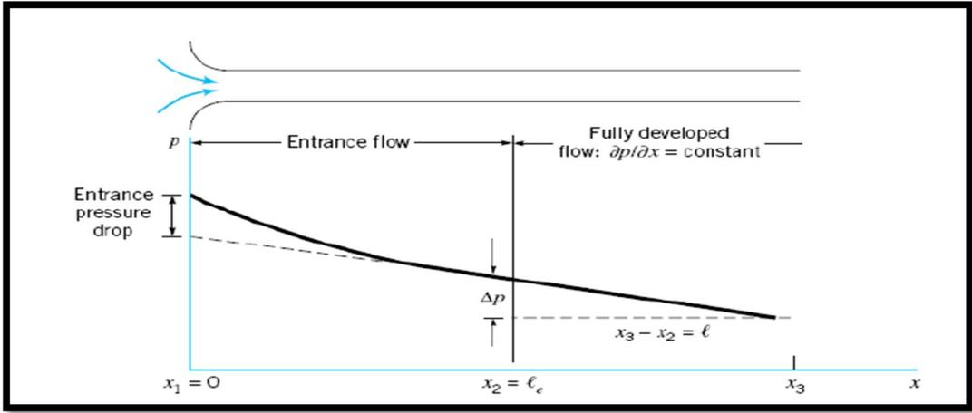
**Fig 2.3: Pressure Distributions in a Horizontal Pipe**
