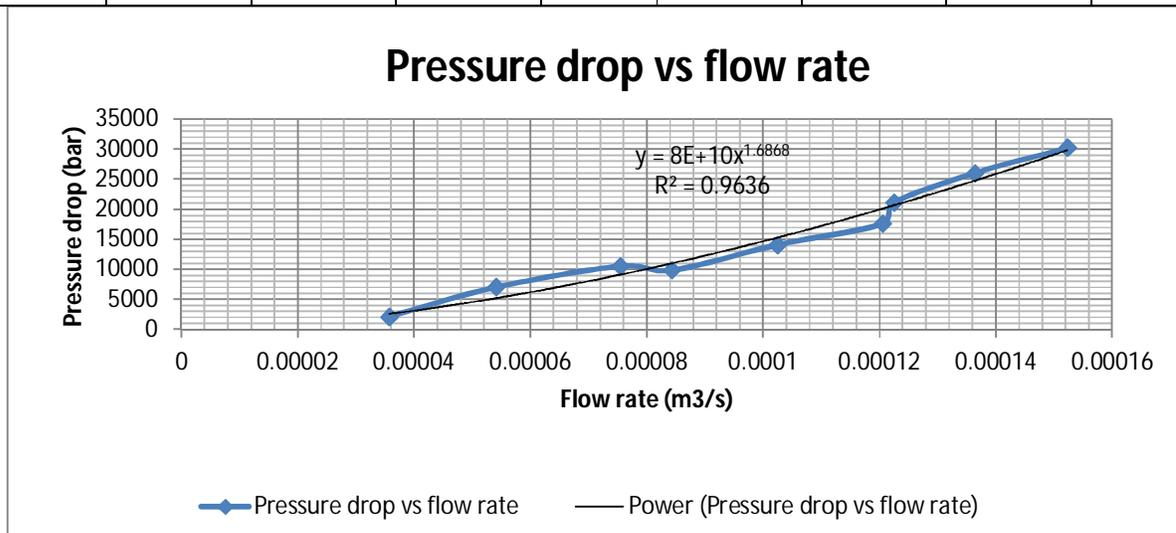
Figure [4.3: pressure drop vs flow rate for elbow and pipe model
