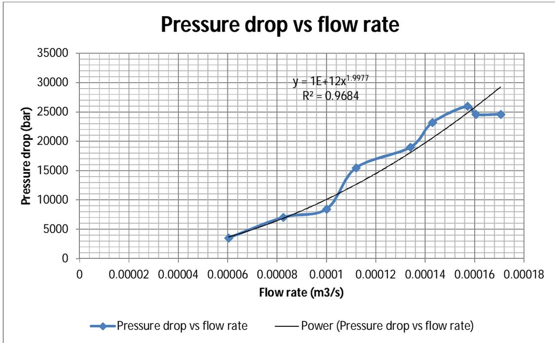
**Figure 4.1: pressure drop vs flow rate for elbow model**
