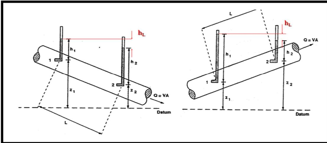
**Fig 2.4: Flow in non horizontal pipe**
